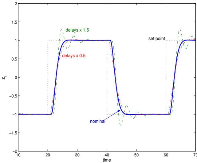
**Figure 1:** Response of the closed loop system to step input: nominal case and the effect of delay uncertainty.
