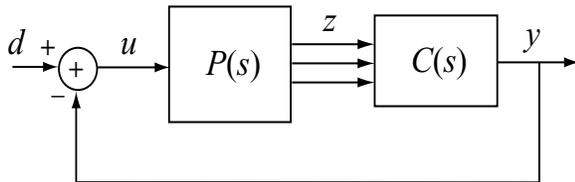
**Figure 2:** The configuration used for loop transfer function comparison of the time delay system and the non-delay proxy system.
