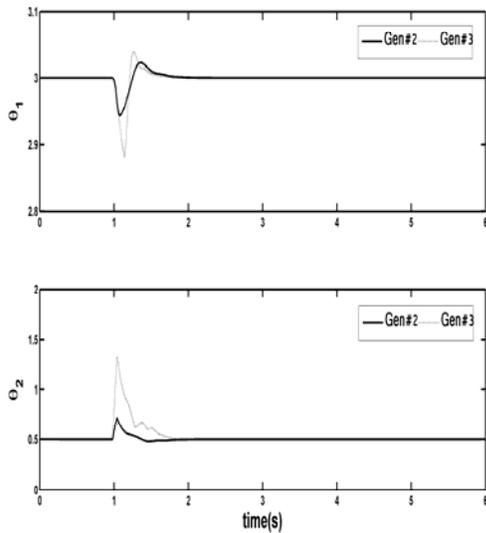
Fig. 4. Estimated parameter for generator 2 and 3 (case 1)
