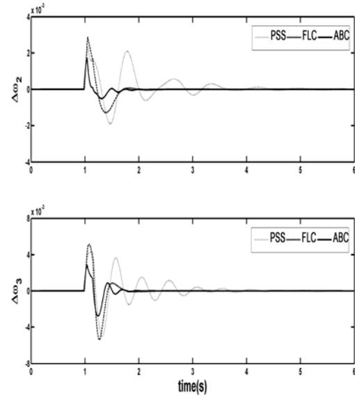
Fig. 3. Response of angular speed for generator 2 and 3(case 1)
