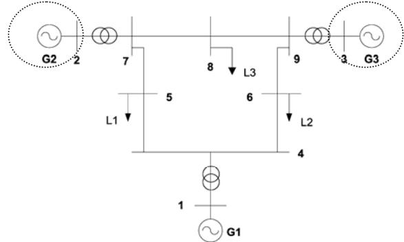
Fig. 1. 3-machine 9-bus power system (--PSS installations)
