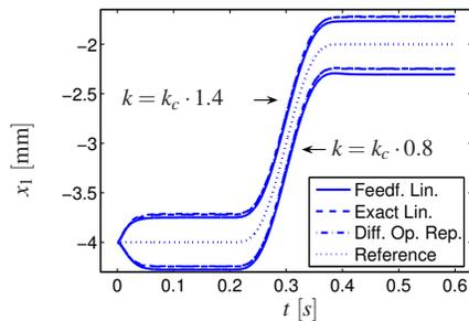
Fig. 2. Resulting trajectory for deviations of  $k$
