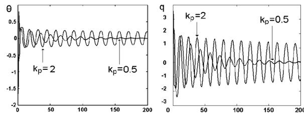
Fig. 2. Closed loop responses of the velocities  $\dot{\theta}$  and  $\dot{q}$ , for  $k_p = 0.5$  and  $k_p = 2$ .
