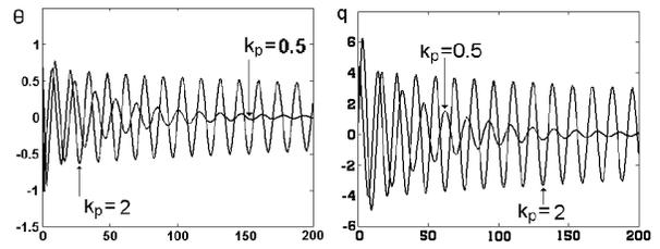
Fig. 1. Closed loop responses of the variables  $\theta$  and  $q$ , for  $k_p = 0.5$  and  $k_p = 2$ .
