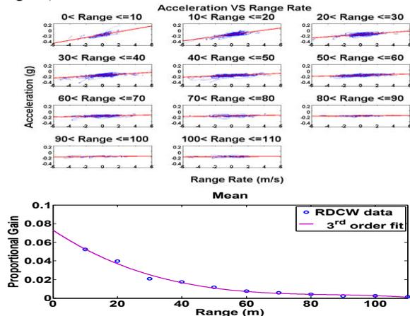
Fig. 1. RDCW data vehicle acceleration VS range rate with respect to different range
