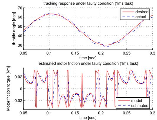
Fig. 6. Estimated friction torque under faulty conditions with a sinusoidal input.
