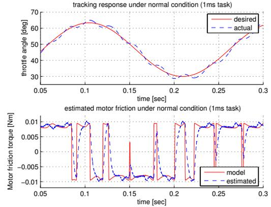
Fig. 4. Estimated friction torque under normal conditions with a sinusoidal input.
