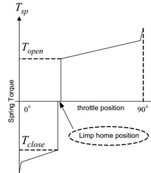
Fig. 3. Nonlinear Spring Torque
