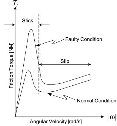
Fig. 2. Friction Torque under a Specific Control Input
