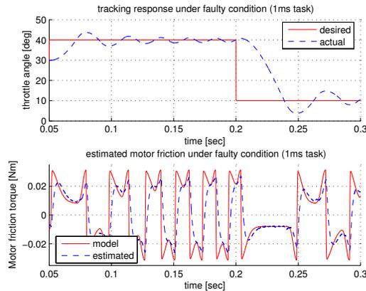
Fig. 7. Estimated friction torque under faulty conditions with a step input.
