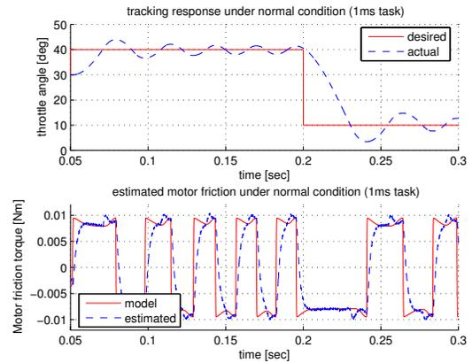
Fig. 5. Estimated friction torque under normal conditions with a step input.
