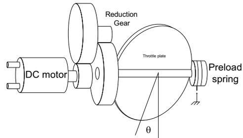
Fig. 1. Electronic Throttle Body Schematic
