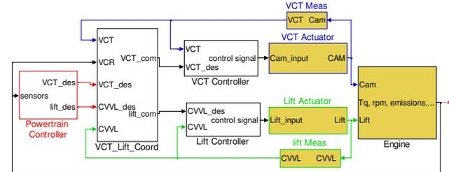
Fig. 6: Block diagram of system showing a new strategy block, *VCT\_lift\_Coord*, inserted into a standard control system.
