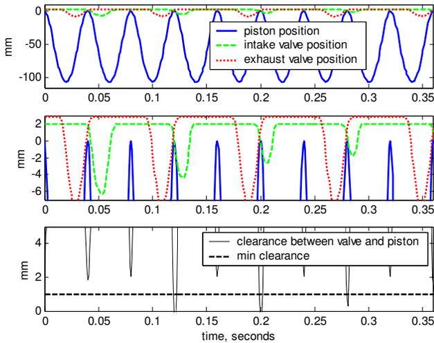
Fig. 4: VCT gets ahead of lift, causing interference.
