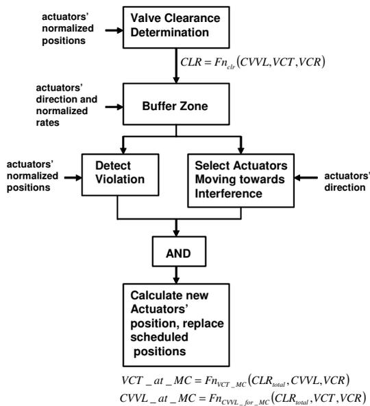
Fig. 8: Flow of control in the  $VCT\_Lift\_coord$  block.
