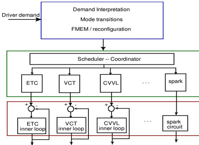
Fig 3: A hierarchical block diagram of a typical engine control system.
