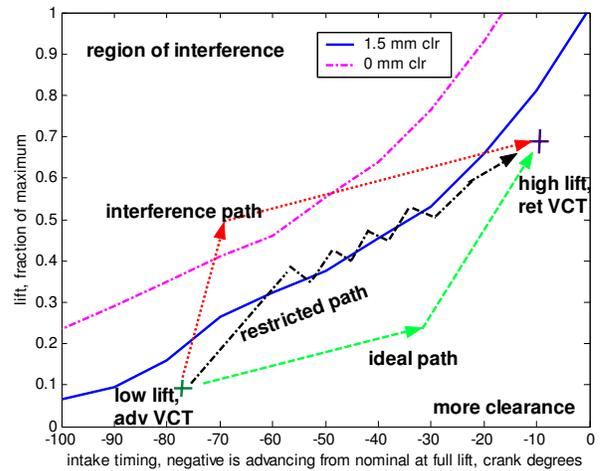
Fig. 9: Possible paths that the two actuators may take when moving from the lower left to the upper right steady state scheduled operating point.
