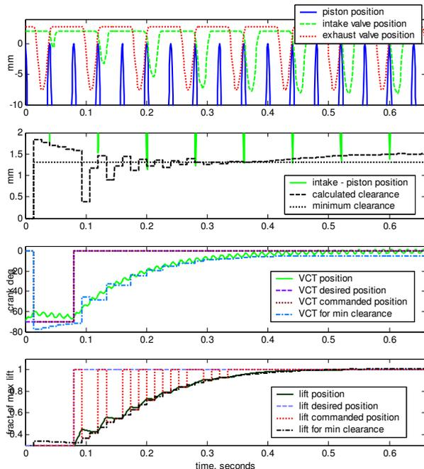
Fig. 10: CVVL lift is too fast and is restricted.
