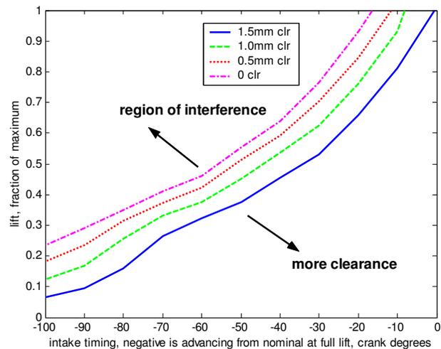
Fig. 7: TDC clearance curves in the VCT and valve lift plane, fixed VCR.
