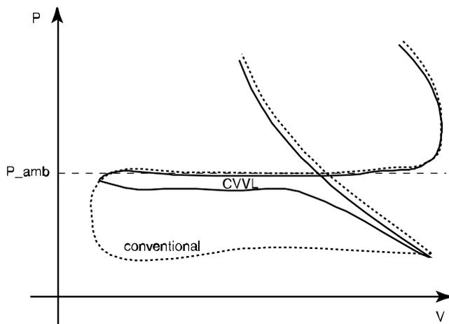
Fig 1: Pumping loop comparison of CVVL and conventional engines.
