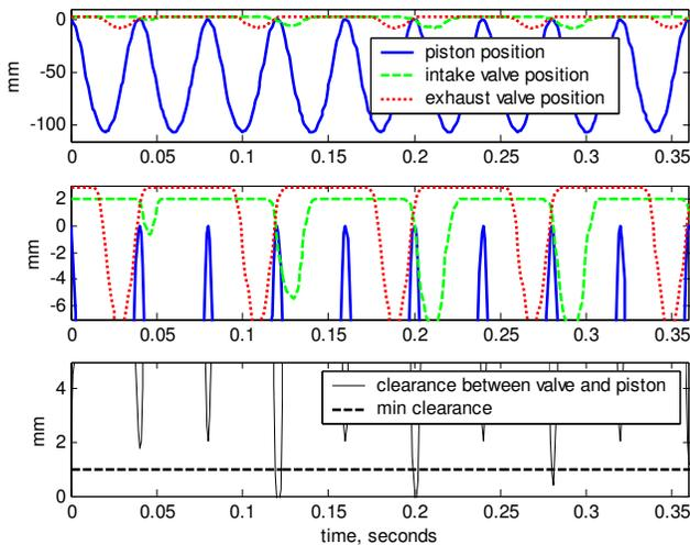
Fig. 5: Lift gets ahead of VCT, causing interference.
