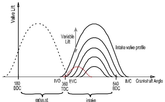
Fig. 2: Intake valve profiles versus crank angle for different values of lift.
