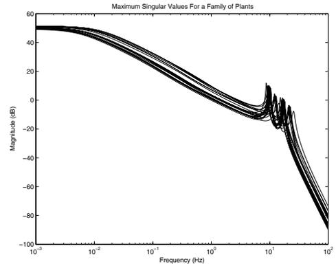
Fig. 3. Singular value plot of plants with varying parameters
