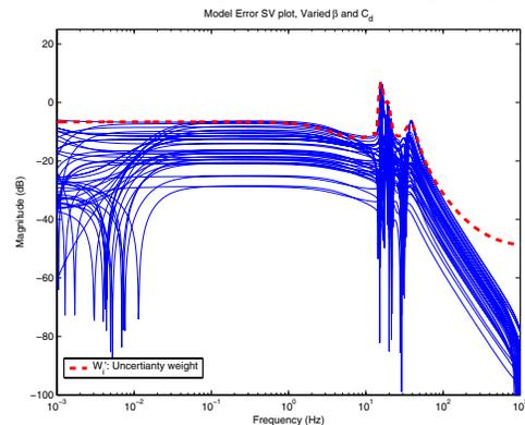
Fig. 12. Family of input multiplicative errors for the Nonlinear force control system
