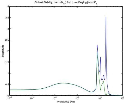
Fig. 8. Robust stability for  $H_\infty$  controlled system, varying parameters attributed to the selection of the performance weight,  $W_p$ . There is an initial jump in the tilt error.
