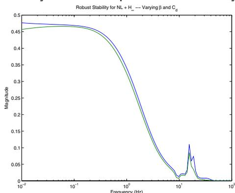
Fig. 14. Robust stability of the NL force -  $H_\infty$  controlled system with varying parameters
