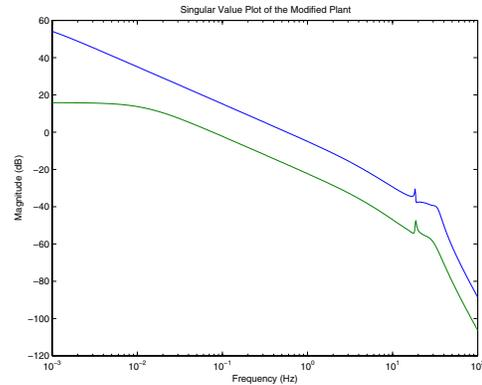
Fig. 11. Nonlinear force control system frequency response
