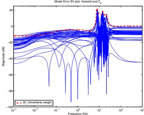
Fig. 4. Singular value plot of plant uncertainty and bounding weight for varied parameters,  $\beta$  and  $C_d$
