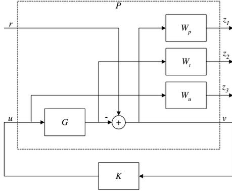
Fig. 6. Plant with Sensitivity Weights
