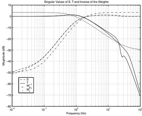
Fig. 7. Sensitivities S and T for the  $H_\infty$  control design
