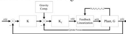
Fig. 10. Nonlinear force control system structure
