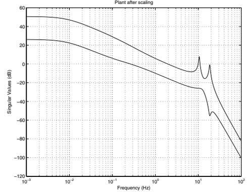
Fig. 2. Singular value plot of the plant after scaling
