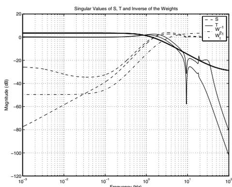
Fig. 13. Nonlinear/ $H_\infty$  force control system sensitivity frequency responses
