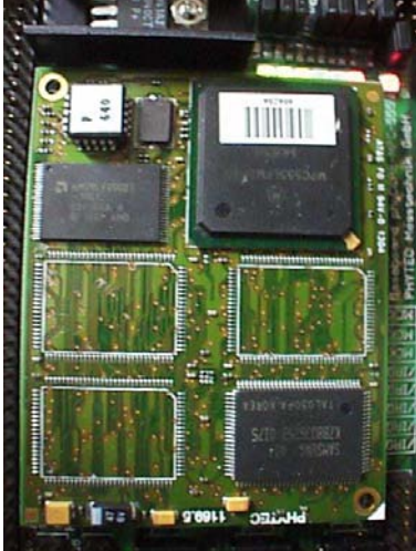
Fig. 3. The Motorola MPC555 processor on the top right. The size of the chip is about 2\text{cm} \times 2\text{cm} .
