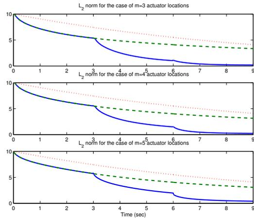
Fig. 1.  $L_2(0, L)$  norm of  $z(t, \xi)$  vs time for different available actuator locations.
