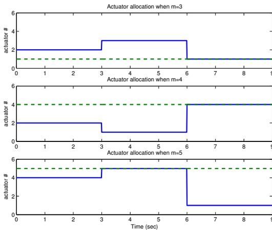
Fig. 3. Actuator allocation (switching) for  $m = 3$ ,  $m = 4$  and  $m = 5$  actuator locations; switching (solid) and fixed (dashed).
