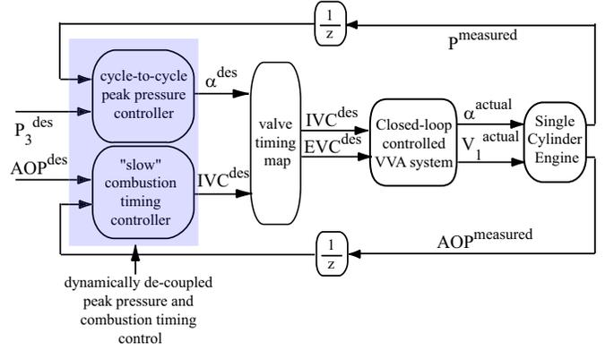
Fig. 3. Control Strategy for Simultaneous Control of Peak Pressure and Combustion Timing
