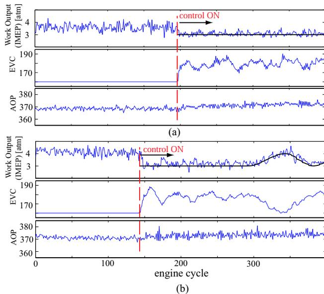
Fig. 8. Direct control of work output, (a) - step response, (b) - step followed by a sine
