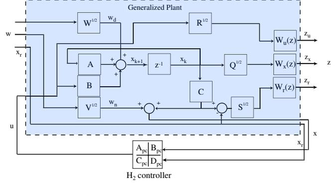
Fig. 4. General control configuration considered for the synthesis of the in-cylinder peak pressure controller
