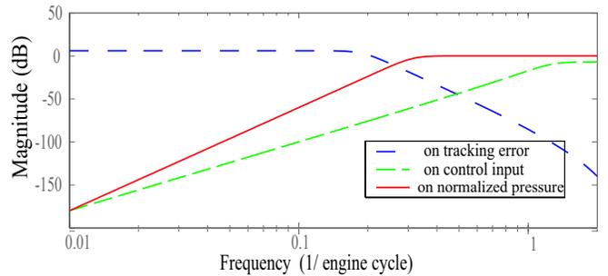
Fig. 5. The frequency dependent weights used for synthesis of the peak pressure control
