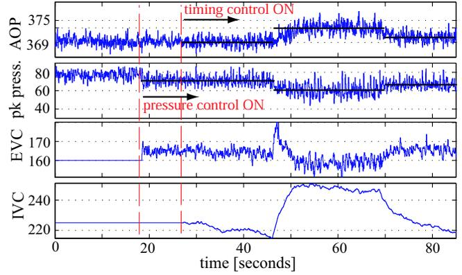
Fig. 7. Simultaneous control of both peak pressure and combustion timing
