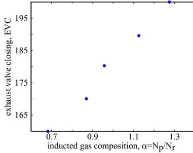
Fig. 1. Relationship between exhaust valve timing and experimental estimate of molar ratio of inducted exhaust products and reactants,  $\alpha \equiv N_p/N_r$
