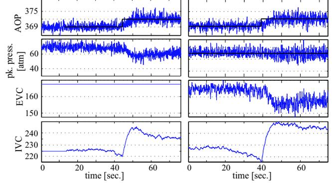
Fig. 6. Comparison of system response with combustion timing control only (a) and both combustion timing and peak pressure control simultaneously (b)
