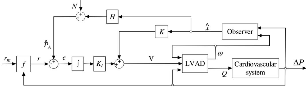
Fig. 4. Physiologic control system structure.
