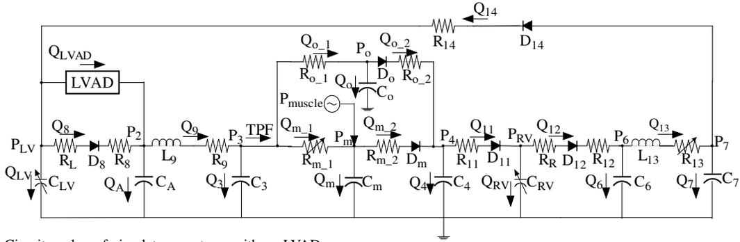
Fig. 1. Circuit analog of circulatory systems with an LVAD.
