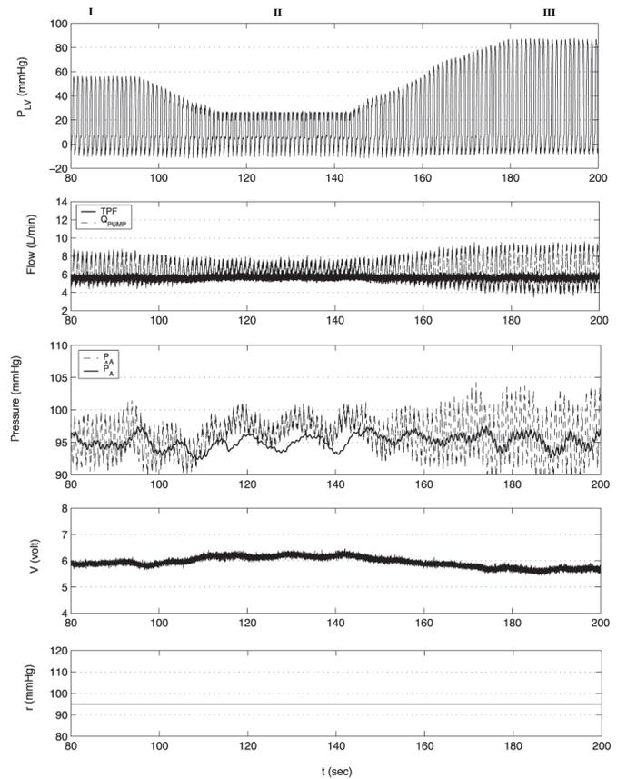
Fig. 6. Experimental results (with MY2 pump):  $P_{LV}$ : left ventricular pressure;  $TPF$  (solid): total peripheral flow;  $Q_{PUMP}$  (dashed): LVAD flow rate;  $P_A$  (dashed): aortic pressure;  $\hat{P}_A$  (solid): estimated aortic pressure;  $V$ : control input voltage;  $r$ : reference value.
