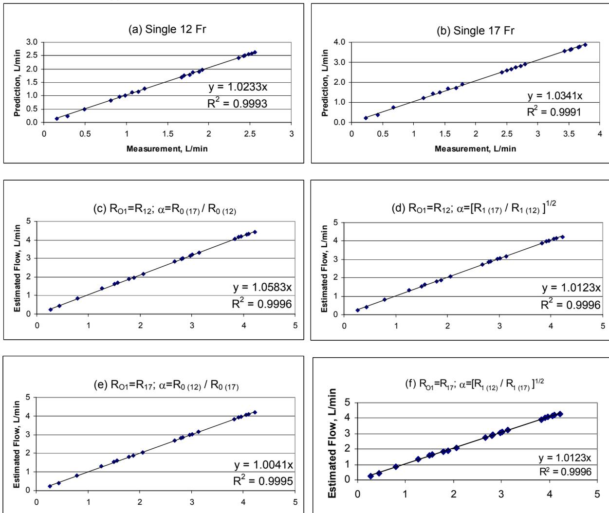
Figure 6. Flow prediction vs. measurement with various outflow cannula configurations
