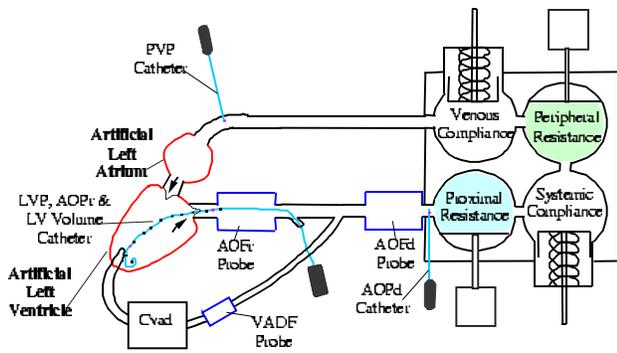
Fig. 1. Schematic of the mock circulatory system with the assist device
