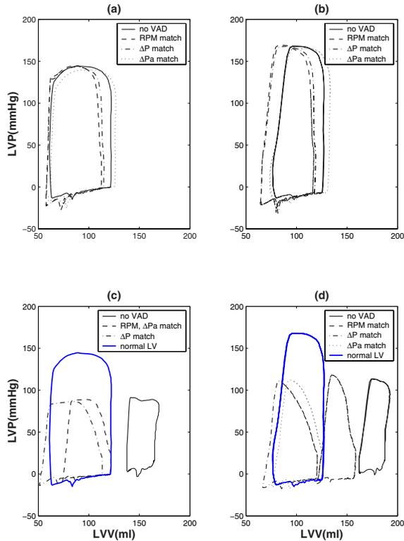
Fig. 3. PV loops with and without VAD assistance using constant rpm,  $\Delta P$  and  $\Delta Pa$  control strategies for the following test conditions: (a) Normal LV during rest; (b) Normal LV during exercise; (c) Failing LV during rest; (d) Failing LV during exercise.
