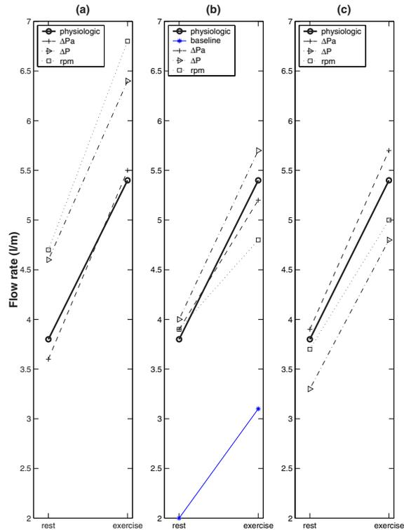
Fig. 2. Comparison of total flow generated with  $\Delta Pa$ ,  $\Delta P$  and constant rpm strategies with and without the VAD: (a) Normal LV; (b) Failing LV; (c) Asystolic LV;
