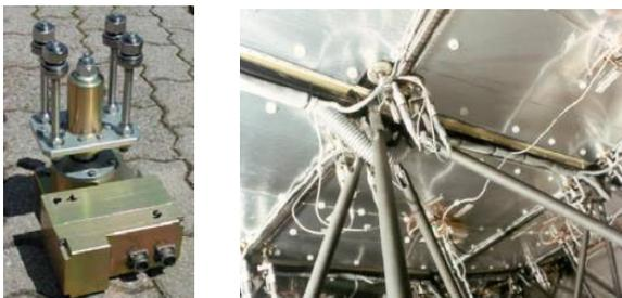
Figure X-2 Surface actuators of the 64m SRT (left)<sup>7</sup> and the 15m IRAM (right) telescopes
