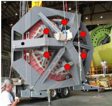
Figure X-5 SOFIA 2.7m mirror cell with attachment points for reaction mass actuators
