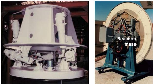
Figure X-6 Subreflector positioner (left) and wobbler (right) of the 30m MRT Spain
