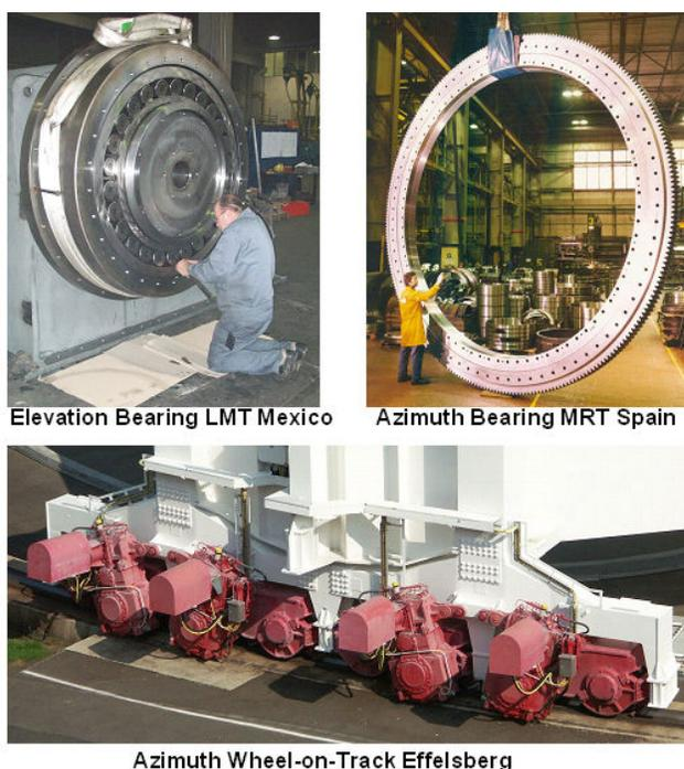
Figure IV-1 Examples of axes mechanisms
