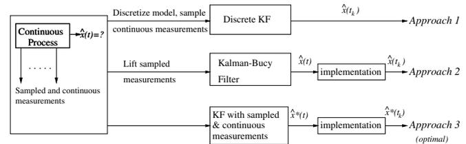
Fig. 1. State estimation problem for continuous process with continuous and sampled measurements.
