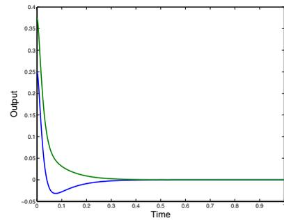
**Fig. 6** Full-order system outputs with reduced-order controller.
