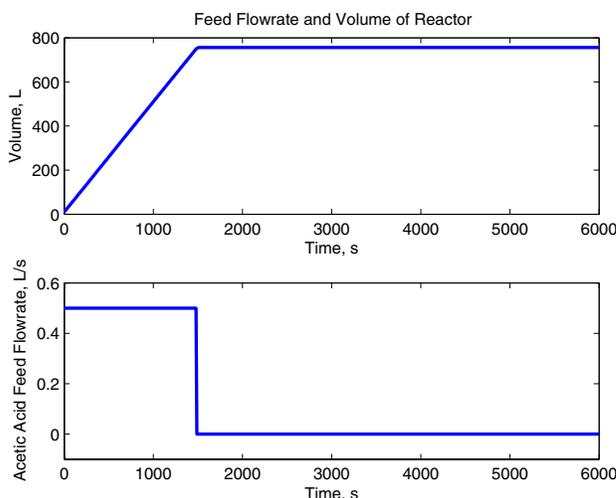
Figure 2 Optimal Feed Rate and Volume Profiles
