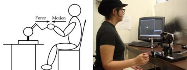
Figure 1: Human interaction with an impedance-based haptic interface
