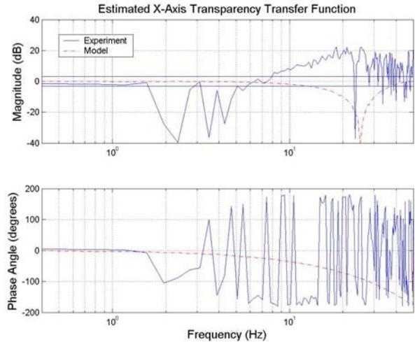
Figure 9: Estimated transparency of X-axis interaction in active test
