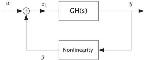
Fig. 7. Block diagram of the AMB model.
