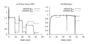
Fig. 5. Power losses (a) and efficiency (b) with optimal (solid) and standard (dashed)  $\psi_{ref}.$
