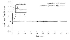
Fig. 13. Rotor flux q component - (underestimated  $R_r$ ).
