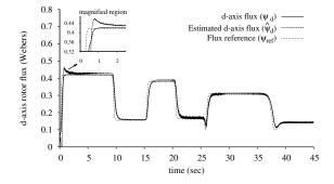
Fig. 12. Rotor flux d component - (underestimated  $R_r$ ).
