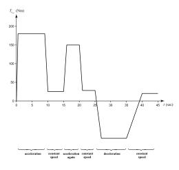
Fig. 4. The Torque reference curve.
