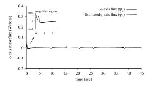
Fig. 9. Rotor flux q component - (known  $R_r$ ).
