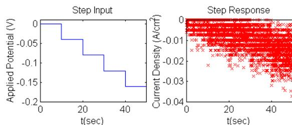
Fig. 2. Incremental step input implemented on the KMC-FD code and the resulting step response. The step response was constructed by plotting the current density computed for every 0.01 second. As shown, the step response is stochastic.
