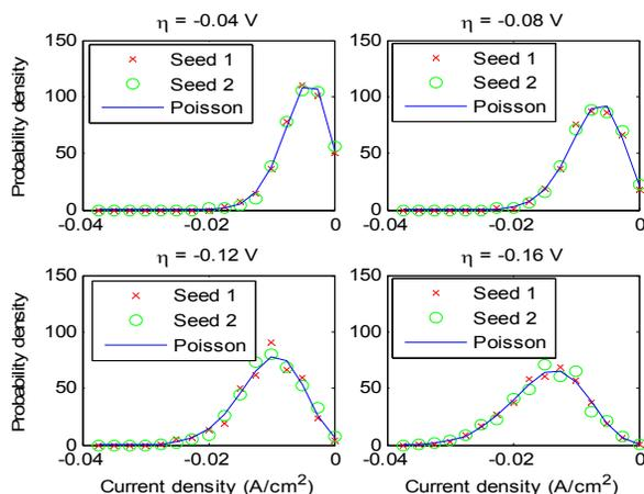
Fig. 3. Current density distributions on four overpotential  $\eta$  values for the low order stochastic model (3)-(4) (solid line) and the coupled KMC-FD simulation.
