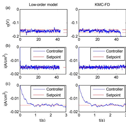
Fig. 5. Closed-loop responses of the overpotential (a) and the filtered current density (b and c) for the feedforward-feedback controller implemented on the low-order stochastic model (3)-(4) and the KMC-FD simulation code.
