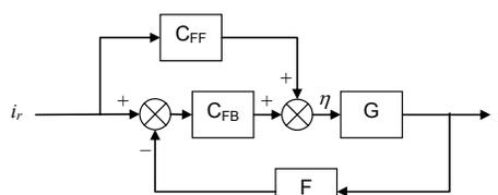
Fig. 4. Block diagram for the closed-loop system:  $G$  is the plant (either the coupled KMC-FD codes or the low-order stochastic model),  $C_{FB}$  and  $C_{FF}$  are the feedback and feedforward controllers,  $F$  is the filter,  $\eta$  is the applied overpotential,  $i$  is the current density, and  $i_r$  is the desired current density.
