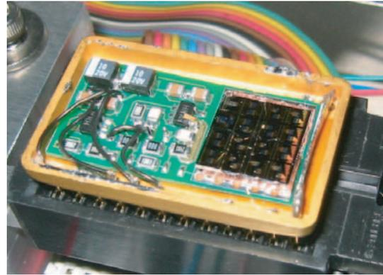
Fig. 4. Picture showing the PCB and the cantilever die during testing.
