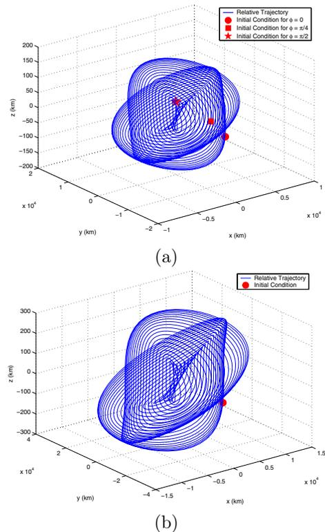
Fig. 2. Trajectory of the follower spacecraft relative to the nominal Halo orbit using: (a)  $Z_{f1}(0) = 0, D = 0.0001, \phi = 0, \phi = \frac{\pi}{4}$ , and  $\phi = \frac{\pi}{2}$  and (b)  $Z_{f1}(0) = 0, D = 0.0002, \phi = 0$
