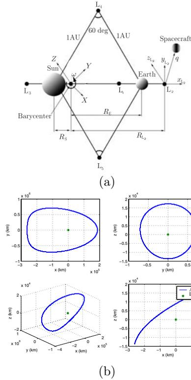
Fig. 1. (a) Sun-Earth system schematic diagram and (b) Halo orbit trajectory of the leader spacecraft relative to the L<sub>2</sub> Lagrange point
