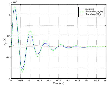
Fig. 8. Impulse disturbance response of Suspension space for nominal plant
