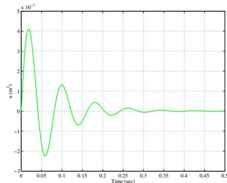
Fig. 9. Control effort in the case of the LQG controller for the nominal plant
