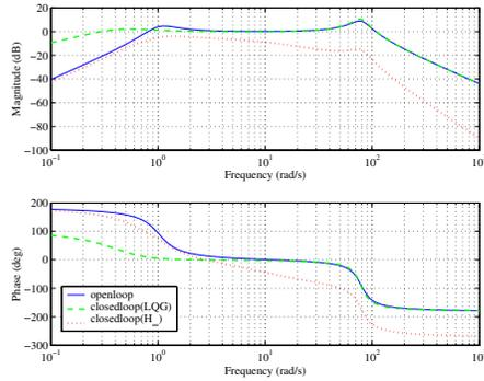
Fig. 6. Bode plots of relative displacement between chassis and wheel  $x_{rel}$
