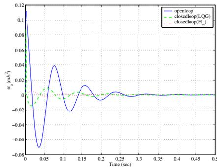
Fig. 7. Impulse disturbance response of chassis acceleration for nominal plant
