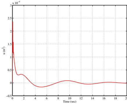
Fig. 10. Control effort in the case of the  $H_\infty$  controller for the nominal plant
