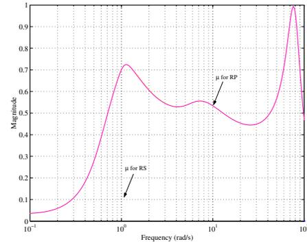
Fig. 12. Structured singular values ( $\mu$ ) in the case of  $H_\infty$  controller
