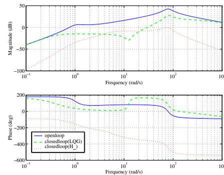
Fig. 5. Bode plots of chassis acceleration  $\ddot{x}_a$
