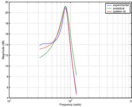
Fig. 2. System identification of wheel parameters
