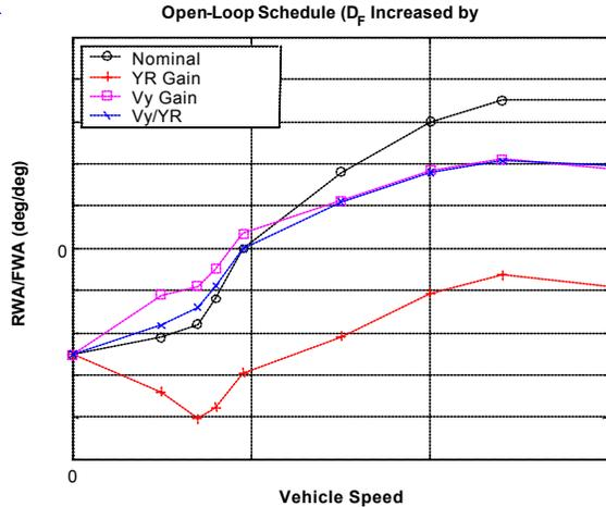
Figure 2. Open-Loop RWS Gear Ratio Schedule for Different Adaptation Strategies.
