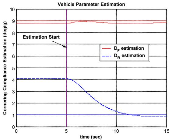
Figure 6. Vehicle Dynamics Parameter Estimation
