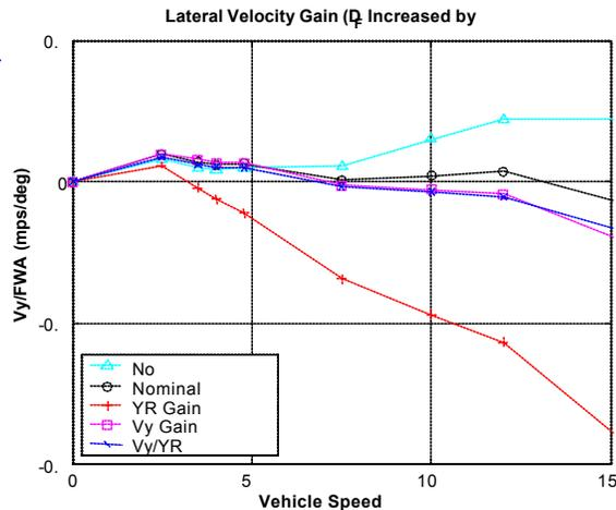
Figure 4. Steady-State Lateral Velocity Gains for Different Adaptation Strategies.
