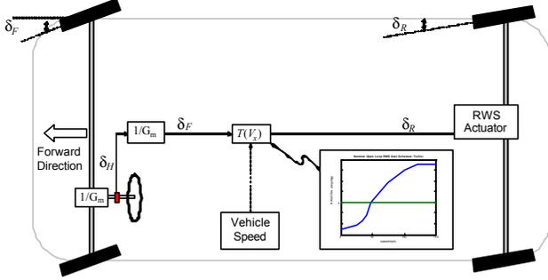
Figure 1. Open-Loop Rear Wheel Steering.
