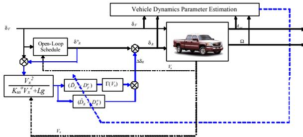
Figure 5. Adaptive Open-Loop RWS Control Structure
