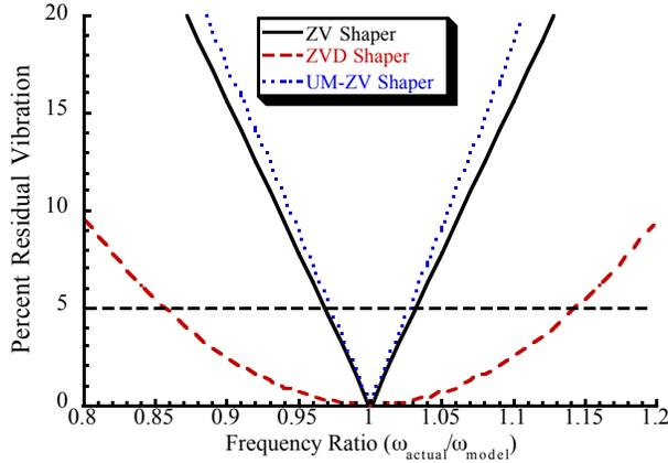
Fig. 2. Sensitivity Curve.
