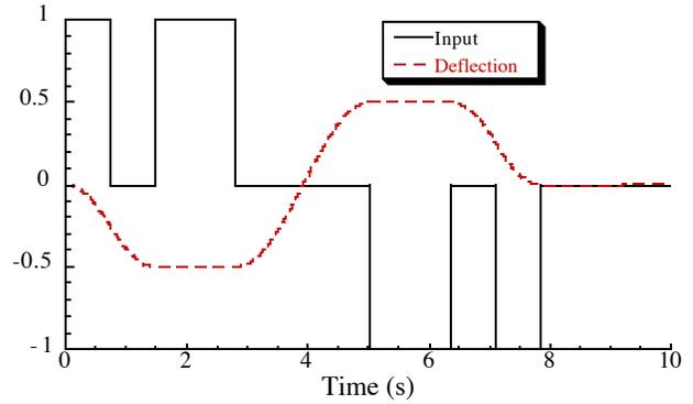
Fig. 7. Five Unit Rest-To-Rest Move Of Benchmark System.
