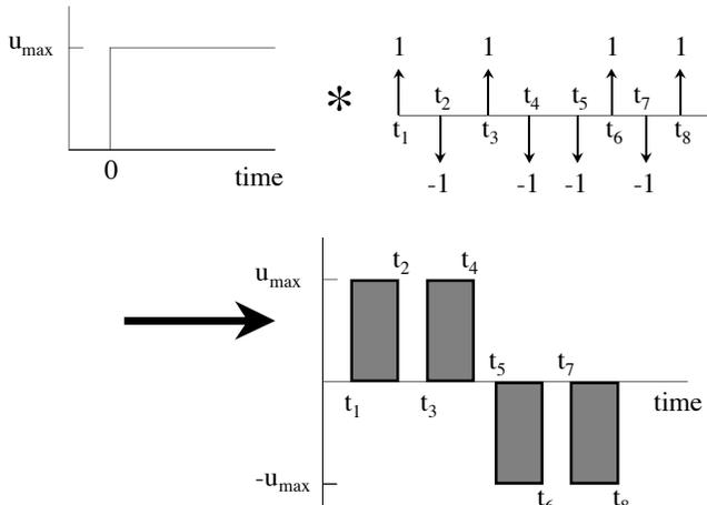
Fig. 6. Creating On-Off Commands using Input Shaping.
