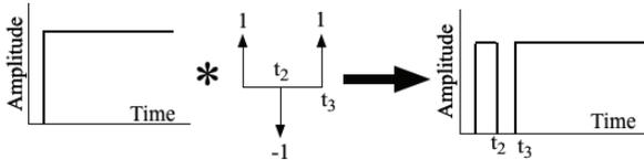
Fig. 3. Unity Magnitude, Zero Vibration Command Shaper.
