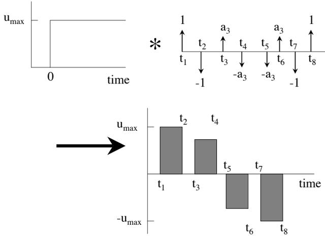
Fig. 9. Analytic Deflection-Limiting Command.
