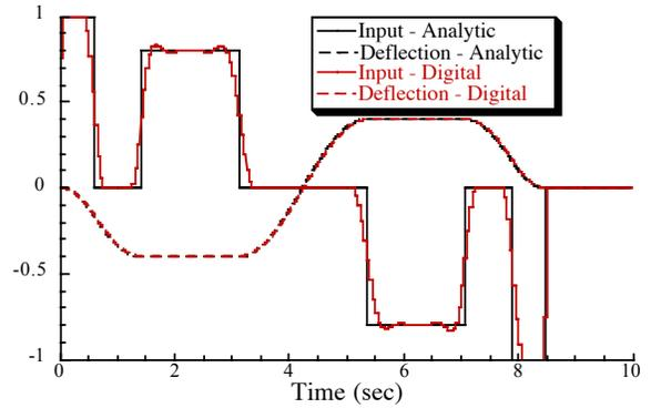
Fig. 10. Move distance = 5 units, deflection limit = 0.4.
