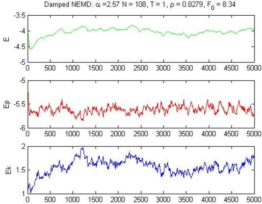
Fig. 2. Energy evolution in damped NEMD simulation (without velocity scaling)
