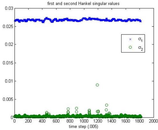
Fig. 4. Two largest Hankel singular values over 1800 time steps of  $r^*(t)$
