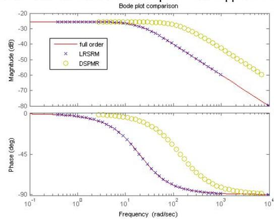
Fig. 6. Bode Plot comparison between full order, first order LRSRM, and first order DSPMR models
