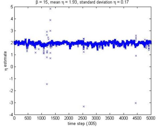
Fig. 3. Estimates of viscosity over 5000 time steps of  $r^*(t)$
