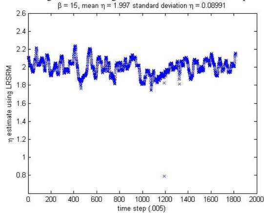
Fig. 5. Viscosity estimates based on the first order LRSRM model, over 1800 time steps of  $r^*(t)$
