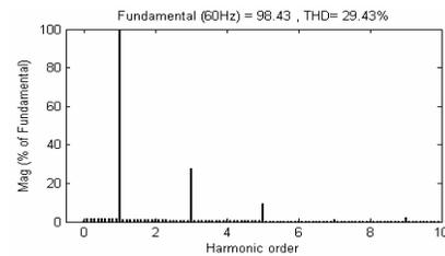
Fig. 8. Spectrum analysis of the source current
