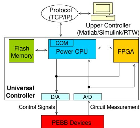
Fig. 2. Topology of a typical universal controller
