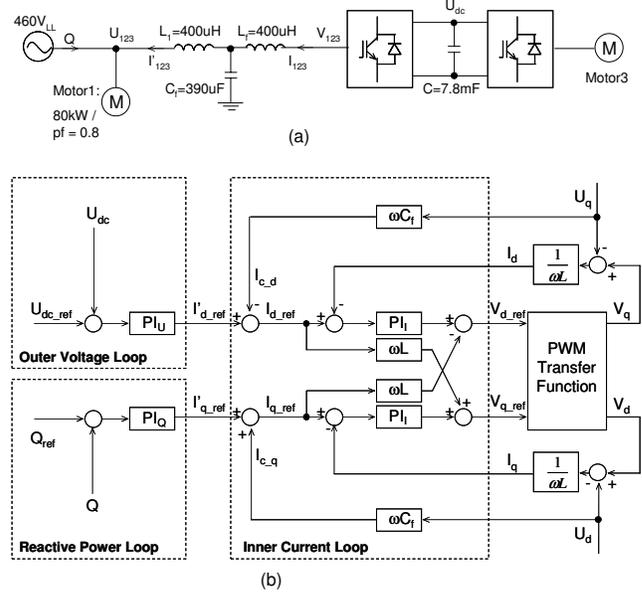
Fig. 10. (a) Simplified circuit; (b) two-loop control block diagram for STATCOM (front end rectifier of the motor drive)
