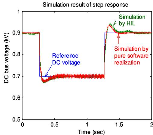
Fig. 11 Comparison of complete software and RT-HIL simulation results
