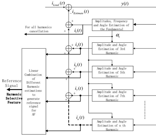
Fig. 5. Control Structure of the Proposed AF
