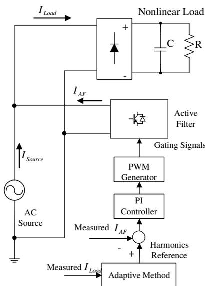
Fig. 6. Simplified Simulation Implementation Block Diagram
