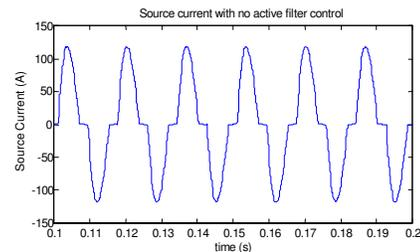
Fig. 7. Source current waveform without active filter control
