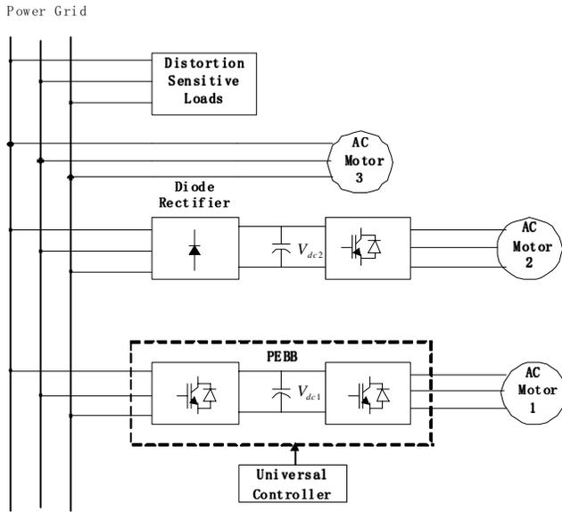
Fig. 3. Functional reconfiguration of PEBB/UC
