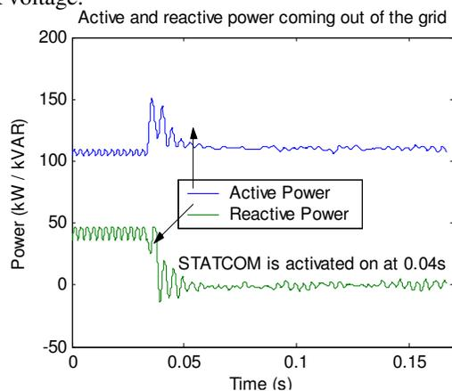
Fig. 12 Illustration of the compensation of reactive power
