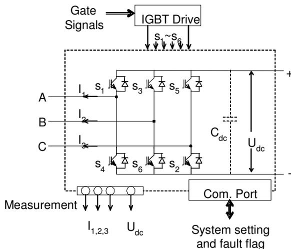
Fig. 1. Pictorial of an IGBT-based PEBB
