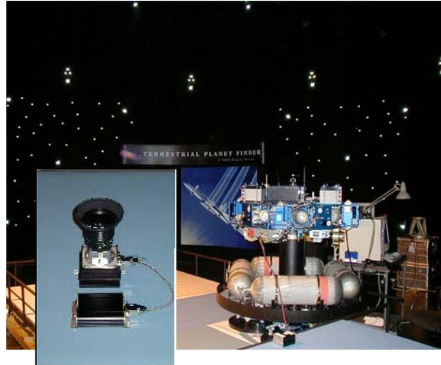
Fig. 1. Photograph of the FCT robot in the Formation Flying Technology Laboratory at JPL. The top attitude stage is supported by a spherical air bearing. Linear air bearings support the entire robot on a precision ground flat floor. Inset shows celestial sensor optics and preamps which are mounted in the center of the attitude stage.
