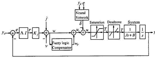
Fig. 3. NN saturation and FL deadzone compensator of systems.
