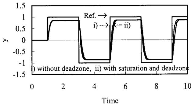
Fig. 7. Experimental response with saturation and deadzone nonlinearity.
