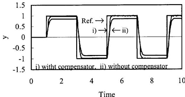
Fig. 8. Experimental response with NN saturation and FL deadzone compensator.
