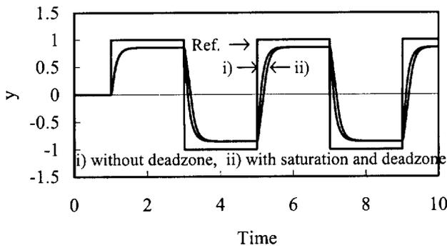
Fig. 5. System response with saturation and deadzone nonlinearity.
