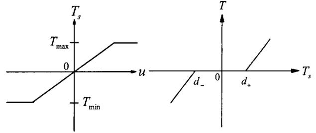
Fig. 1. (a) Saturation and (b) deadzone nonlinearity.
