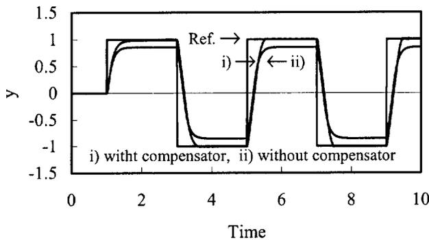
Fig. 6. System response with an NN saturation and FL deadzone compensator.
