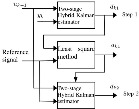
Fig. 7. Structure of the general twosteps hybrid Kalman estimator.
