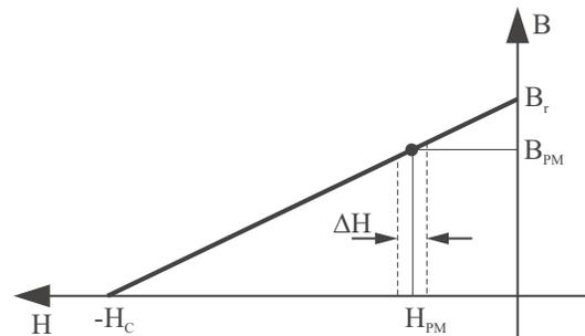
Fig. 3. Permanent-magnet demagnetization curve.
