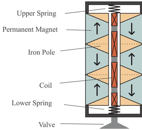
Fig. 2. Cross-section view of the perpendicular linear actuator.
