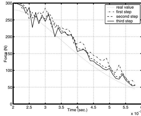
Fig. 11. Disturbance estimation. One-step algorithm (without LSM). Two-step and three-step algorithm (with LSM).
