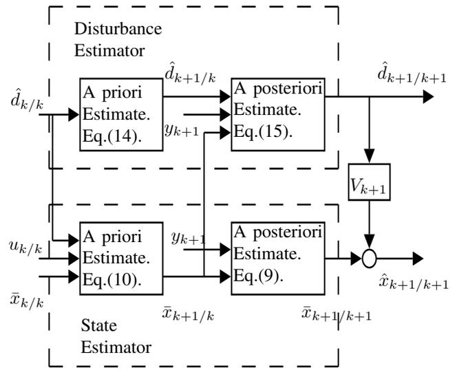
Fig. 6. Structure of the hybrid Kalman estimator.
