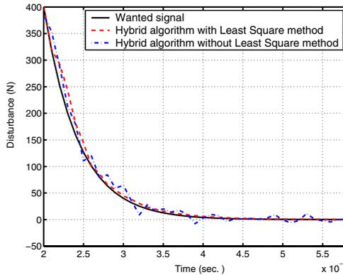
Fig. 10. Disturbance estimation. Dot line: One-step algorithm (without LSM). Dashed line: two-step algorithm (with LSM).
