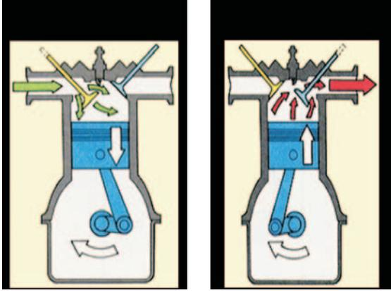
Fig. 1. On the left: Intake valve. On the right: Exhaust valve.
