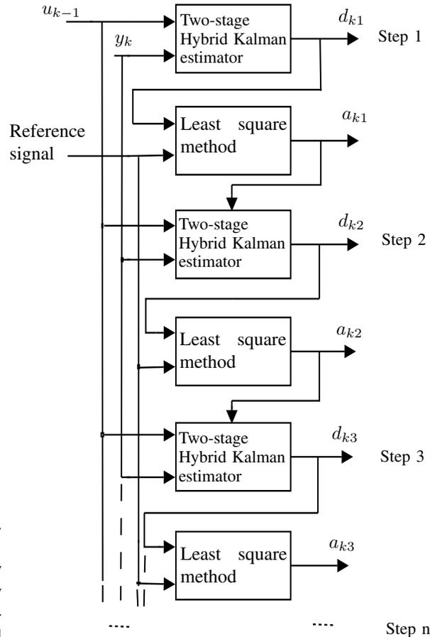
Fig. 8. Structure of the general multistep hybrid Kalman estimator.
