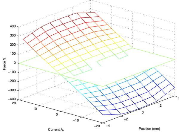
Fig. 4. Force vs. current and position, calculated using FEM.
