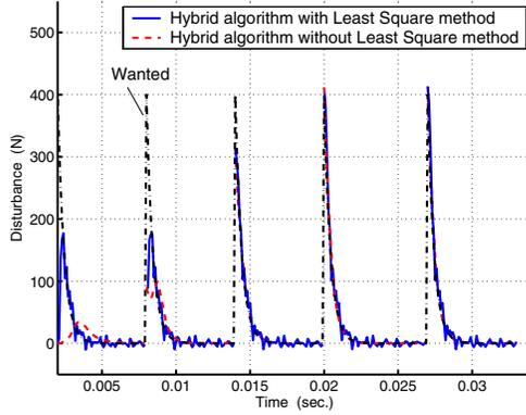
Fig. 9. Approximation of pressure disturbance. Hybrid two stage Kalman algorithm (one-step algorithm) (Solid line). Hybrid two stage Kalman algorithm (two-step algorithm) (Dashed line).
