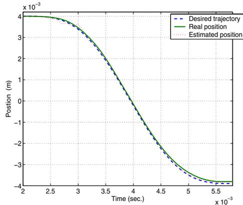
Fig. 12. Dashed line: desired position. Dot line: estimated position. Solid line: controlled position.
