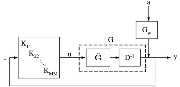
Fig. 2. Closed loop system with separation of interactor matrix
