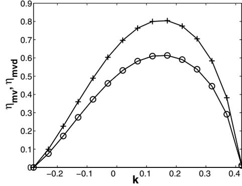
Fig. 3. Comparison of  $\eta_{mv}$  (o) and  $\eta_{mvd}$  (+) for Example 2. The controller structure limits the achievable output performance.
