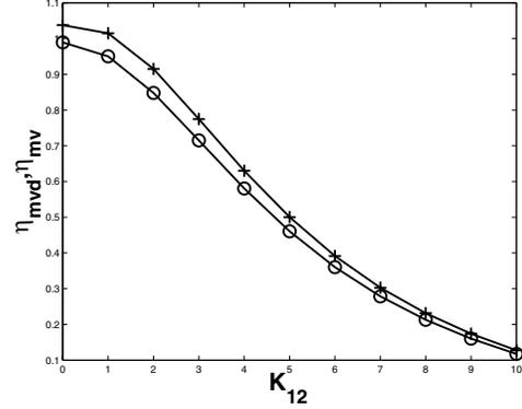
Fig. 4. Comparison of  $\eta_{mv}$  (o) and  $\eta_{mvd}$  (+) for Example 3. The controller structure poses no serious limitations.
