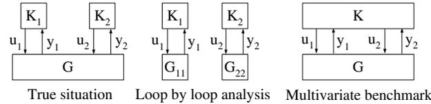
Fig. 1. Insufficiency of available Minimum Variance based benchmarks for performance assessment of systems under decentralized control
