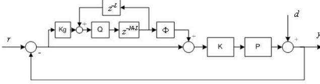
Fig. 1. Plug-in Repetitive Control Scheme
