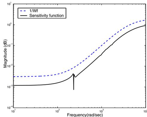
Fig. 10. Magnitude of Sensitivity and Performance Weighting Functions
