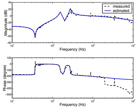
Fig. 7. Measured vs Estimated Model Frequency Response
