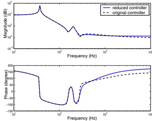
Fig. 9. Frequency Response of Robust Controller
