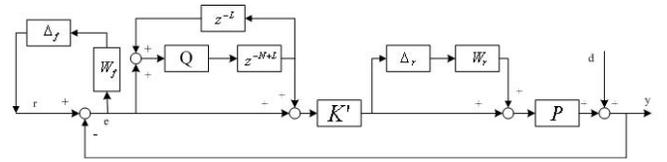
Fig. 6.  $Q$  design in TSRRC
