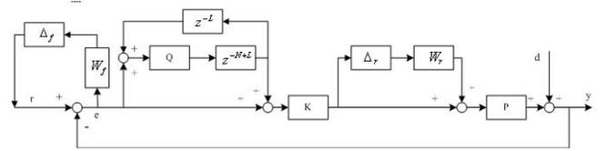
Fig. 2. Block Diagram of Robust Repetitive Control System
