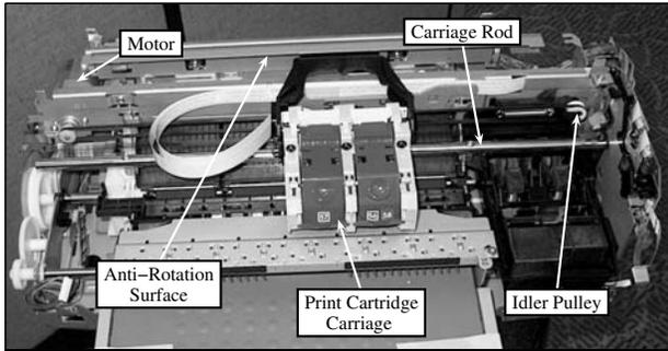
Fig. 2. Pen Carriage Drive on the HP DeskJet 5150
