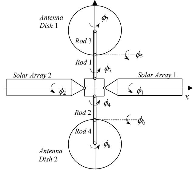
Fig. 1: Top view of a satellite system kinematic model
