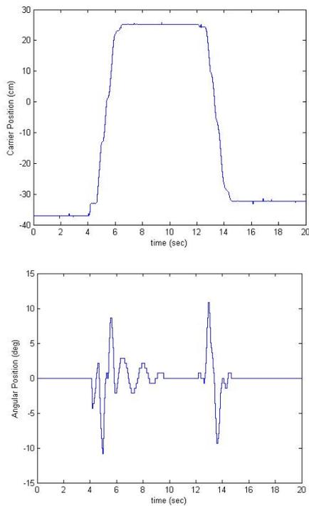
Fig.9. Responses of the trolley position and pendulum's angle based on ZVD ISC ( $m = 100\text{gr}$ )
