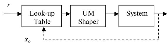
Fig. 7. Input Shaping of the pneumatic crane-pendulum system.
