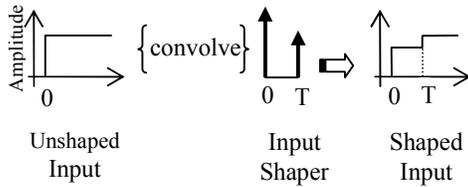
Fig.3. Schematic of input shaping process
