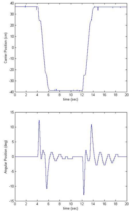
Fig.10. Responses of the trolley position and pendulum's angle based on ZV ISC ( $m = 1\text{kg}$ )
