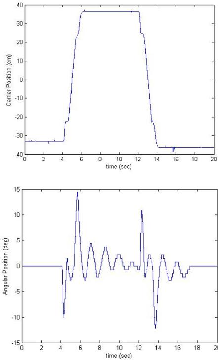
Fig.8. Responses of the trolley position and the pendulum's angle based on ZV ISC ( $m = 100\text{gr}$ )
