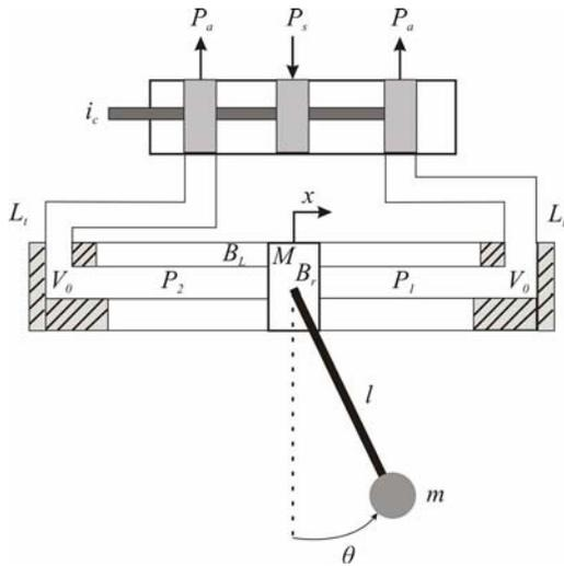
Fig.1. Cylinder-valve system
