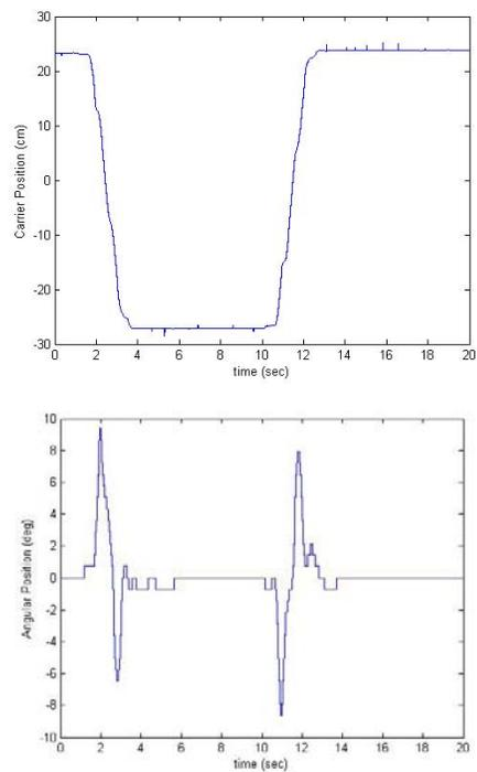
Fig.11. Responses of the trolley position and pendulum's angle based on ZVD ISC ( $m = 1\text{kg}$ )
