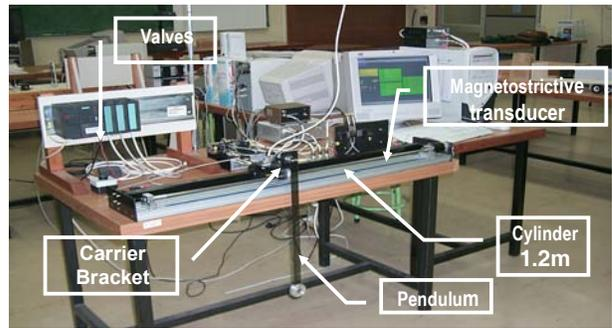
Fig.4. An overall view of the experimental set-up.
