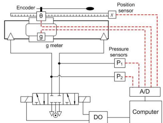
Fig.2. Long pneumatic cylinder with pendulum system
