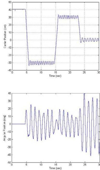
Fig.6. Responses of the carrier position and the pendulum's angle based on on-off control.
