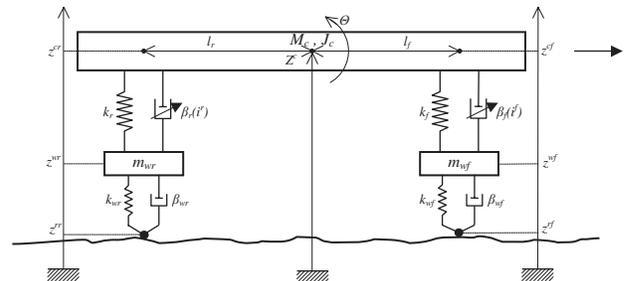
Fig. 1. Half-car semi-active suspension schematic
