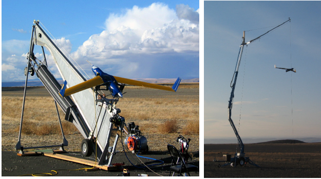
Fig. 3. SeaScan UAV ready for catapult launch (left). SeaScan “landing” using the skyhook system.
