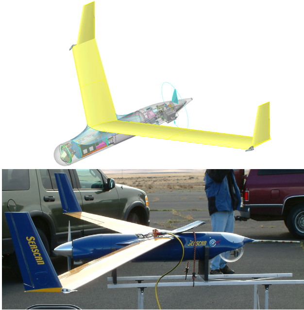
Fig. 2. Transparent view of the SeaScan UAV (top), and the SeaScan prepped for launch (bottom).
