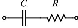
Fig. 50. Compensation network to cancel the right half-plane zero due to the feedforward current through the compensation capacitor.
