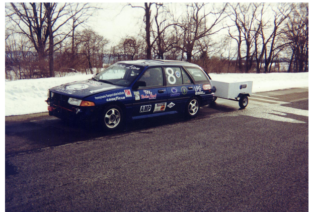
Fig. 7. The Electric Lion series hybrid vehicle used to test the hybrid control strategy.
