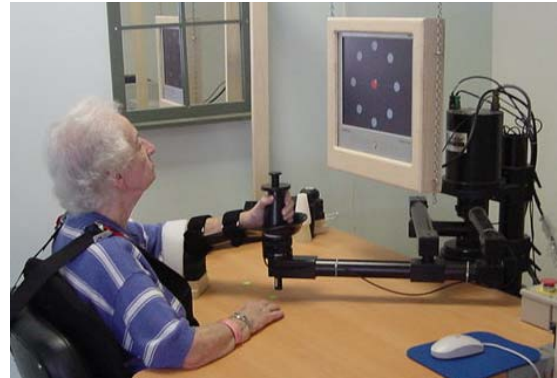
Figure 1. MIT-MANUS robot for shoulder and elbow rehabilitation in the horizontal plane.
