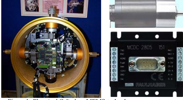
Figure 1. Electrical Cylinders , MEMS-technology servomotor, and VLSI controller-driver
