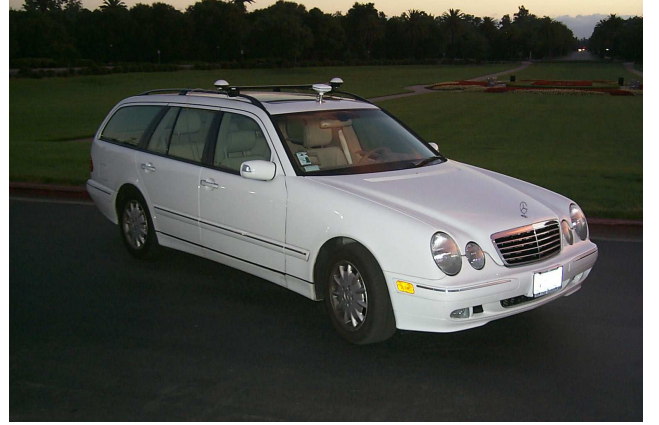
Fig. 3. Test Vehicle with Two-Antenna GPS Set-up
