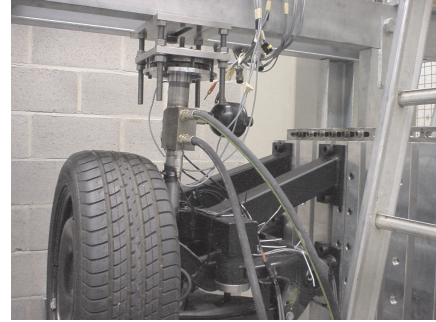
Fig. 3. Picture of the quarter car test-rig equipped with the active suspension.
