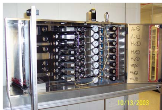
Figure 6. Gas box and its components.
