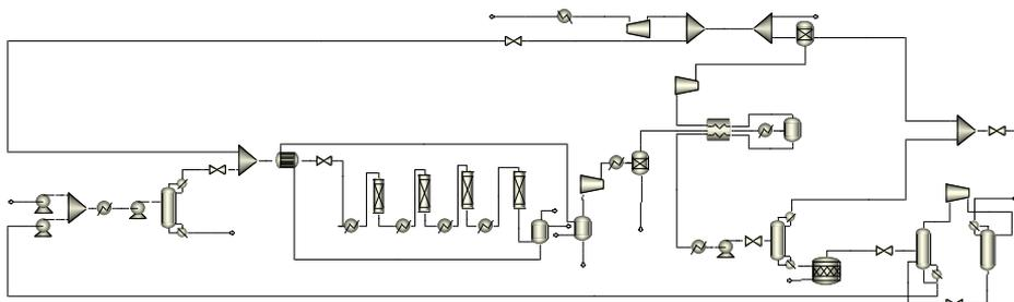
Figure 1. Flowsheet of the PDH process built in Aspen Plus<sup>TM</sup>.
