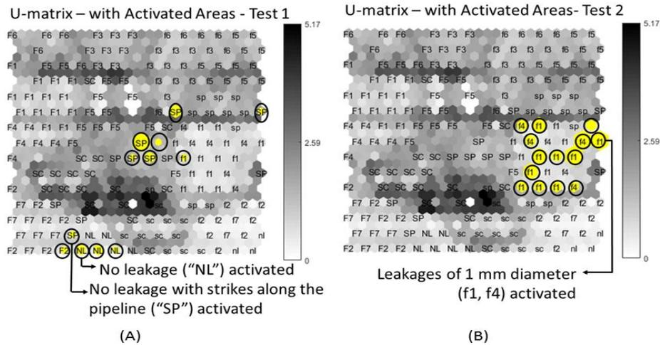
Figure 4. Self-organized map with test results in u-matrix, areas with patterns similar to test data are circled. Test data with (A) beats in the pipeline (B) 1 mm leakage
