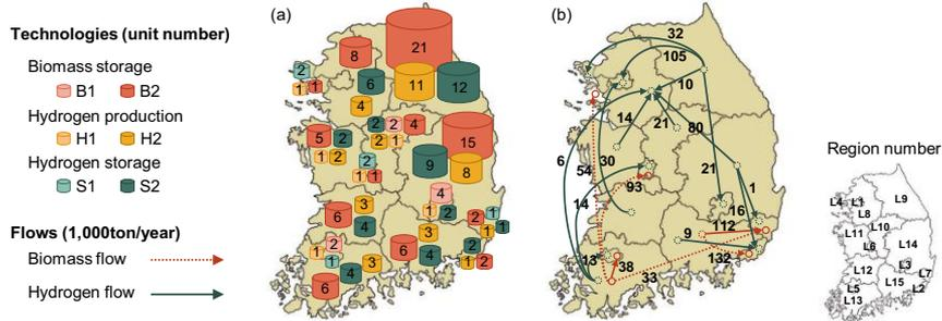
**Fig. 2** (a) System configuration and (b) biomass or hydrogen flows
