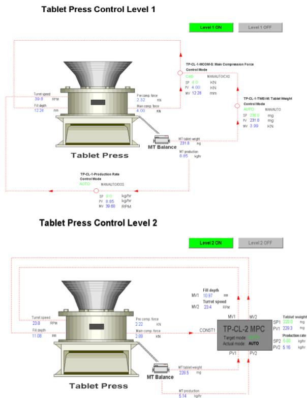
Figure 2. The hierarchical Level 1 (top) and Level 2 (bottom) control for tablet press.
