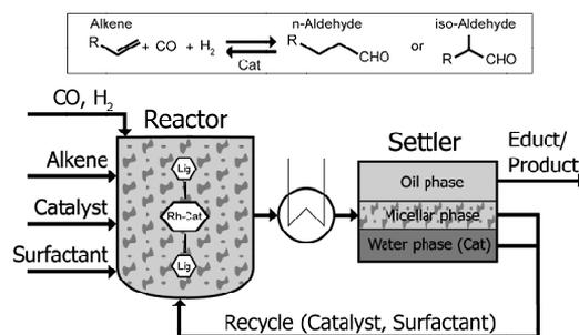
Figure 1: General process concept for the hydroformylation reaction in microemulsions
