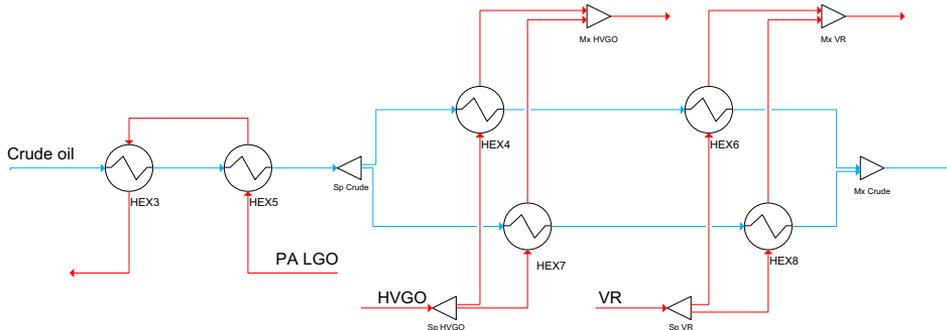
Figure 1. Case study of a refinery preheat train with parallel branches
