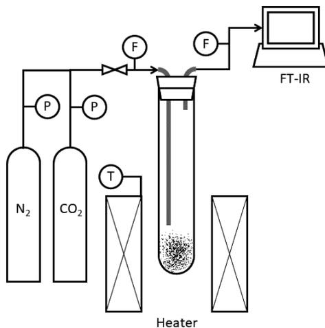
Fig. 2 Experimental setup for absorption reaction
