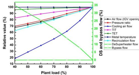
Figure 5 Plant operating variables versus plant load for the optimal strategy.
