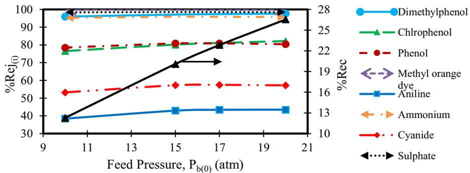
Fig. 5. Operating pressure verses rejection and recovery rate (operating conditions:  $2.583E-4$  m<sup>3</sup>/s, 30 °C, 350 ppm)
