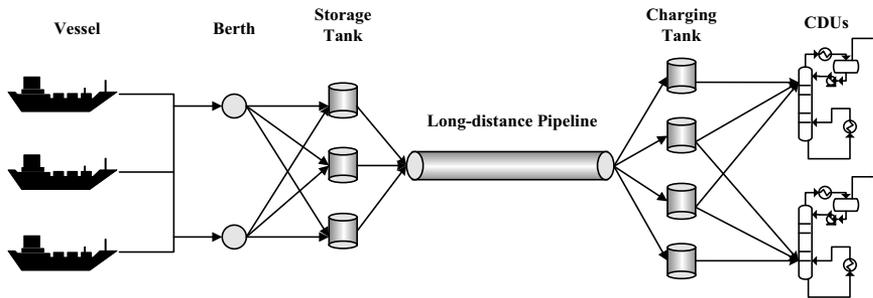
Figure 1. The entire scope of front-end crude scheduling for inland refineries.
