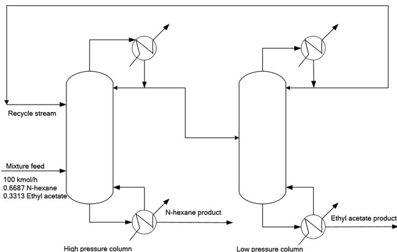
Figure 2. Proposed flowsheet of pressure-swing to separate n-hexane-ethyl acetate mixture
