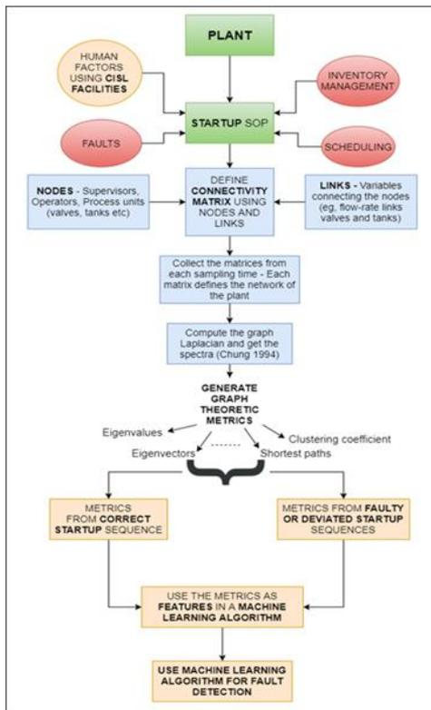
Figure 1. Flowchart of proposed fault detection methodology using process dynamics, graph theory, machine learning and CISL facilities. Color code – Green (available information for any process), Red (external disturbances affecting the startup sequence), Blue (Ongoing work in the lab), Yellow (Future work)
