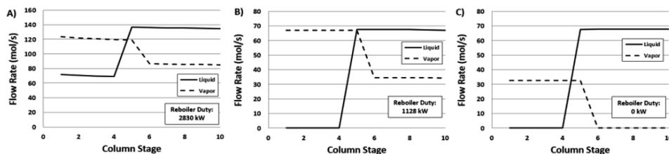
Figure 2: Distillation optimization results for A)  $x_{\text{benzene,top}}, x_{\text{toluene,bottom}} \geq 0.90$ , B)  $x_{\text{toluene,bottom}} \geq 0.80$ , and C)  $x_{\text{toluene,bottom}} \geq 0.57$ .
