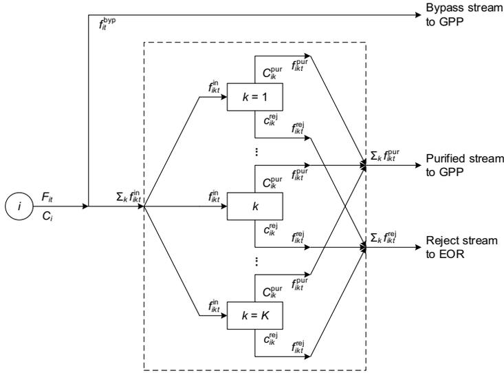
Figure 1. Schematic of Gas Sweetening
