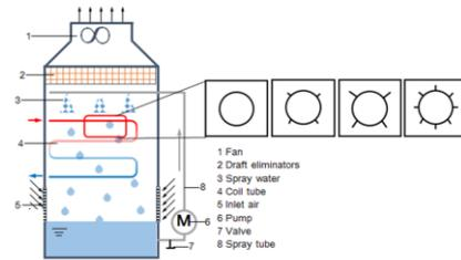
Figure 1 Schematic of the closed wet cooling tower
