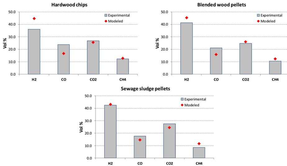
Figure 2. Validation of product gas composition from different feedstocks.
