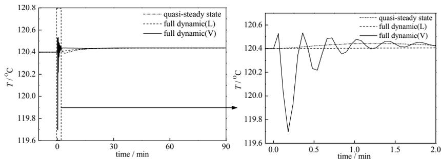
Figure 5. Dynamic response of reactor in quasi-steady state and full dynamic model
