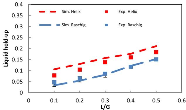
Figure 3 The validation of the liquid holdup of helical rings and Raschig rings
