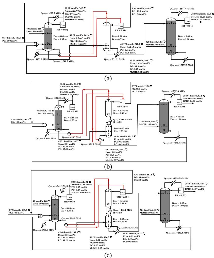
Figure 4. Optimal design for (a) RD+CD\_HI1, (b) RD+CD\_HI2, and (c) RD+CD\_HI3 configurations.
