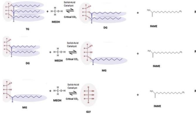
Figure 2. Kinetic mechanism involving three reversible reactions. TG is triglyceride (triolein), MEOH is methanol, DG is diglyceride (diolein), FAME is fatty-acid methyl-ester (methyl oleate – biodiesel), MG is monoglyceride (monoolein), GLY is glycerol, and critical  $\text{CO}_2$  is in or near the critical region
