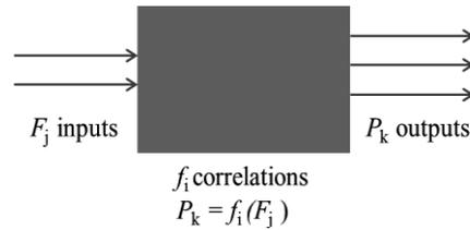
Figure 3. A technology unit represented by inputs ( $F_j$ ), outputs ( $P_k$ ) and relations  $f_i$  that connect them.
