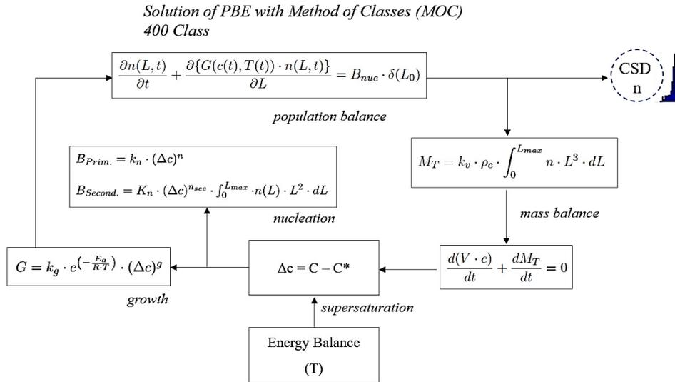
Figure 2. Batch cooling crystallization model (Adapted from Giuletti et al., 2001).
