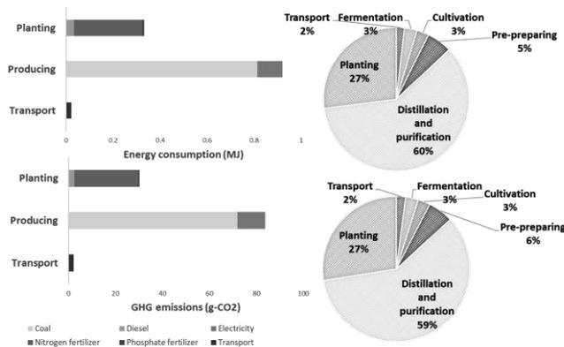
Figure 2. GHG emission and energy consumption in each production process of ASSF.
