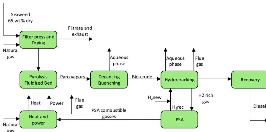
Figure 1. Block flow diagram of the fast pyrolysis route
