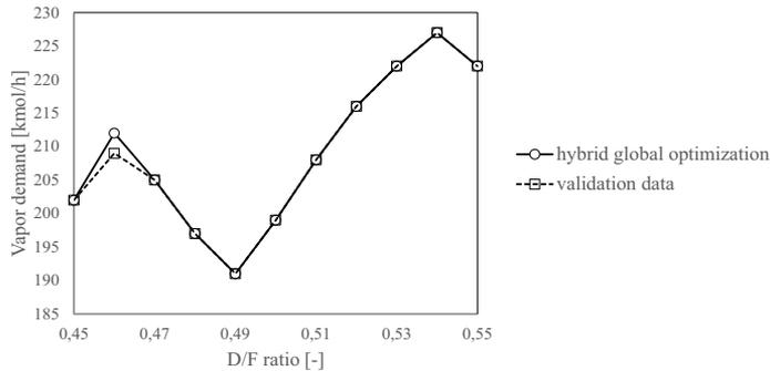
Figure 4: Results of the optimization of the vapor demand of a reactive distillation of the hybrid global optimization method in comparison to validation data
