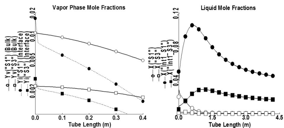
Figure 3. Initial negative condensing fluxes of S1 and S3 (left) and liquid species (right).
