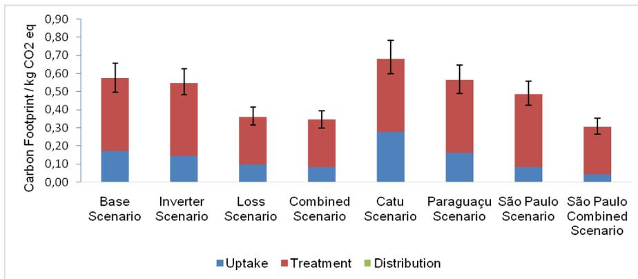
**Fig. 3** Impact contribution of Carbon Footprint with uncertainty (background and foreground) of 1 m<sup>3</sup> of distributed water per stage along the life cycle for each scenario
