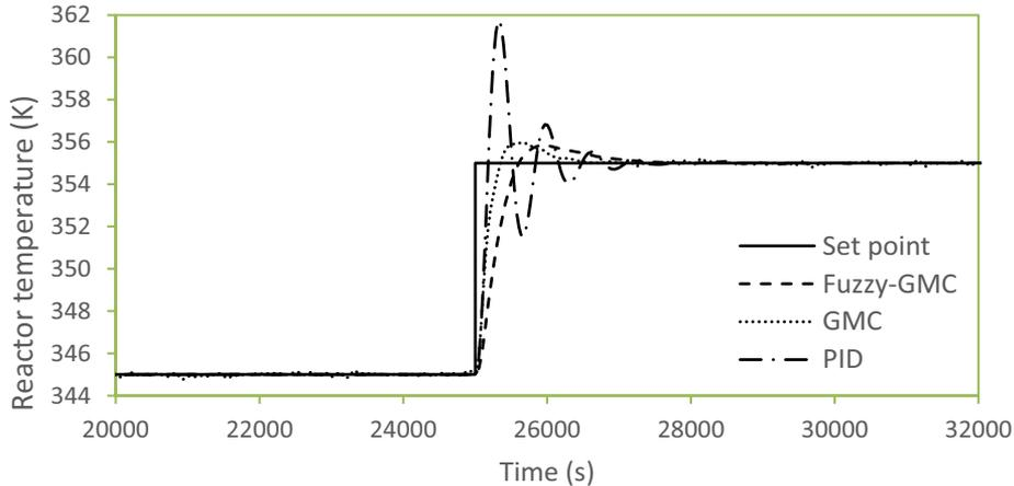
FIGURE 3. Performance comparison of GMC, Fuzzy-GMC Hybrid and PID controller in set point tracking. (PID setting are as follows:  $K_c = 24.24$ ,  $\tau_i = 129.5$ ,  $\tau_D = 32.37$ )
