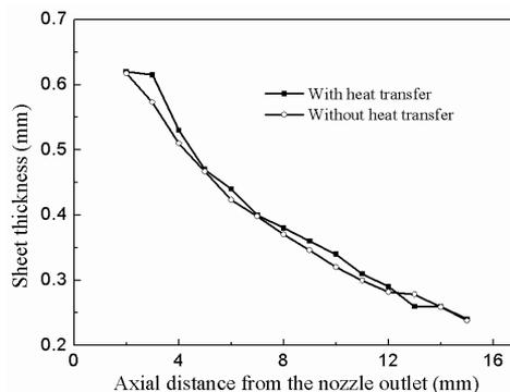
Figure 5: Profile of sheet thickness along the flow direction
