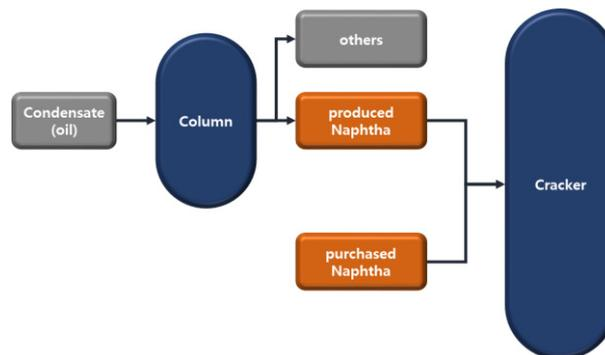
Figure 2. Process diagram for naphtha supply
