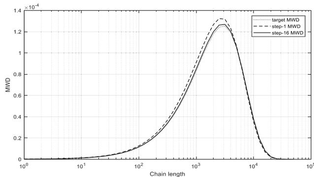
Figure 4. MWD curves of the target, step-1 and step-16 (optimum) points.
