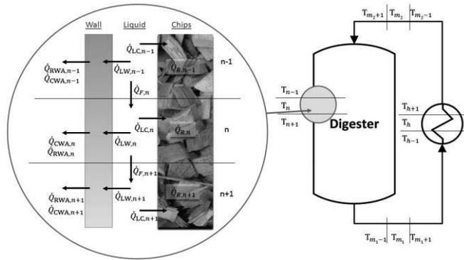
Figure 1. Right: Digester system liquid circulation. Left: Direction of the simulated thermal energy fluxes inside the reactor vessel. The wood chip fraction is absent in the pipes and the heat exchanger.
