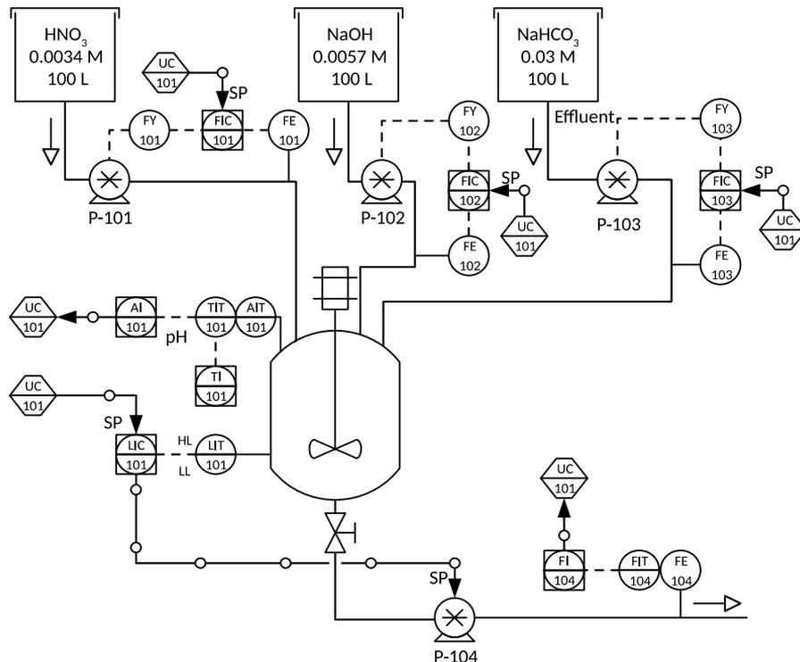
Figure 1 – Instrumentation diagram of the pH neutralization plant.
