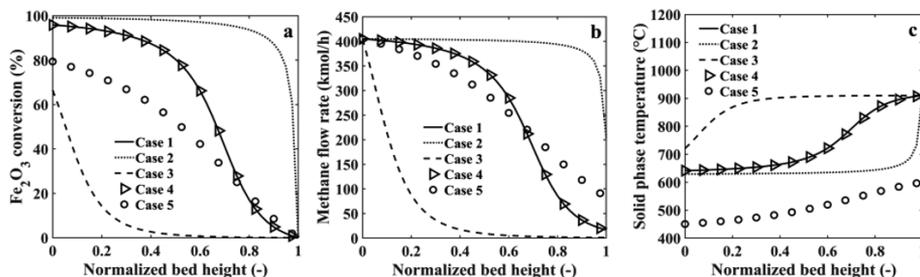
Figure 1. (a) Fe<sub>2</sub>O<sub>3</sub> conversion, (b) CH<sub>4</sub> molar flow rate, and (c) solid temperature profiles along the normalized length of the reactor bed (gas inlet:  $z = 0$ , solids inlet:  $z = 1$ ).
