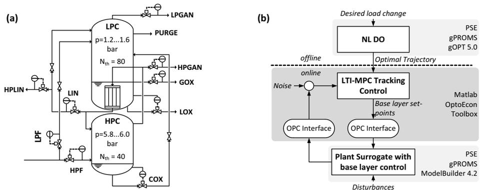
Figure 1: (a) Flowsheet of the ASU considered in this work. (b) Two-layer APCS incorporating offline nonlinear dynamic trajectory optimizations (NL DO) and online tracking control using a linear time-invariant model predictive controller (LTI-MPC).
