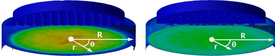
Figure 4. (left) Cross section of  $\text{SiH}_3$  concentration taken just above the surface of the wafer substrate (right)  $\text{SiH}_3$  concentration above the wafer surface for the adjusted reactor geometry.
