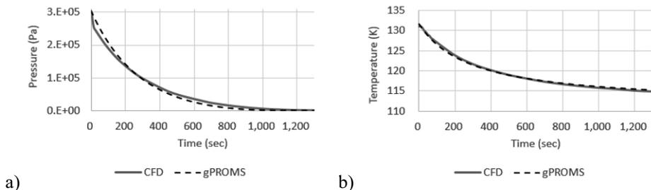
Figure 4. Comparison of CFD and gPROMS simulation results, a) outlet pressure, b) liquid temperature
