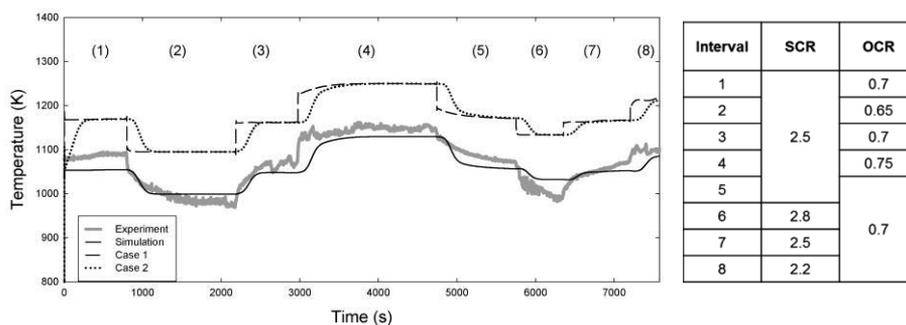
Figure 3. Temperature profile at reformer exit compared with experimental results in the sequence of step changes. Adiabatic simulation results (dotted line) and non-adiabatic simulation results (solid line). Step change details are listed in the table.
