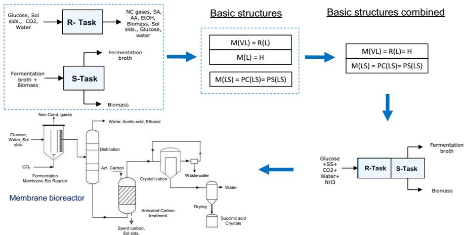
Figure 4. Intensified flowsheet alternative 1 (Identified task, combination of basic structures)
