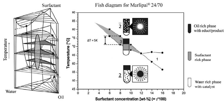
Figure 2: Left: Gibb's phase prism for oil, water, and a nonionic surfactant. Grey areas indicate three phasic miscibility gaps. Taken from (Stubenrauch et al., 2009). Right: Kahlweit's Fish plot with temperature dependent separation regimes for the applied component system. Adapted from (Pogrzeba et al., 2017)
