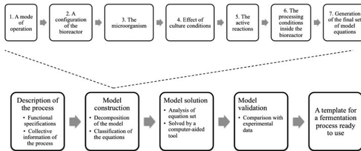
Figure 3. Workflow for the model construction of fermentation.
