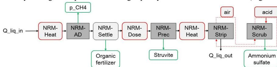
**Figure 1** Optimal treatment train configuration targeting bio-based struvite and ammonium sulfate fertilizer production; Red = consumable (= cost); Green = recovered resource (= revenue); AD = anaerobic digestion; Dose = chemical dosing; Heat = heat exchanger; Prec = precipitation/crystallization; p = partial pressure in the biogas;  $Q_{liq}$  = liquid flow rate; Scrub = scrubber; Strip = stripper.
