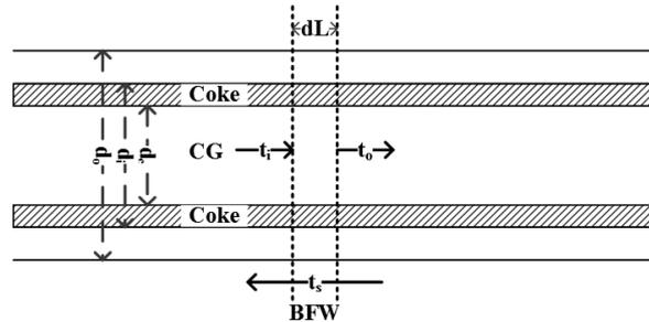
Figure 1. Schematic diagram of TLE tube.
