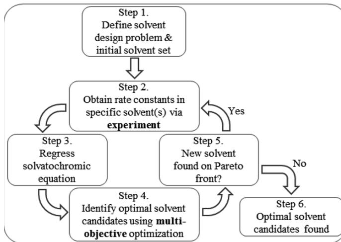
Figure 1: Empirical-CAMD algorithm for identifying optimal solvents for reaction productivity where the solvent influences multiple reaction parameters of interest.
