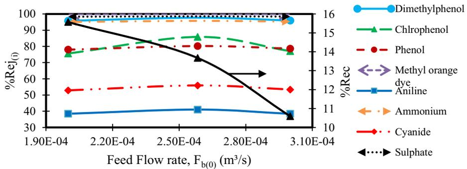
Fig. 6. Effect of operating feed flow rate on rejection and recovery rate (operating conditions: 10 atm, 30 °C, 350 ppm)
