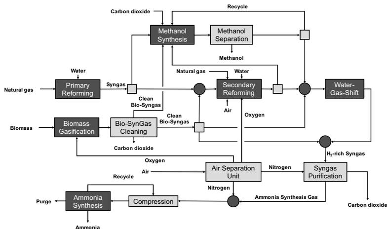
Figure 1. Process superstructure for Biomass/Natural Gas to Ammonia and Methanol
