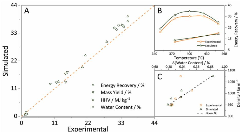
Figure 2. Validation of the automated reduction method. Dependence of A) experimental and simulated validation parameters, B) simulated and experimental energy recovery in respect to pyrolysis temperature, and C) difference in simulated and experimental water content.
