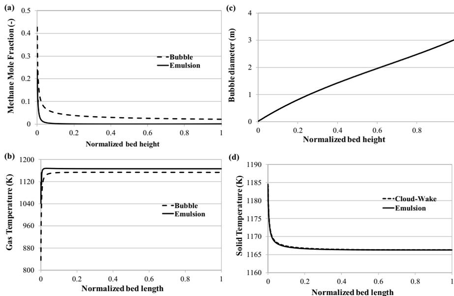
Figure 1. Profile data of selected variables vs. bed height (a) Methane mole fraction (b) Gas velocities (c) Gas Temperatures (d) Solid Temperatures
