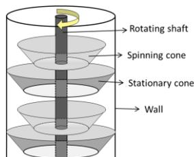
Figure 1. Simplified scheme of Spinning Cone Column
