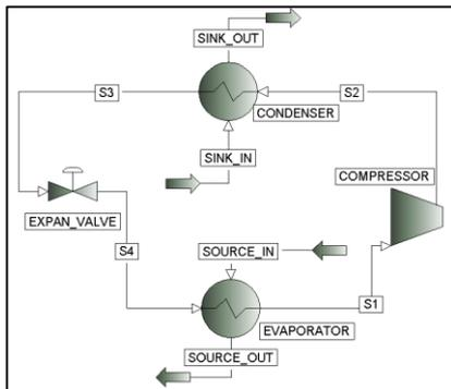
Figure 1: Pro/II flowsheet of a heat pump.
