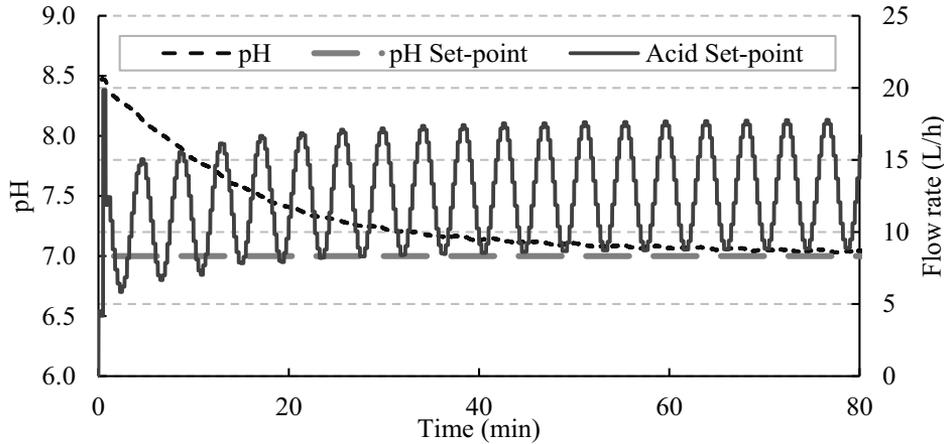
Figure 3 – SISO experimental results. Acid flow rate (FIC-101) as manipulated variable.
