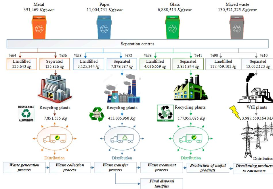
Figure 1. Schematic of considered municipal solid waste management supply chain network
