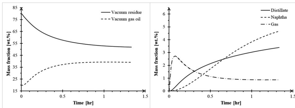
Fig. 5. Concentration of species with time at bubble column exit.
