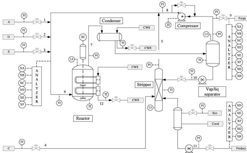
Figure 3: Schematic diagram of Tennessee Eastman model
