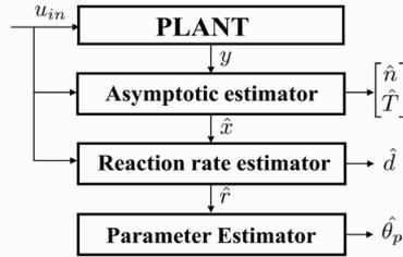
Figure 1. State and parameter estimation structure of Extent-Based LPV systems
