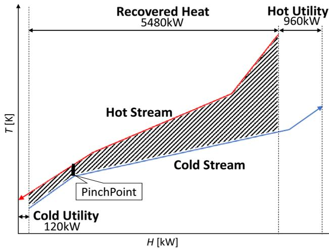
Figure 2: Composite curves of 4SP1.
