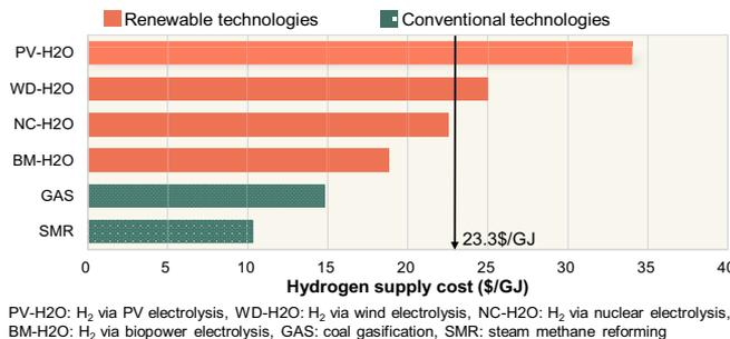
**Fig. 4** Comparison of hydrogen supply cost in different technologies
