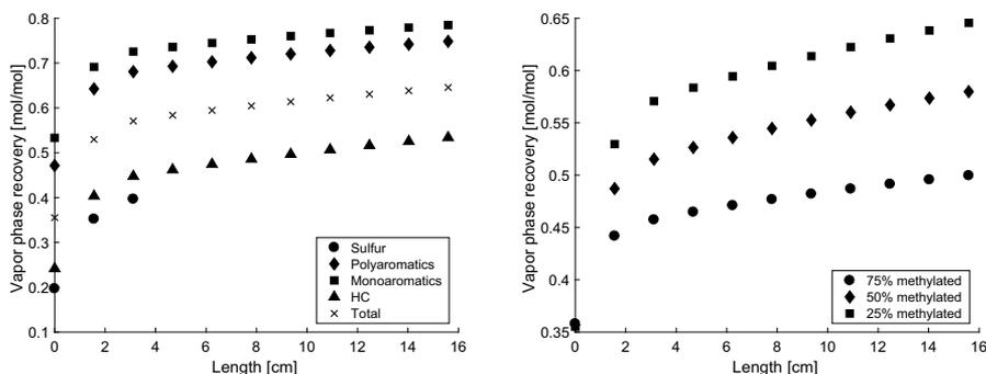
Figure 1 Calculated vapor recovery profiles of oil species in simulations neglecting evaporation. The plots present an overview of the individual species at 25 wt.-% methylated feed (left) and the recovery of oil species at different levels of methylation (right).
