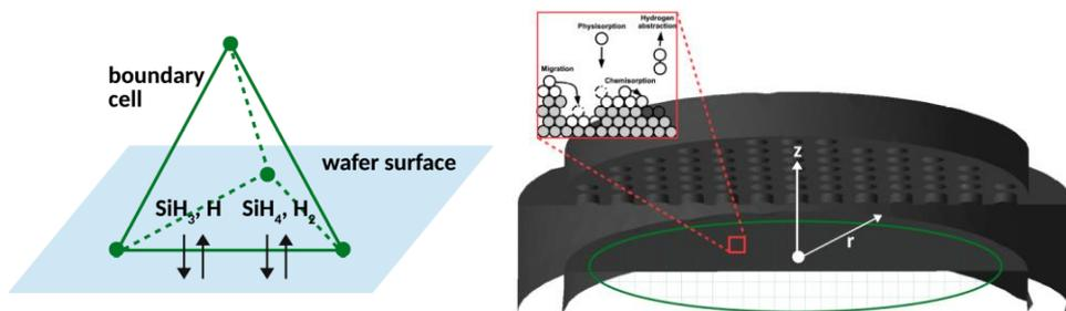
Figure 2. (left) Finite element adjacent to the substrate surface with dynamic boundary condition calculated via microscopic simulation domain. (right) Kinetic Monte Carlo setup within overall multiscale simulation. Wafer substrate discretized in both the  $x$  and  $y$  directions forming a ‘grid’ structure.
