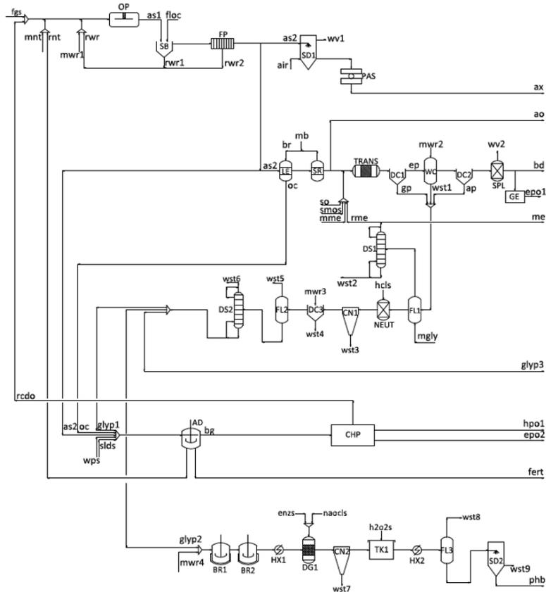
Figure 1. Integrated microalgae-based biorefinery superstructure
