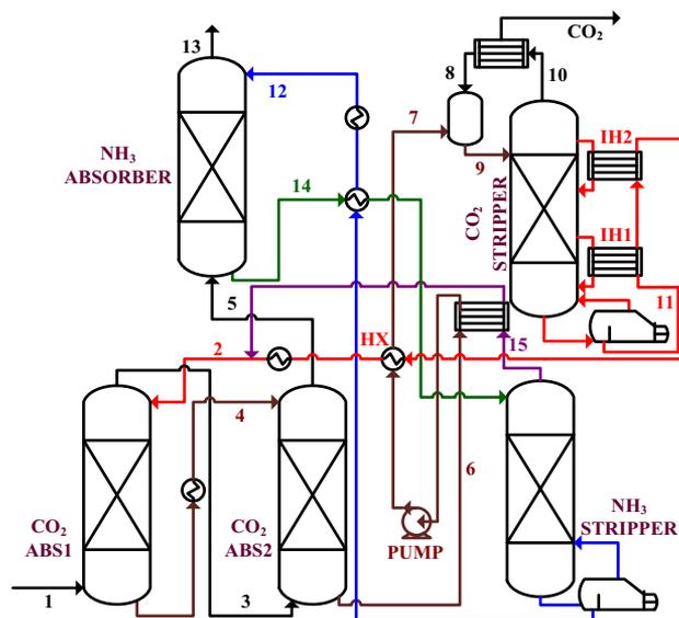
Figure 1. The integrated PCC process with the additional inter-heaters.
