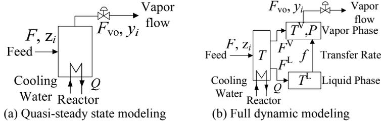
Figure 3. Schematic of quasi-steady state and full dynamic modeling in reactor
