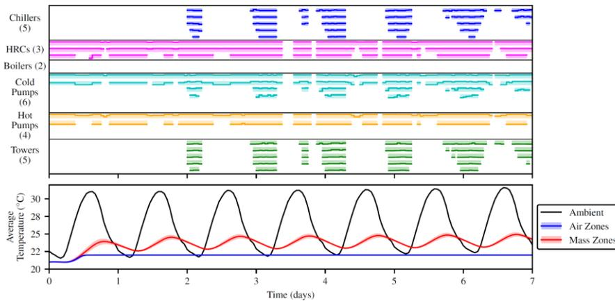
Figure 3: Hierarchical decomposition solution for big instance. Temperature plot shows average  $\pm$  standard deviation for 500 air and mass zones.
