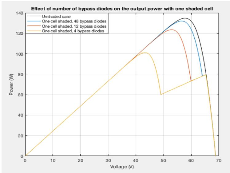
Figure (3): P-V curve for one shaded cell at different bypass diodes
