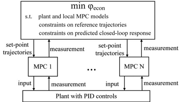
Figure 1: The control architecture for coordination of distributed MPCs with closed loop DRTO approach.
