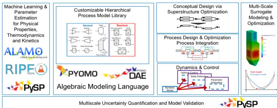
Figure 1. The major components and connection of the IDAES PSE Framework to support conceptual design, process design & optimization, process integration, dynamic optimization, and control while incorporating multi-scale surrogate models.
