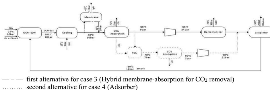
**Figure 1.** Schematic representation of the OCM covering four process structures
