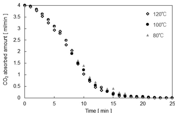
Fig. 3 Rate of CO<sub>2</sub> absorption as a function of time for different reaction temperature
