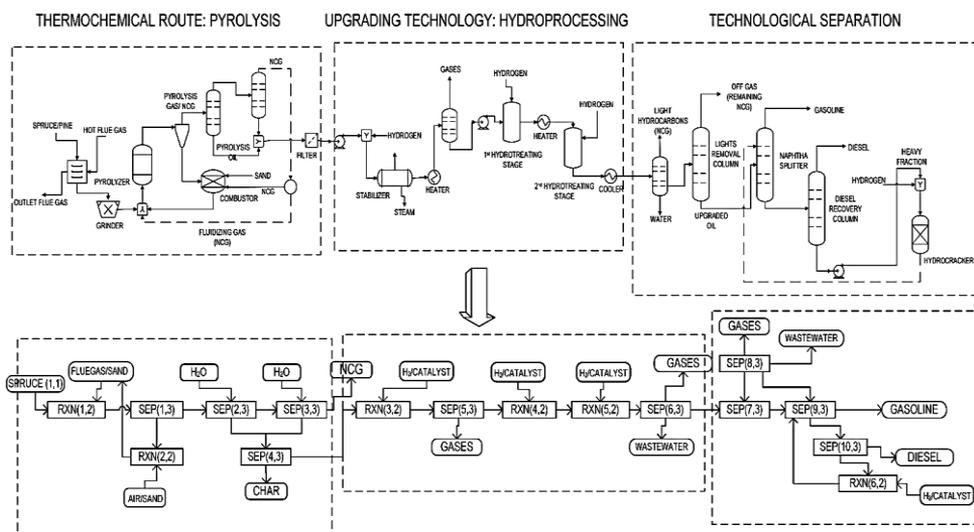
Figure 1. Formulation of processing blocks for BC-PHS: reaction (RXN) and separation (SEP)
