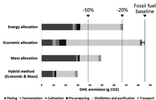
Figure 3. GHG emissions for ASSF using different allocation methods.
