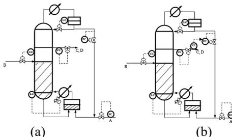
Figure 4. Control systems of RDC-TBER, (a) CS1, (b) CS2
