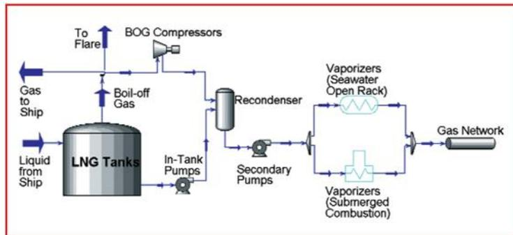
Figure 1. LNG regasification terminal
