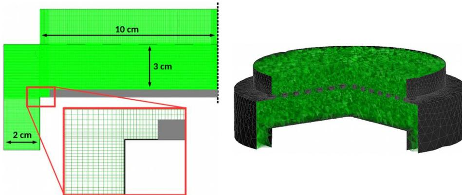
Figure 1. (left) 2D axisymmetric geometry after discretization using a structured mesh containing 120,000 cells. (right) Collection of 1.5 million polygons which define the unstructured, 3D mesh.
