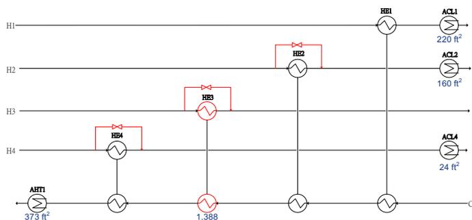
**Figure 3.** Refined HEN design obtained by introducing area margin to HE3.
