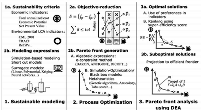
Figure 1. Framework for the optimal design of sustainable processes.
