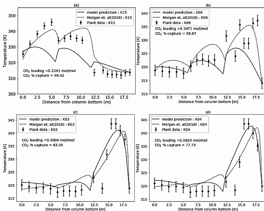
Figure 3: Packed Column Temperature Profiles, this work, National Carbon Capture Center Data, and Morgan et al. (2018)
