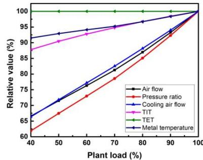
Figure 4 Plant operating variables versus plant load under IGVC.
