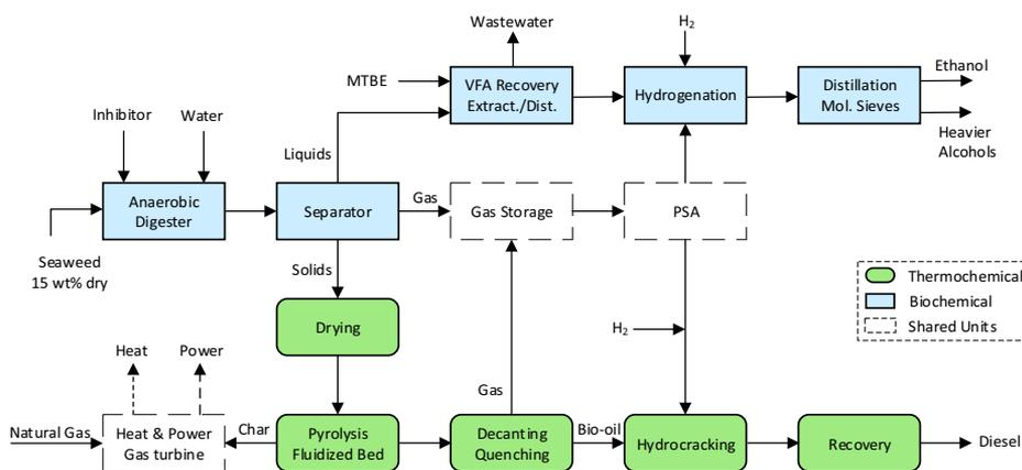
Figure 2. Block flow diagram of integrated process
