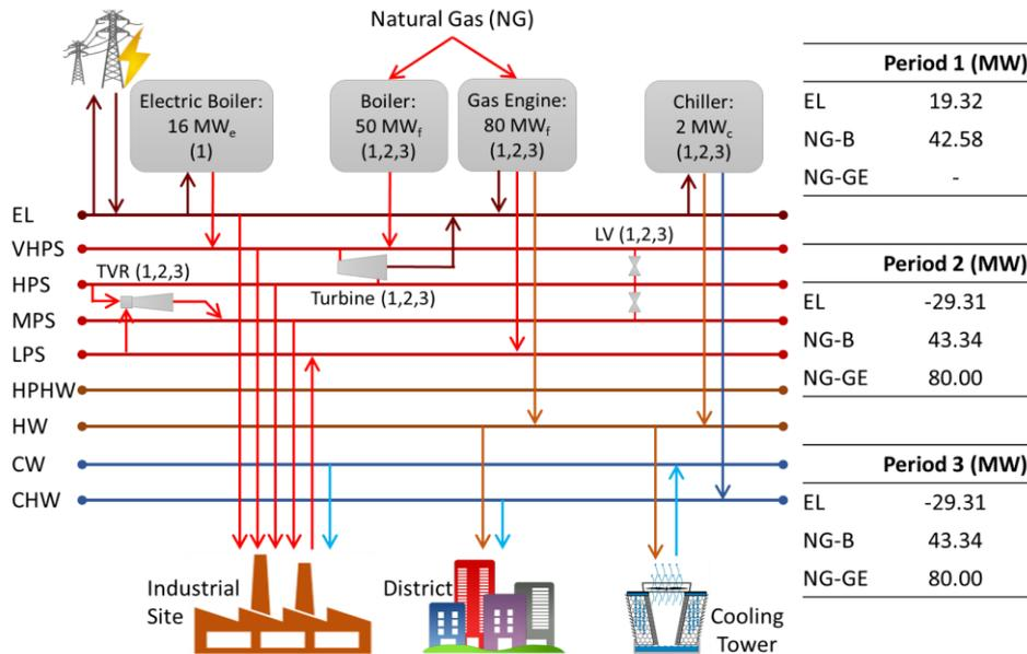
Figure 4: Utility systems structural design with key fuel and equipment for minimum TAC.
