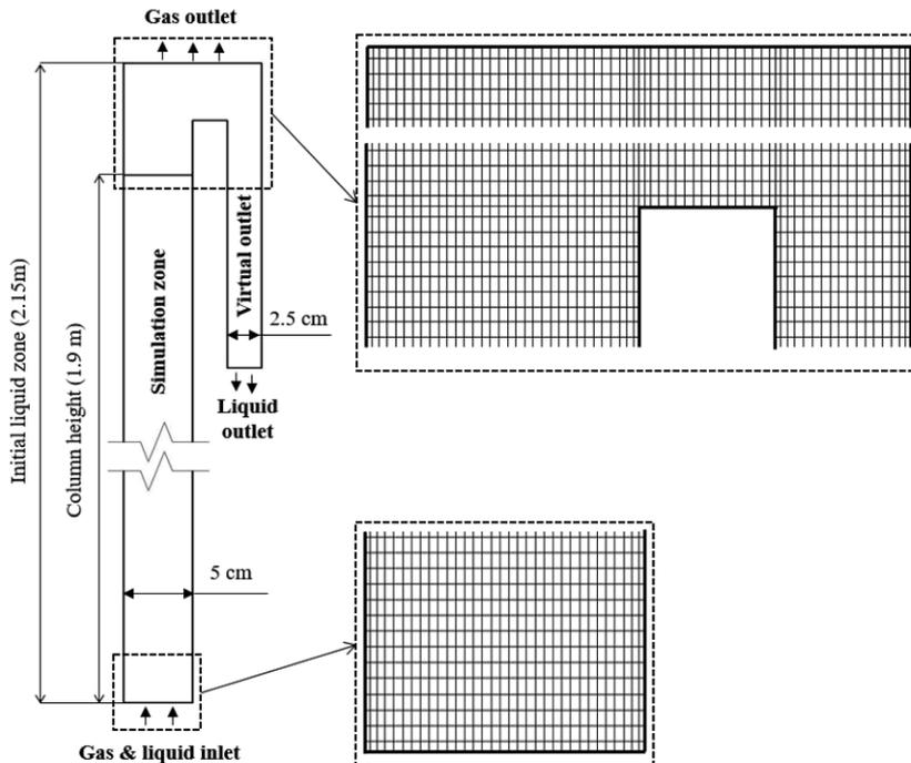
Fig. 1. Geometry and meshing of CFD calculation domain
