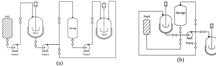
Figure 1 (a) Conventional pump allocation and (b) proposed pump allocation
