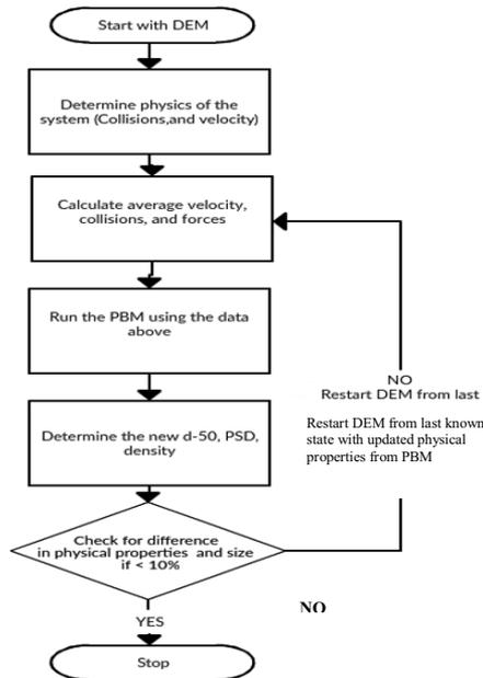
Figure 1: Schematic of the bi-directional approach used to model the high shear granulator.
