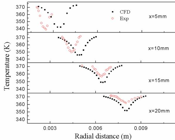
Figure 6: Comparison of the simulated temperature profiles with experimental data at various axial distance ( $x$ ) from the nozzle outlet
