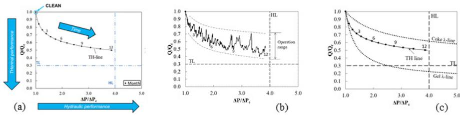
Figure 4. Thermo-hydraulic plot and reference lines are useful for monitoring and diagnosis (Diaz-Bejarano *et al* 2016b).
