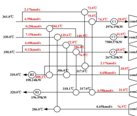
Figure 4 The simultaneous optimized network
