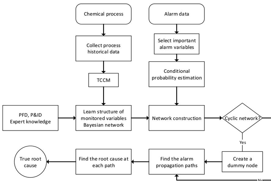
Figure 2: Proposed method for the root cause analysis of alarms
