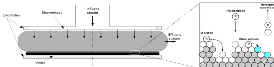
Figure 1. Macroscopic (left) and microscopic (right) PECVD simulation regimes.
