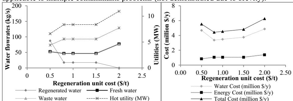
Figure 2 Effect of regeneration cost on flow rate and utilities
