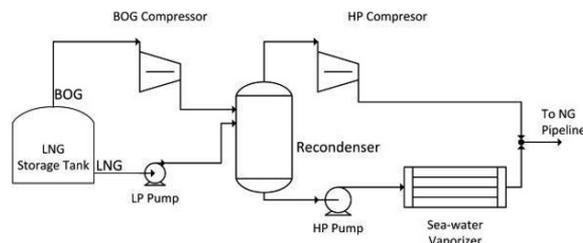
Figure 1: A typical LNG regasification terminal
