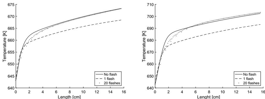
Figure 2 Liquid temperature profiles with or without flashes. The plots present the feed with 75 wt.-% (left) and 25 wt.-% methylated substrate (right).
