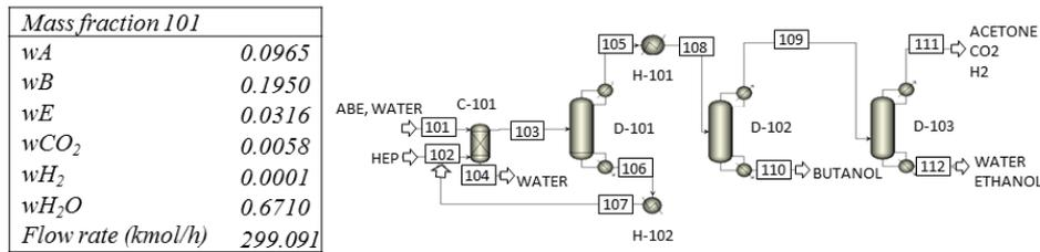
Figure 2. Process configuration for the ABE separation using HEP as extractant agent.
