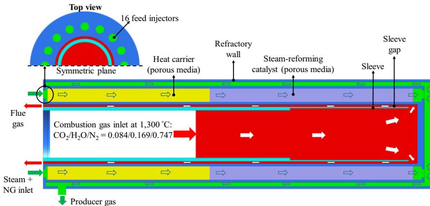
Figure 1. Geometry and mesh structure of compact SMR process.
