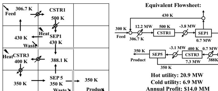
Figure 4. Solution obtained from the original superstructure.
