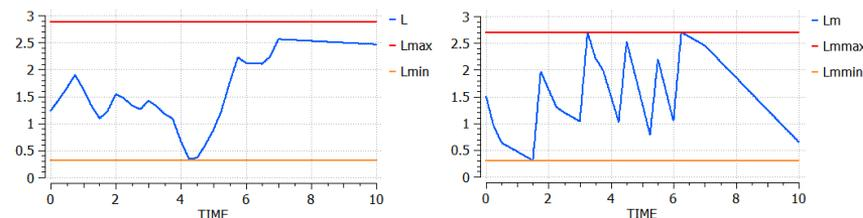
Figure 4. Time evolution of the levels in the supply tank (left) and strike receiver (right) with the corresponding upper and lower limits.
