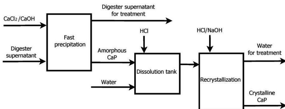
Figure 2. Two-step fast precipitation/recrystallization technology.
