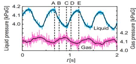
Figure 3 Gas and liquid feed pressures
