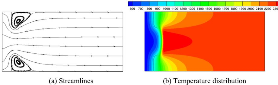
Figure 5: Streamlines and temperature distribution in micro-combustor with baffles
