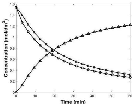
Figure 2: Concentration profiles of the species using the true and estimated values (o –  $C_{EC}$ , □ –  $C_{BZ}$ , Δ -  $C_P$ , solid lines represents the concentrations obtained by the estimated values.)
