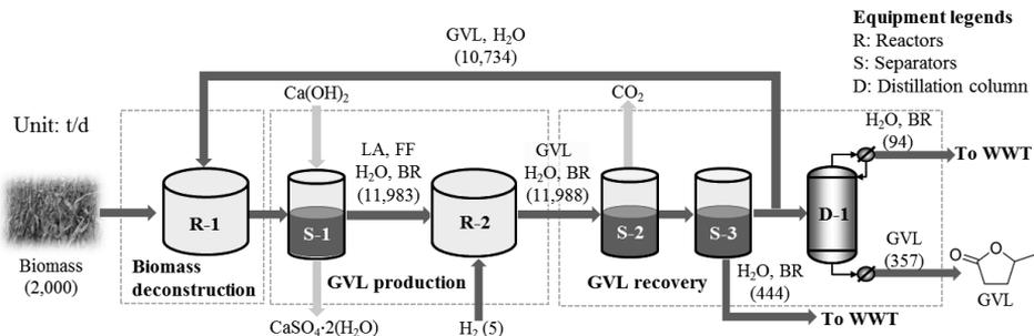
**Figure 3.** Simplified process flow diagram of LA-based GVL production process.
