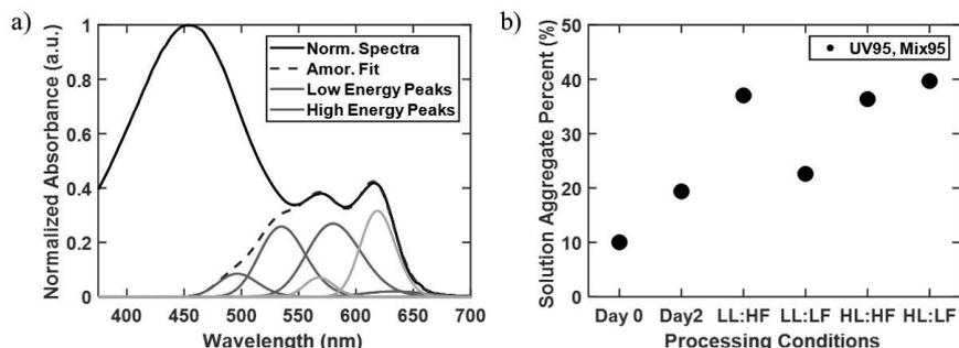
**Figure 2.** (a) Normalized solution UV-vis absorbance spectra of LL:LF sample deconvoluted into amorphous and aggregate contributions. (b) Solution aggregate percent for both batch and continuous flow processing experiments. The standard errors over multiple replicates were all less than 1.15 %.
