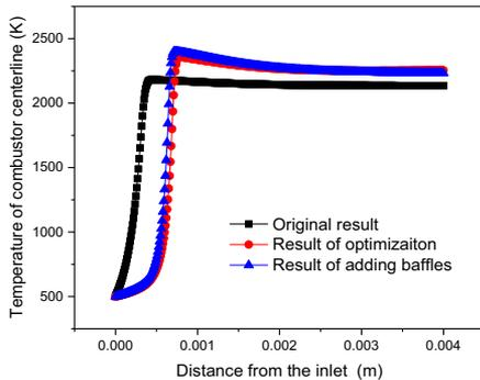
Figure 6: Centerline temperature profile comparison with the results of optimization, adding baffles and original results
