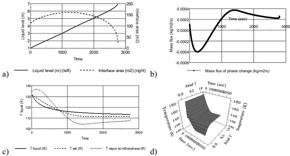
Figure 5. Dynamic simulation results of developed LNG tank model, a) interphase tracking, b) mass flux of phase change, c) interphase temperatures, d) vapor temperature profile in a tank
