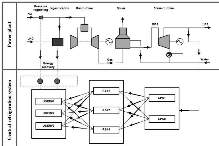
Figure 1. Flowsheet of natural gas power plants and superstructure of CRS
