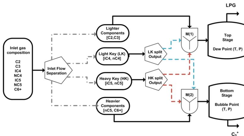
Figure 2. Scheme of the Two-Flash Process Model (TFPM) used for the SRSS.
