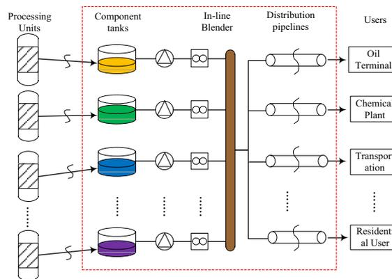
Fig. 1 Illustration of on-line blending and distribution process in a refinery
