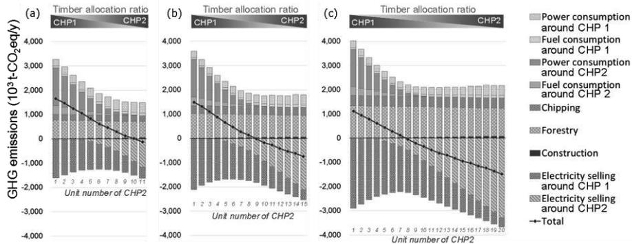
Figure 2 LC-GHG based on the forest resource allocation in Tanegashima to CHP1 and CHP2, where three patterns of resource availability were considered: (a) 15,700 m<sup>3</sup>-timber/y, 21,100 m<sup>3</sup>-timber/y, and 27,600 m<sup>3</sup>-timber/y. Although GHG emitted from fossil resources was considered in LC-GHG, that from the feedstock of biomass was not included on this graph.
