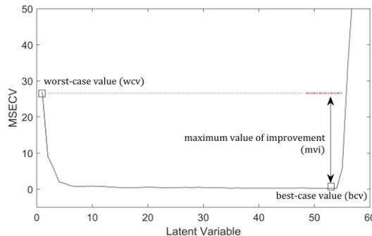
Figure 1. Illustrative example of a typical MSECv curve
