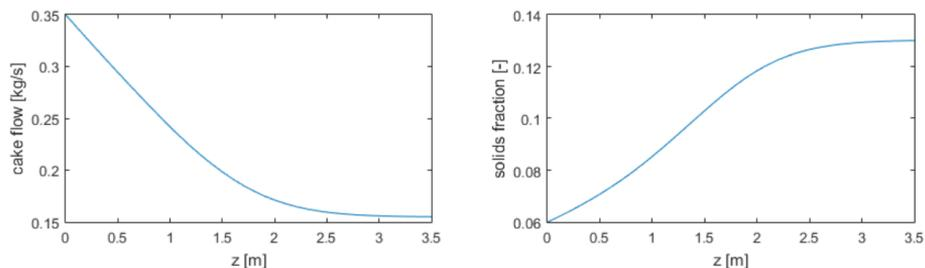
Figure 2. Cake flow (left) and solids fraction (right) simulation results for the developed model
