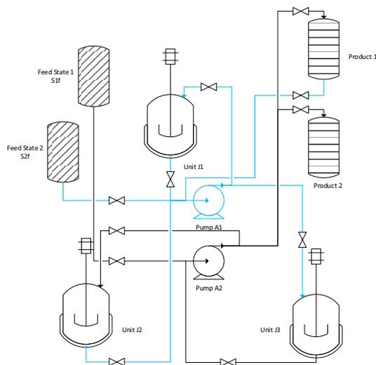
Figure 6 Optimal floating pump allocation and connections
