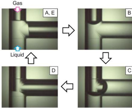
Figure 4 Photos of flow behavior in the mixer
