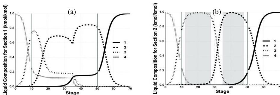
Figure 2. Liquid composition profiles of the Kaibel Column. (a) Liquid composition profiles of the main column with section 1 of the dividing wall. (b) Liquid composition profiles of the main column with section 2 of the dividing wall.
