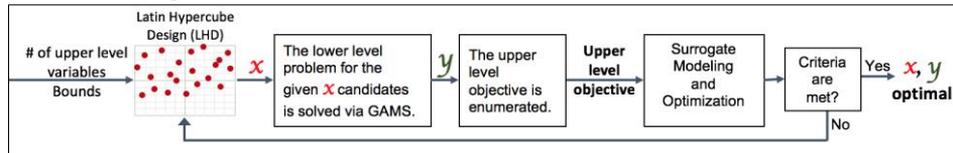
Figure 2 Illustration of the main steps of the Data-Driven Bi-level algorithm
