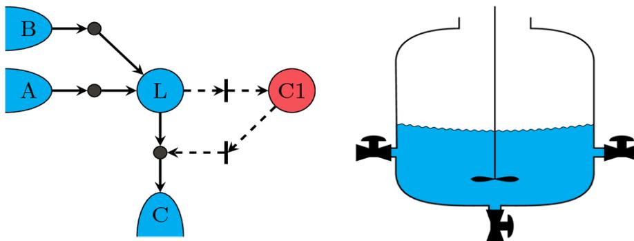
Figure 4. Illustration of the modelled mixing tank and the corresponding topology generated.
