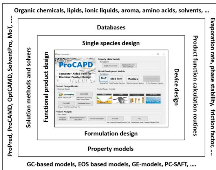
Figure 4: Structure of ProCAPD (design options, models-calculation routines, tools)
