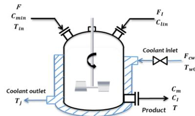
Figure 7. Polymerization reactor flow sheet
