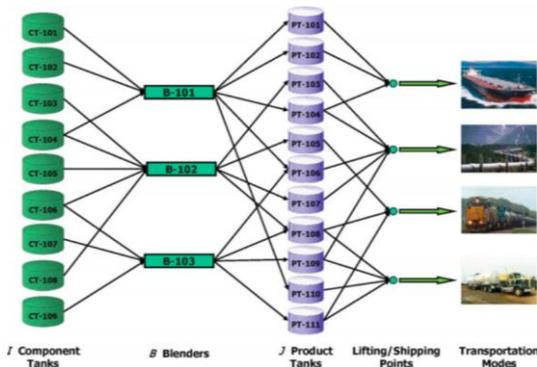
Figure 1 Schematic of a general gasoline blending, storage and order delivery in an oil refinery
