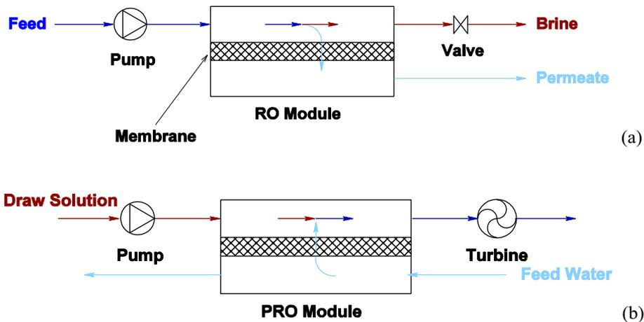
Fig. 1 Schematics of (a) RO for seawater desalination and (b) PRO for power generation.
