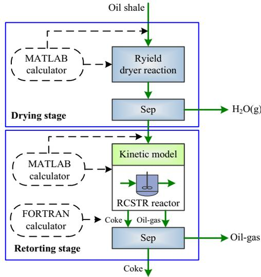
Figure 3. Aspen Plus simulation calculation procedure
