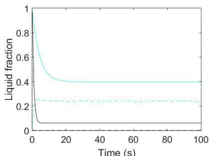
Figure 4. Liquid fraction of the electrodes: anode solid line; cathode (\*10E4) dashed line.  $j_{el} = 0.1 \text{ Acm}^{-2}$  (lighter)  $j_{el} = 1 \text{ Acm}^{-2}$  (dark)
