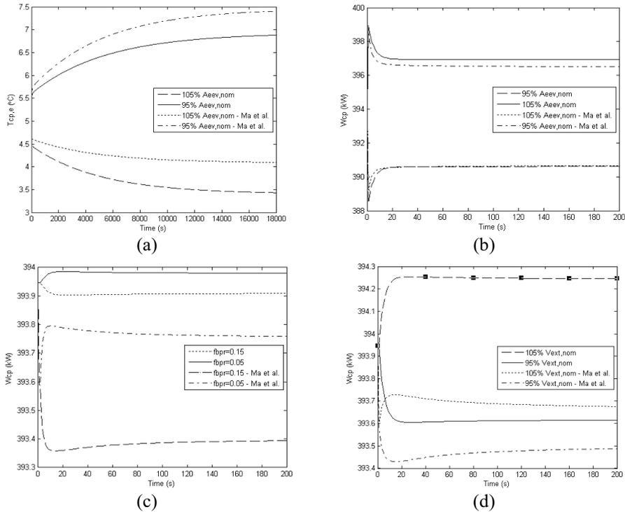
Figure 2: Responses to step changes in manipulated variables in open-loop: (a) EEV effect on compressor suction temperature (b) EEV effect on compressor shaft power (c) Changes in water bypass fraction effect (d) External air flowrate into condenser effect
