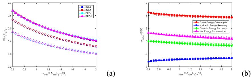
Fig. 6 Optimal (a) dimensionless flux and (b) dimensionless energy consumption (positive) and recovery (negative) in two-stage RO-PRO under different  $\eta_{PRO}$  (100%, solid symbols and 70%, hollow symbols) at 30% water recovery.
