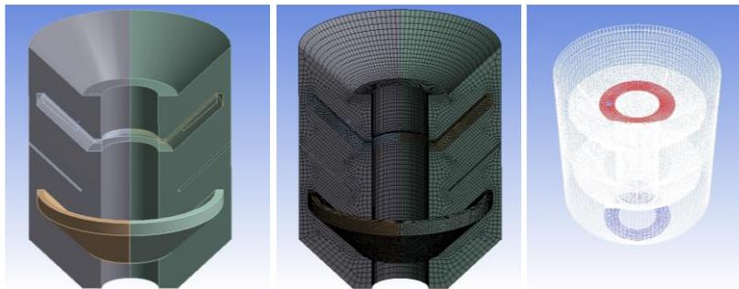
Figure 2. Details of CFD modeling: Geometry, meshes, and boundaries from the left
