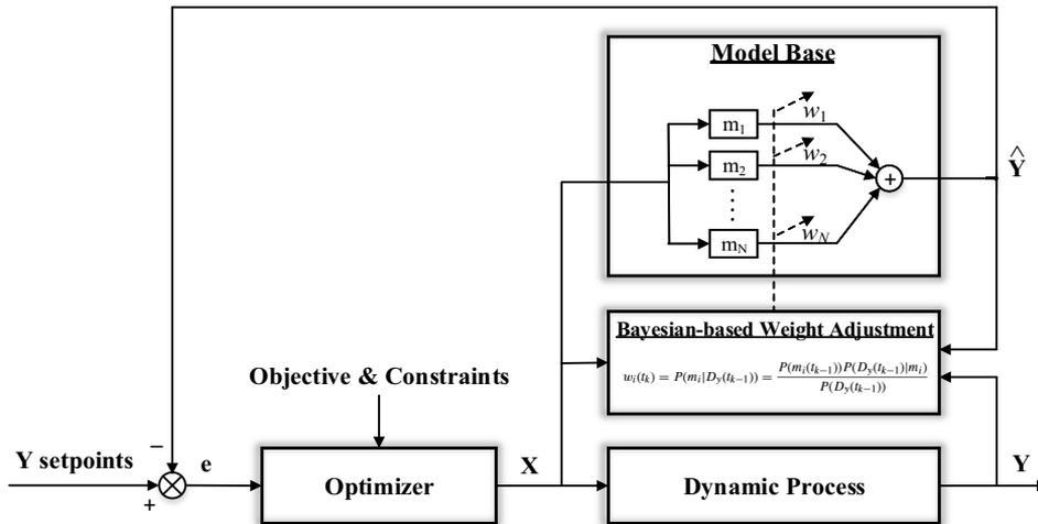
Figure 1 Bayesian-based model evaluation in the model based control diagram
