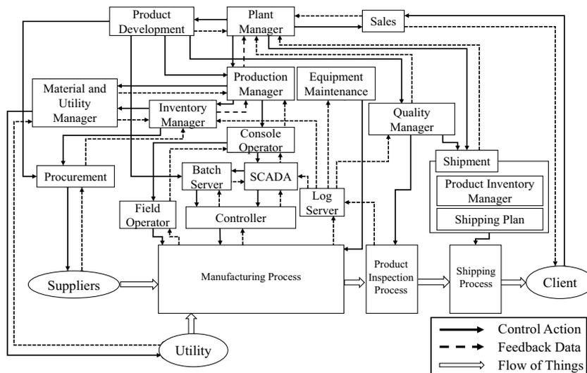
Figure 1: Control Structure Diagram of Batch Plant
