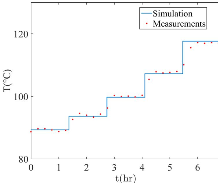
Figure 1: Optimal profiles of reactor temperature for  $GE_f = 60\%$  and  $X_f = 80\%$ .
