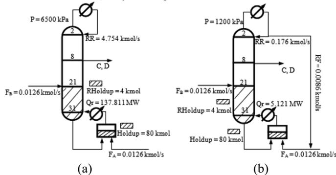
Figure 1. Process synthesis and design. (a) CRDC, (b) RDC-TBER
