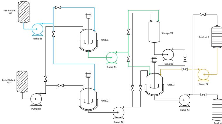
Figure 3 Conventional pump allocation and plant flowsheet
