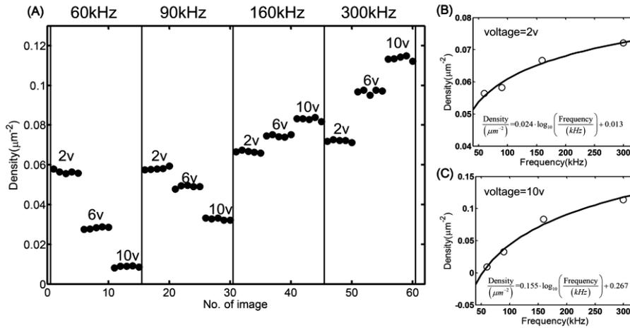
**Figure 1. (A) Particle density of self-assembly system as function of frequency and voltage; (B) Empirical model for particle density as function of frequency at a constant voltage of 2V; (C) Empirical model for particle density as function of frequency at a constant voltage of 10V.**
