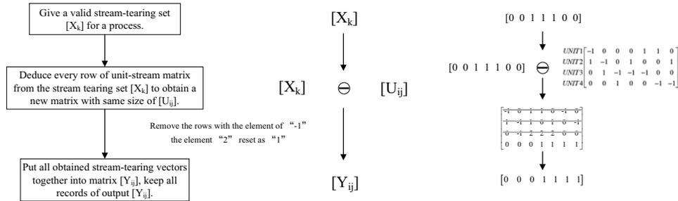
Figure 2 The schematic for logical loop matrix minus and an example
