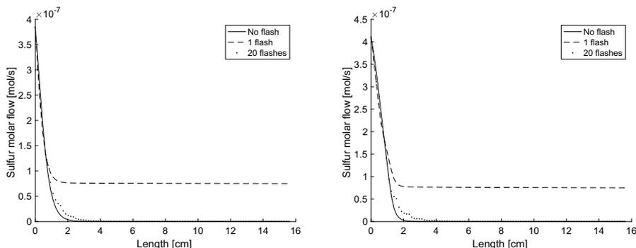
Figure 3 Molar flow profile of sulfur compounds with or without flashes. The plots present the feed with 75 wt.-% (left) and 25 wt.-% methylated substrate (right).
