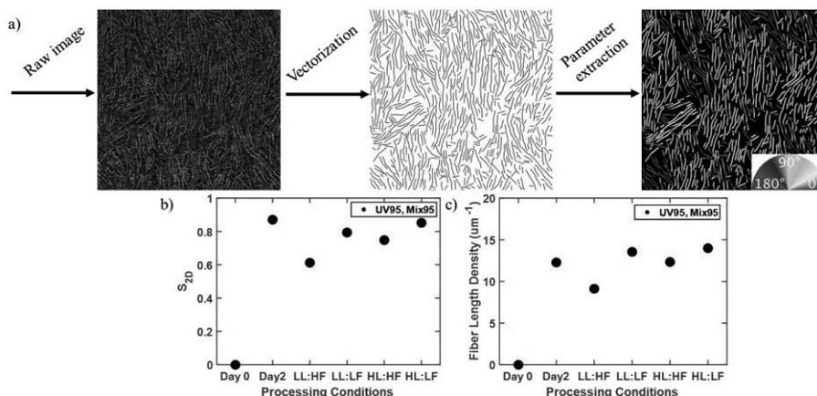
**Figure 3.** (a) Example of vectorization of P3HT fibers into quantifiable format using LL:LF sample. The image on the far right is referred to as an orientation map (b)  $S_{2D}$  orientational order parameter and (c) fiber length density values for batch and continuous flow processing.
