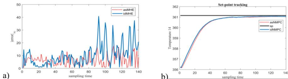
Figure 4 NMPC-MHE Results for Distillation Column; a) absolute error for MHE, b) Set-point tracking profile in NMPC
