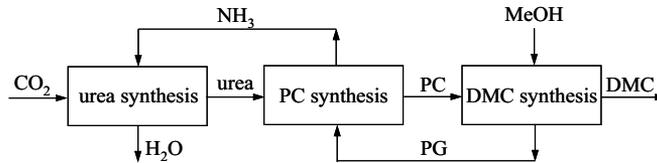
Figure 1. Concept of DMC production by indirect alcoholysis of urea.
