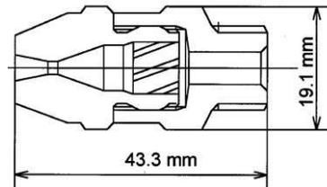
Figure 1: Hollow-cone spray nozzle
