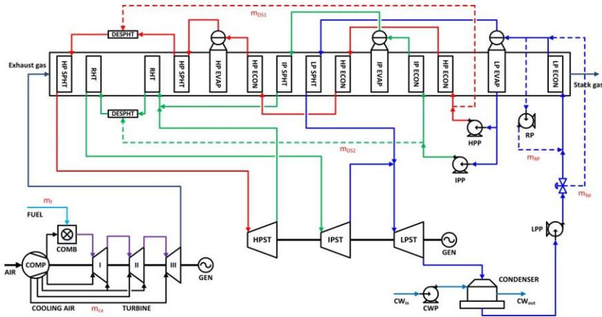
Figure 1 Schematic of a triple-pressure reheat combined cycle power plant.
