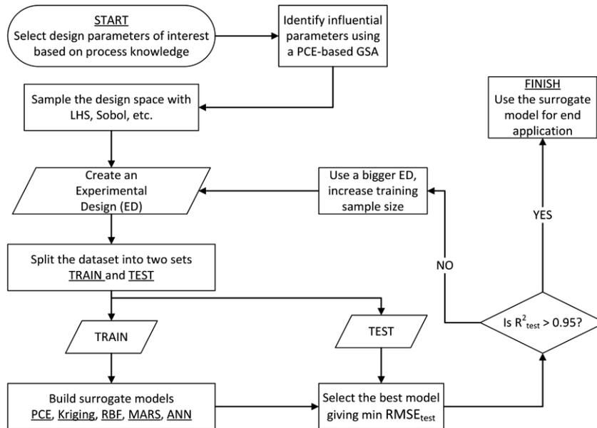
Figure 1: Systematic framework for developing surrogate models to be used in WWTP modeling the BSM1 model is simulated for 150 days using the dry weather influent file. Model outputs of interest included effluent quality indices, such as COD, TSS, TN, and SNH.
