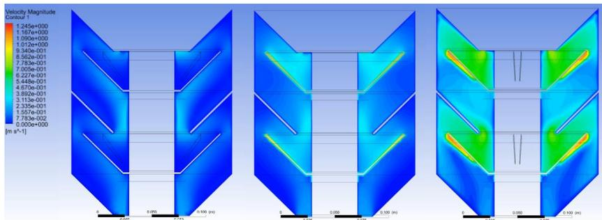
Figure 3. Vapor velocity (left: 0rpm, center: no fin/170rpm, right: fin/170rpm)
