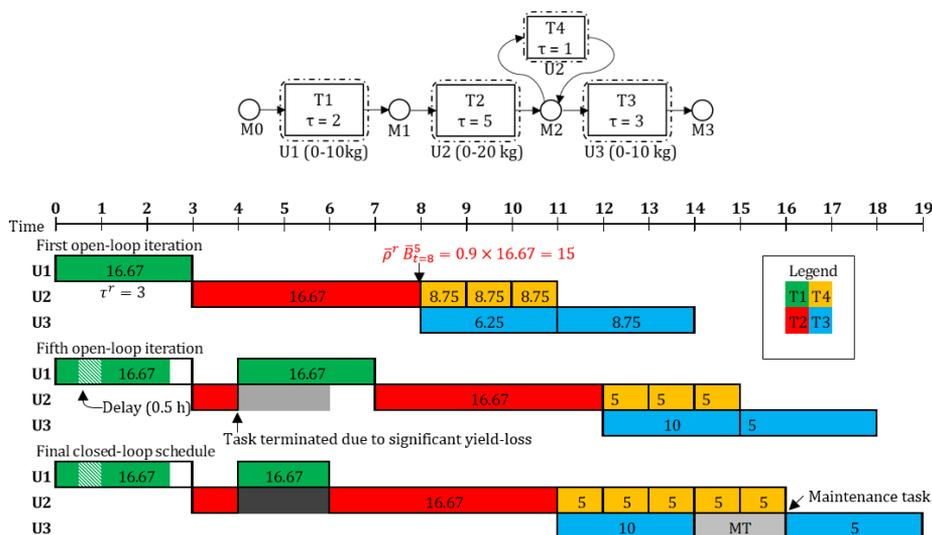
Figure 2: The network, the first and fifth open-loop iterations, and the final closed-loop schedule.
