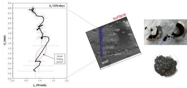
Figure 6. Model-based diagnosis of layering of deposit in a 4 years of operation in a refinery heat exchanger a) matched well with experimental composition analysis of the deposit b).
