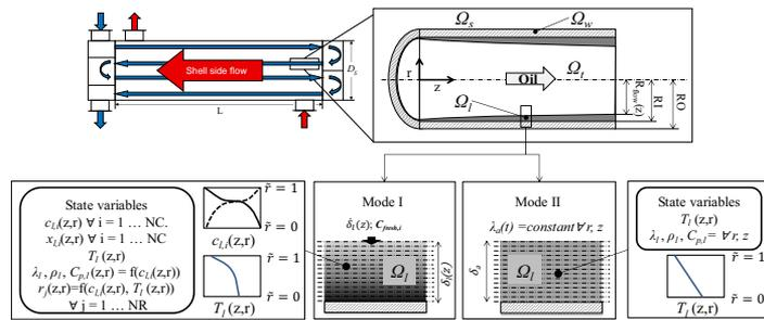
Figure 1. Schematic representation of exchanger modelling framework
