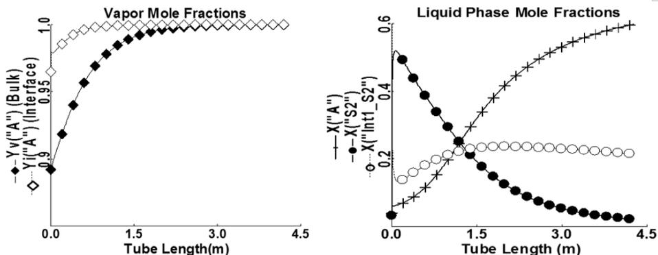
Figure 2. Consistent negative condensing flux of A and liquid profiles of S2 and Int1\_S2.
