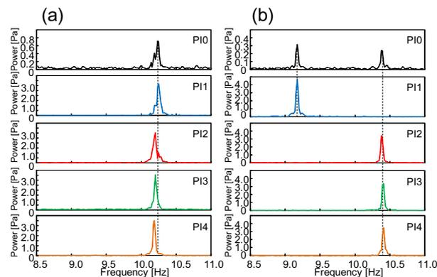
Figure 7 Fourier transform of data acquired from PI1 to PI4: (a) normal and (b) abnormal conditions
