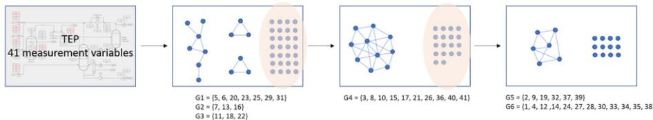
Figure 2. Performing iterative graphical lasso on 41 TEP variables
