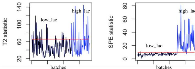
Figure 3. PCA monitoring results. a) in principal space b) in residual space
