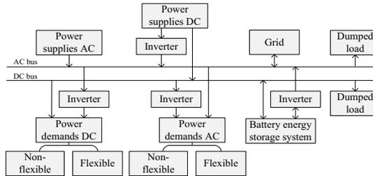
Figure 1 A schematic diagram of an HPS
