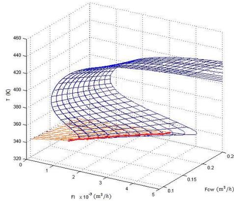
Figure 2. Zone classification of Phase Behavior for space surface of T- $F_I$ - $F_{CW}$ .
