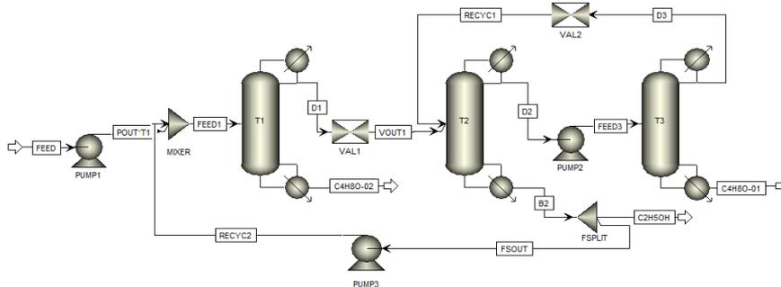
Fig. 5 PSD configuration for the ternary mixture separation
