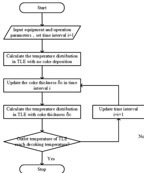
Figure 2. The algorithm diagram of the integrated model.
