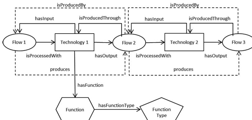
Figure 1. A representative pathway of the developed ontology and the defined object properties (relations). Different shapes correspond to different classes.
