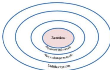
Figure 1. Onion diagram for process design.
