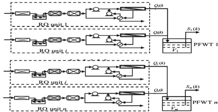
Fig. 1. Schematic diagram of a large-scale SWRO desalination plant
