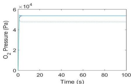
Figure 3. Partial pressures in the anode.  $O_2$  solid line.  $H_2O$  dotted line.  $j_{el} = [0.02, 0.1, 1]$   $Acm^{-2}$  (darker to lighter).
