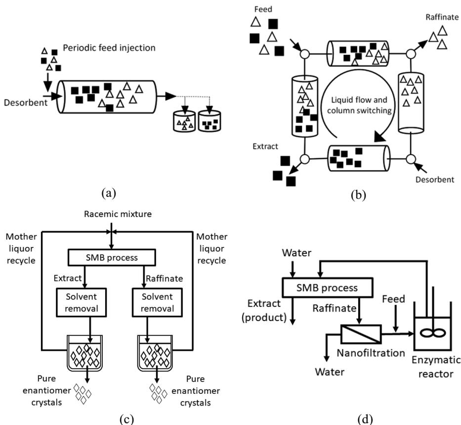
Figure 2 Chromatography processes; (a) single-column batch chromatography, (b) simulated moving bed (SMB) process, (c) integration with crystallizers for enantiomer purification (Kaspereit, et al. 2005), (d) integration with membrane and enzymatic reactor (Bechtold, et al. 2006)
