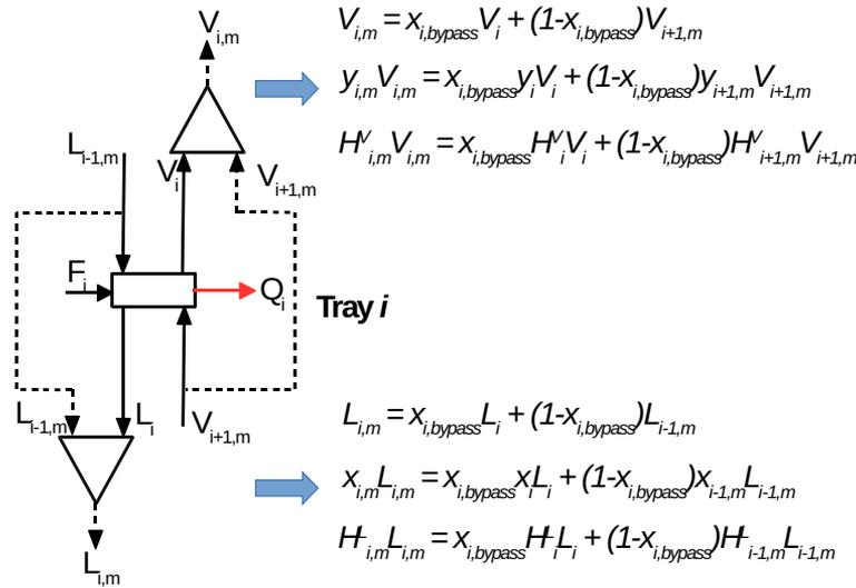
Figure 1: NLP framework with bypass streams
