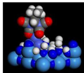
Figure 2: Optimized geometry for CCTBA adsorption on a Co<sub>4</sub> cluster with Ta<sub>3</sub>N<sub>5</sub> terrace. Periodic boundary conditions are not shown for clarity.
