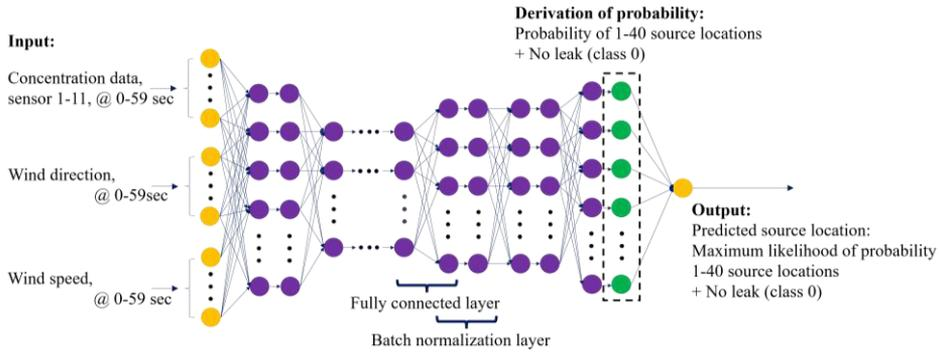
Fig. 4 Feed-forward neural network using 60-second time series data.
