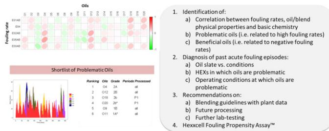
Figure 7. Model-based statistical analysis of large operational data sets identifies which crude oils are problematic, in which parts of the network, and in which operating conditions.
