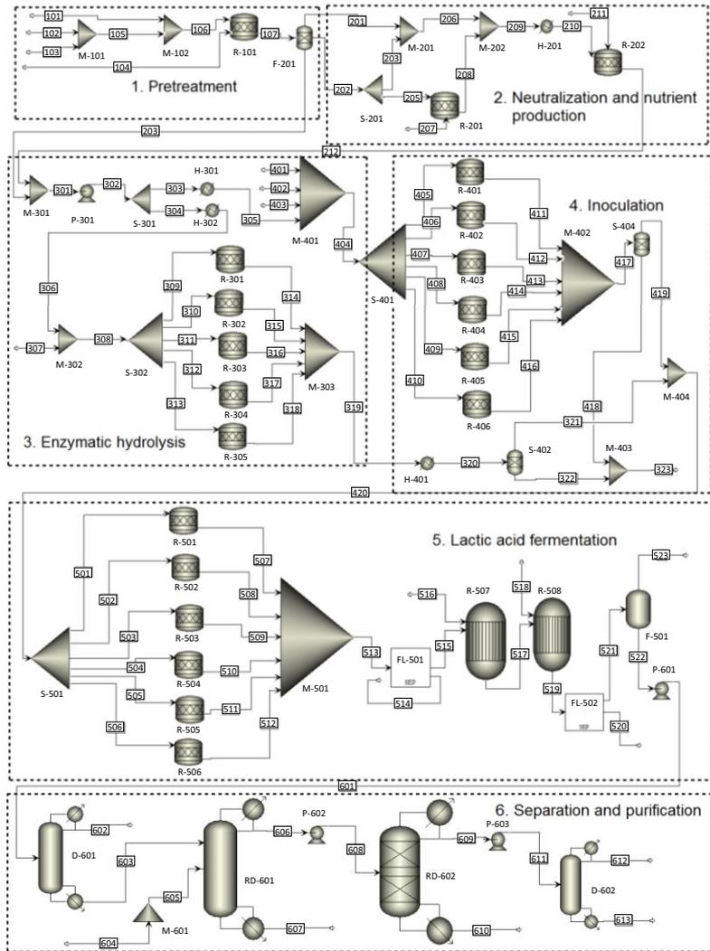
Figure 1. Process flowsheet for the acid lactic production
