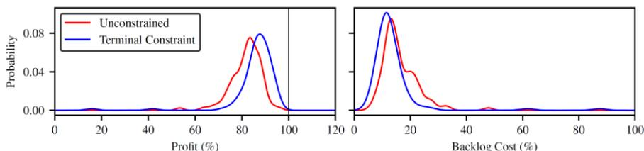
Figure 2: Kernel density estimate for closed-loop profit and backlog cost based on 100 simulations. Values normalized to profit of optimal  $T = 48$  periodic solution.
