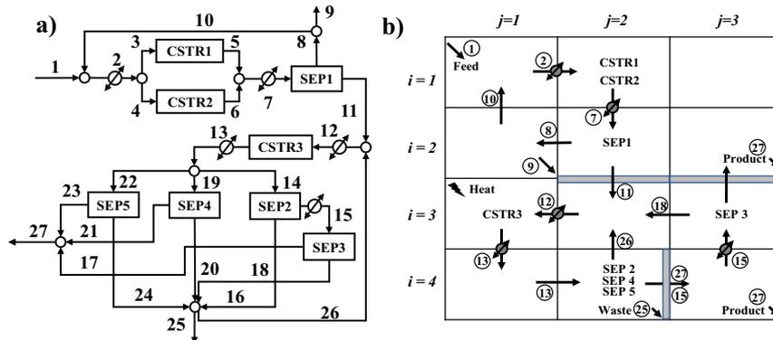
Figure 2. Superstructure representations (a) unit-operation based, (b) block based.
