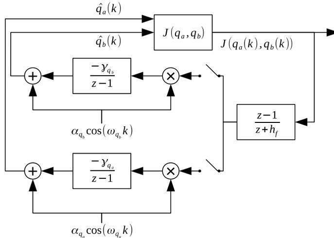
Figure 2 – Proposed Extremum-Seeking Control structure
