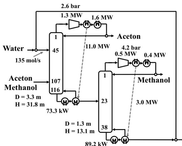
Figure 5 Optimal design of the VRC water process
