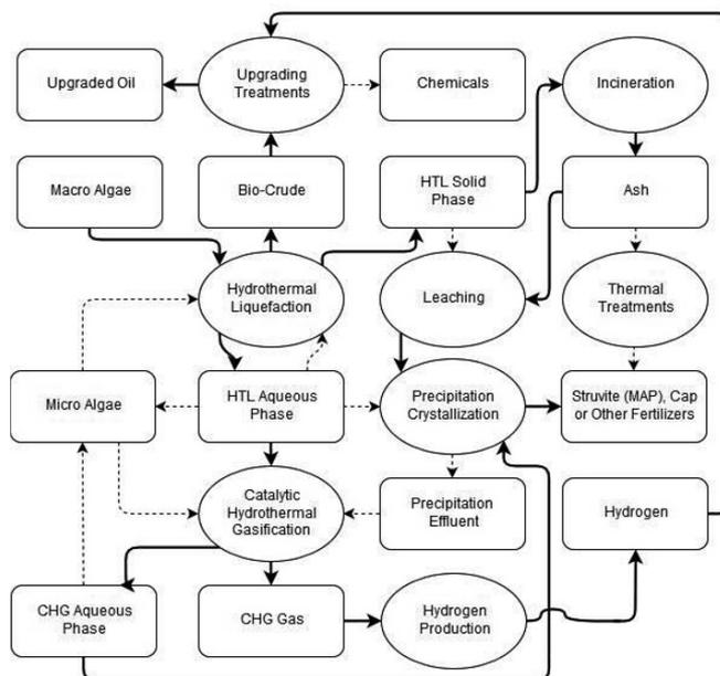
Figure 1: P-recovery for macroalgae HTL superstructure. Ovals and rectangles represent respectively sub-processes and materials. Bold arrows represent the pathway chosen in this work.
