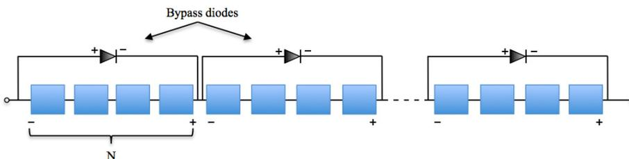
Figure (1): Schematic diagram showing the system's configuration.
