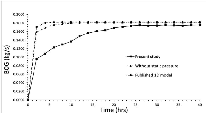
Figure 1. Boil-off-gas (BOG) generation rate in a full-scale LNG storage tank.
