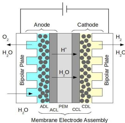
Figure 1. PEMEC diagram
