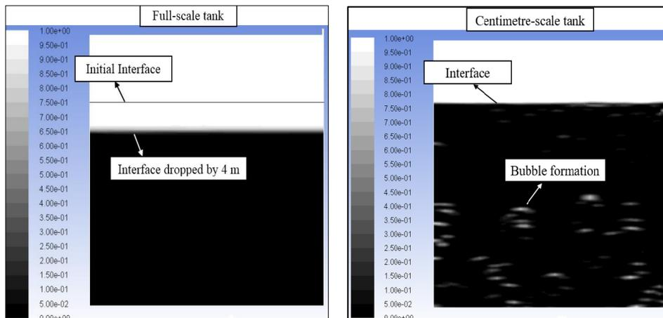
Figure 3. Phase contours for full-scale and centimetre-scale tanks at  $U = 2.5 \text{ W/m}^2\text{K}$ .
