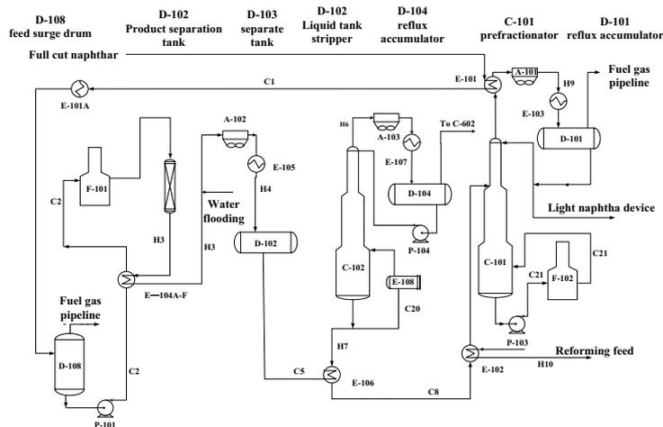
Figure 1. The pretreatment process of CRR unit
