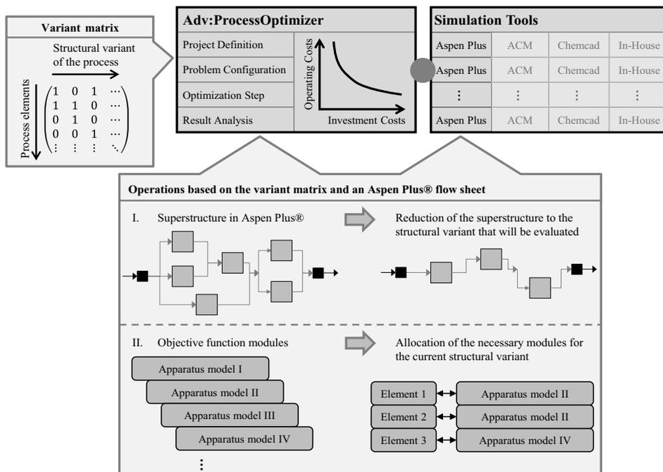
Figure 1: Schematic illustration of the system architecture of the Advanced Process Optimizer for the structural and parameter optimization of chemical production processes, adjusted considering Ernst et al. (2017). Explanatory remarks are given to the most important and new components.
