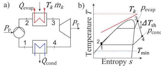
Figure 3: ORC process in (a) flowsheet and (b) qualitative temperature-entropy diagram.
