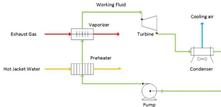
Figure 1: Schematic diagram of the ORC pilot plant
