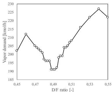
Figure 5: Correlation of minimum vapor demand and D/F ratio in the RD
