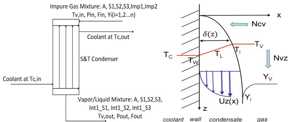
Figure 1. Configurations of a vertical shell-and-tube exchanger and liquid film in tube.
