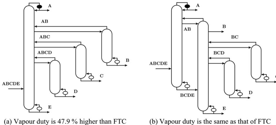
Figure 1: Candidate configurations for the separation of alcohols: (a) Optimal sharp-split configuration (b) Optimal configuration with one sloppy split
