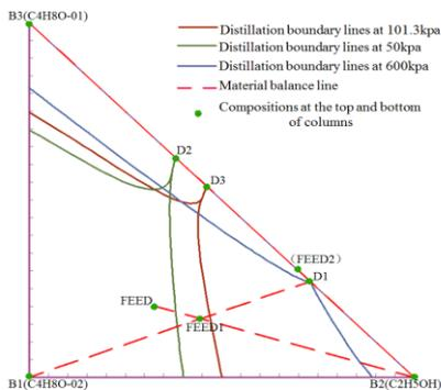
Fig. 4 Distillation boundaries at different operating pressures
