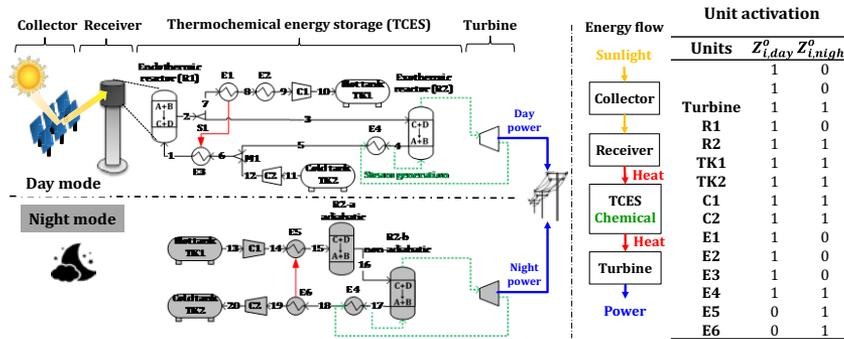
Figure 5. Process flow sheet of CSP plants with fluid phase TCES systems.
