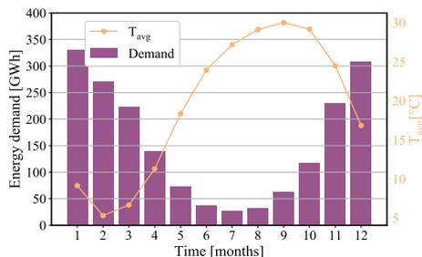
Figure 5. Average temperature in the ground and heating (SH and DHW) demand
