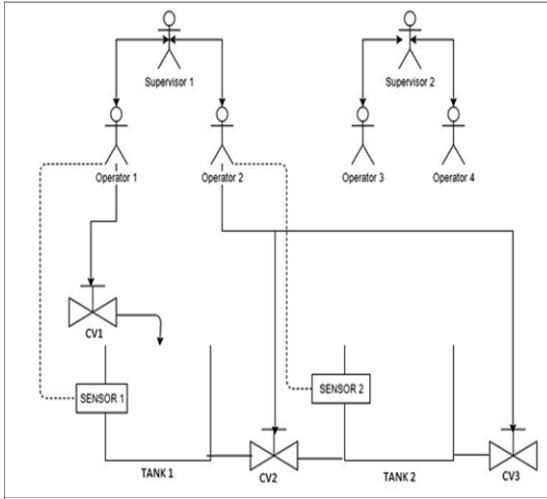
Figure 2. Two tank interacting system hierarchy
