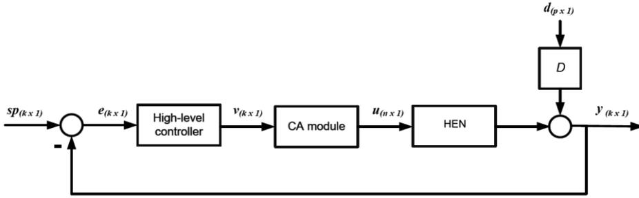
Figure 1: CA-based control structure
