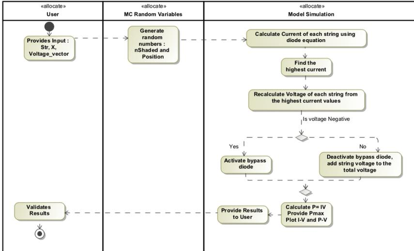
Figure (2): Simulation Algorithm Activity Diagram. Note that “Str” is the number of strings.
