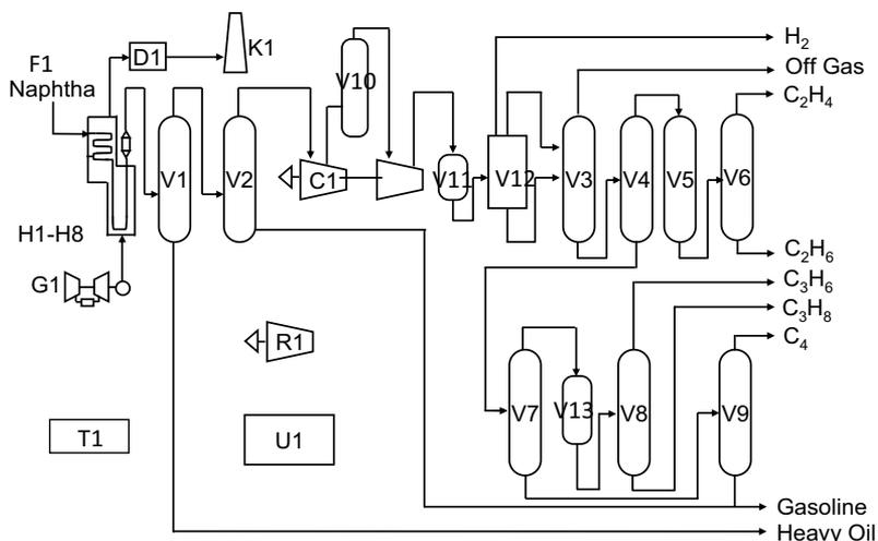
Fig. 4 Process flow diagram for ethylene plant (Higuchi *et al.*, 2010)
