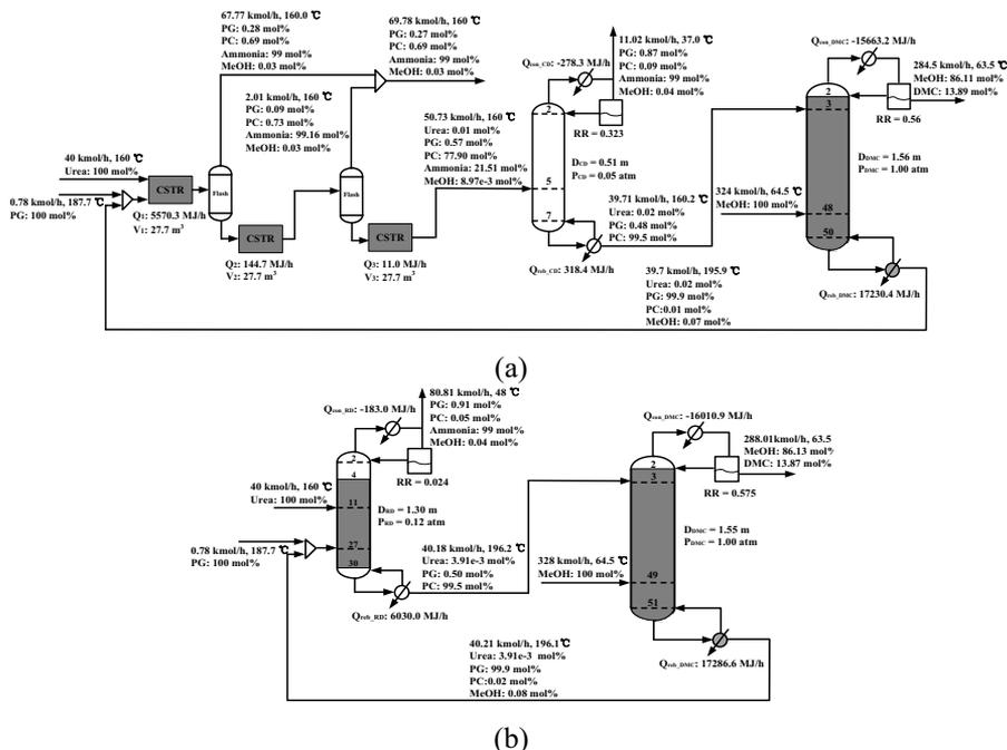
Figure 3. Optimal design for (a) CSTR+CD and (b) RD configurations.
