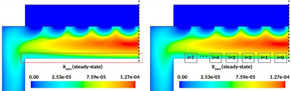
Figure 3. (left) Steady-state  $SiH_3$  concentration within PECVD reactor. (right) Defined reactor zones which contain independent EWMA control algorithms.
