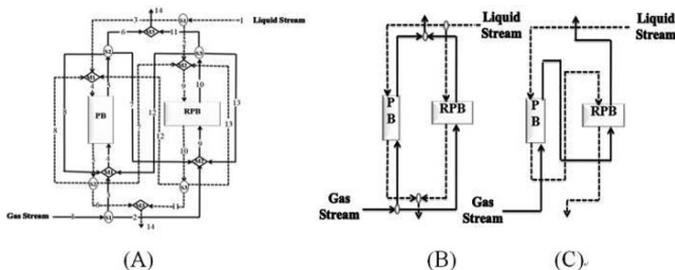
Fig. 3 Superstructure of the integrated RPB and PB processes: (A) overall structure; (B) in parallel configuration; (C) in series configuration. S denotes a splitter and M denotes a mixer, respectively. Gas streams are denoted by solid lines; liquid streams, by dashed lines.
