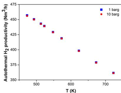
**Figure 2.**  $H_2$  productivity under autothermal conditions (range of  $CH_3OH$  required for autothermal operation:  $\sim 20\text{-}60 \text{ Nm}^3/\text{h}$ )
