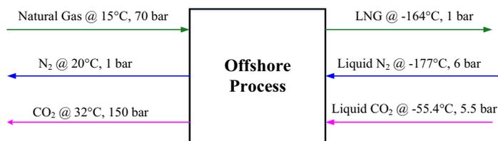
Figure 1 WHENs problem in an offshore LNG process (Aspelund and Gundersen, 2009)
