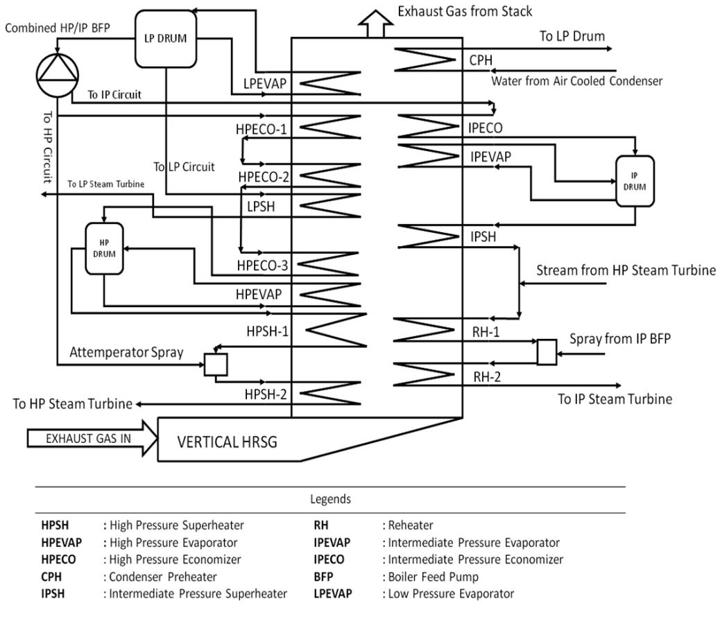
Figure 2. Vertical triple pressure HRSG under consideration
