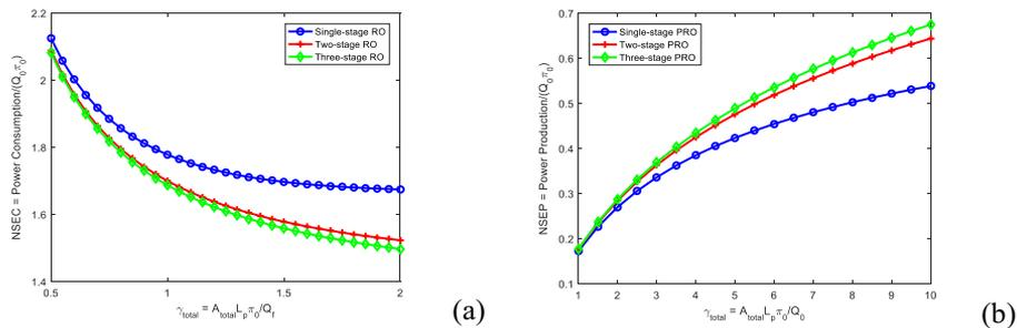
Fig. 2 Effects of total dimensionless membrane area  $\gamma_{total}$  and number of stages on (a) NSEC in RO at 40% recovery (Li, 2011) and (b) NSEP in PRO (Li, 2018).
