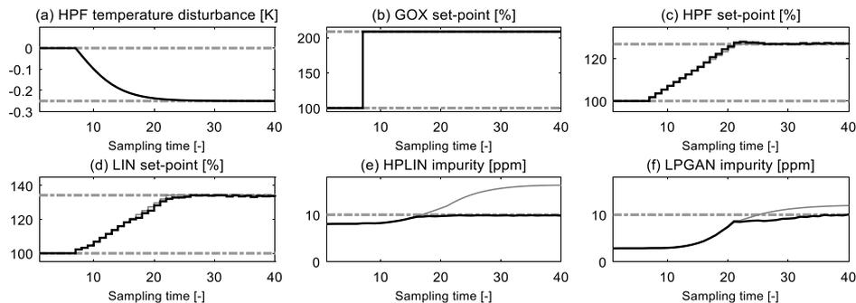
Figure 5: Temporal course of relevant process variables for a change of product mix of the ASU considering disturbances. Solid black lines show the simulation using the two-layer APCS. Thin grey lines show the results without tracking control. Dashed-dotted grey lines show constraints.
