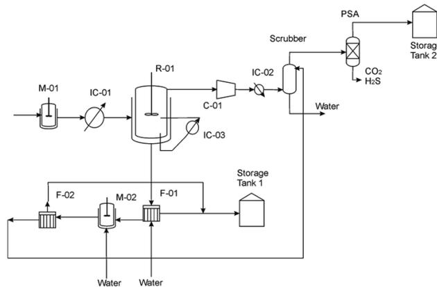
Figure 1.- Scheme of a one digester process for waste to power.
