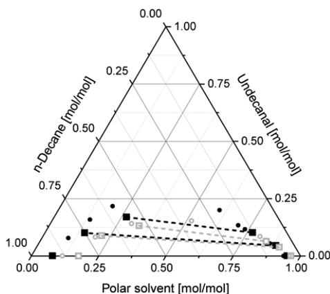
Figure 2. LLE (■) and cloud point measurements (●) for decane, undecanal, and DMS and LLE (□) and cloud point measurements (○) for decane, undecanal, and THPO at 25 °C. The molecular structures for both solvents are shown on the left.
