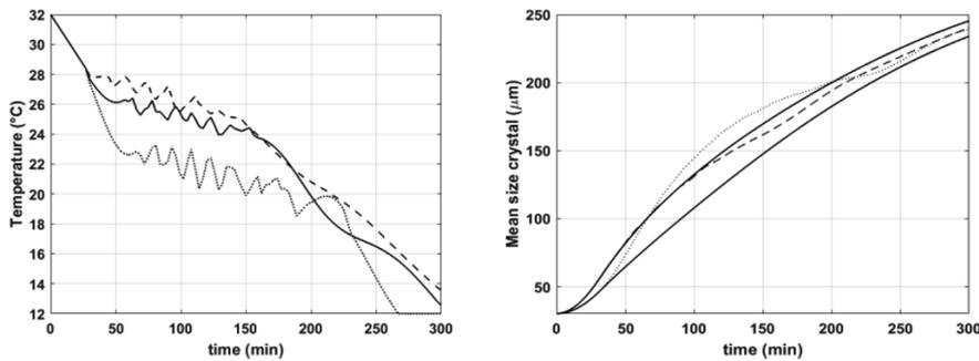
Figure 3- Temperature profiles (left) in closed loop for uncertainty in crystal growth (dashed: +20%, dotted: -20%, full: no disturbances) and the mean size evolution of crystals (right) under disturbance when in open-loop and closed loop (full: open loop for +20% and -20%, dashed:+20%, dotted: -20%,).
