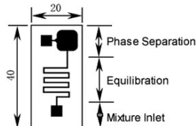
Figure 3. Distillation device consisting of phase separation and equilibration sections (Sotowa et al., 2003)
