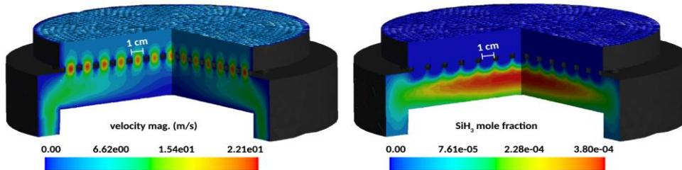
Figure 3. (left) Velocity magnitude within 3D PECVD reactor showing dead-zone near substrate center. (right) Non-uniform, steady-state SiH<sub>3</sub> concentration.
