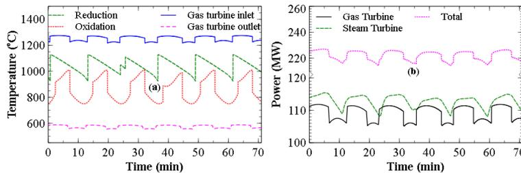
Figure 3. (a) Temperature profiles of the gas streams; (b) dynamic power performance.
