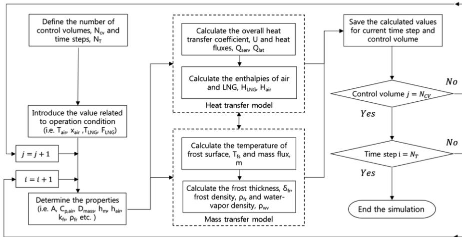
Figure 1. Flowchart of the vaporizer model
