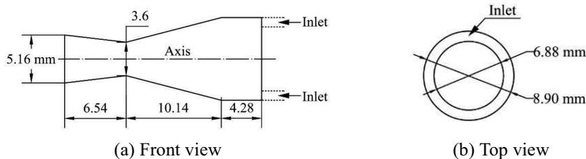
Figure 2: Equivalent model of the nozzle
