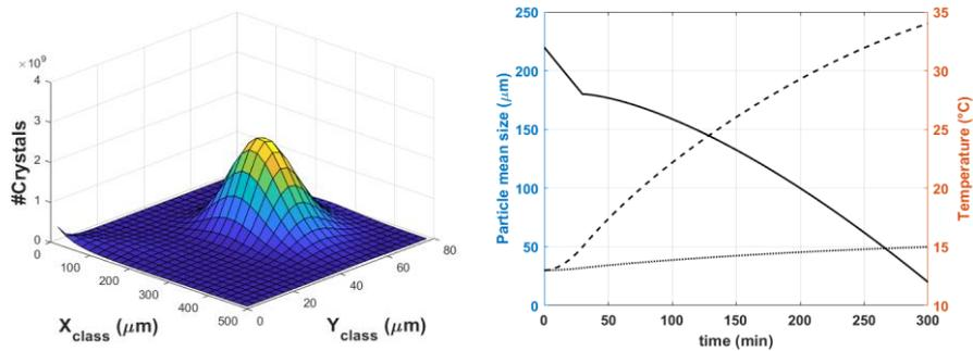
Figure 1- Final particle size distribution, at 5 hours of crystallization (left). Dynamic temperature profile over the process (full line, right), and the evolution of the mean sizes (dashed, right).
