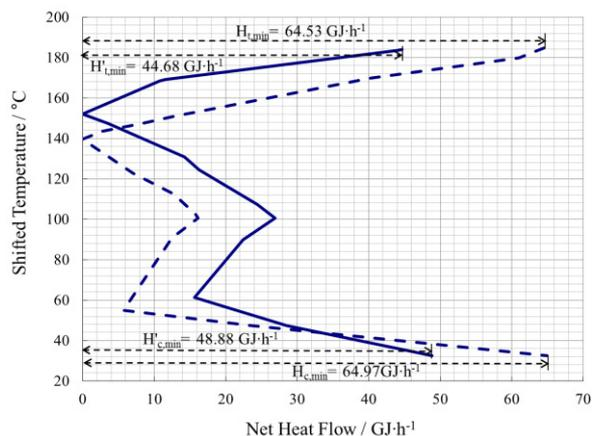
Fig.3. Grand composite curves of the existing and optimal process
