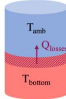
Figure 2. Schematics of stratified geothermal model
