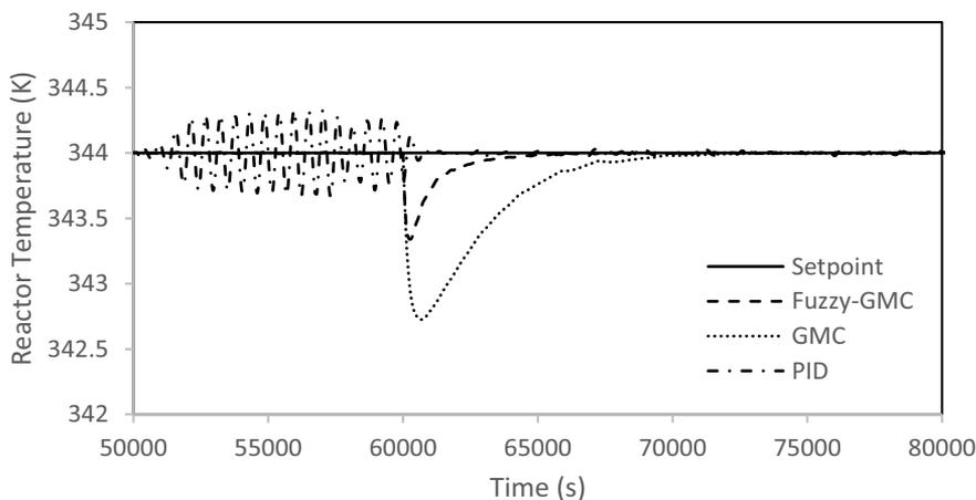
FIGURE 4. Controllers' performance in disturbance rejection.
