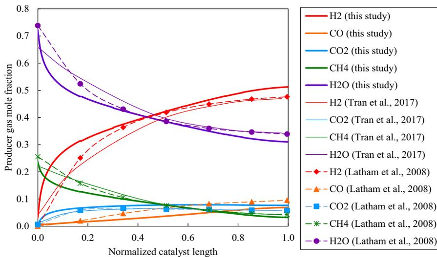
Fig. 3. Comparison of product gas composition along catalyst length with literature
