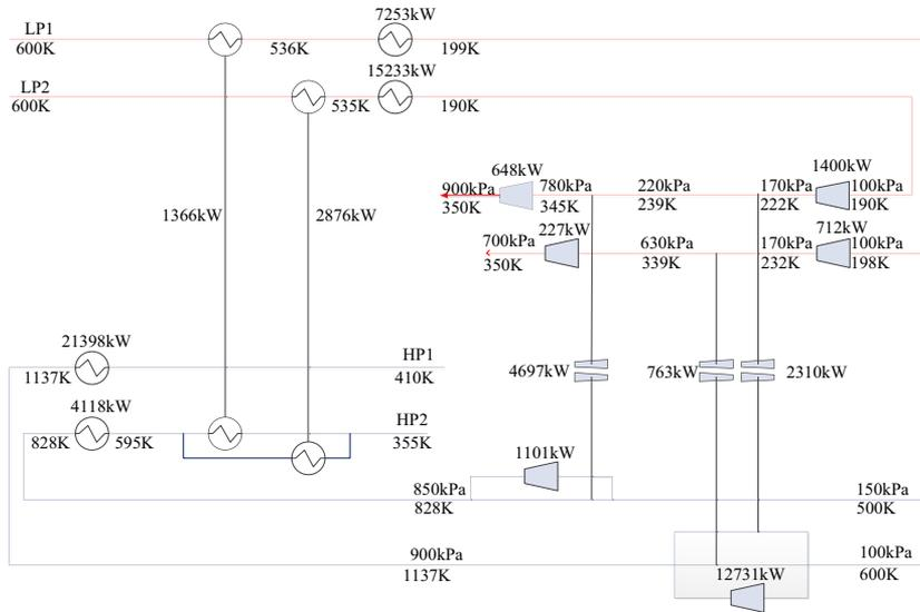
Figure 5 Optimal WHEN configuration for Case A
