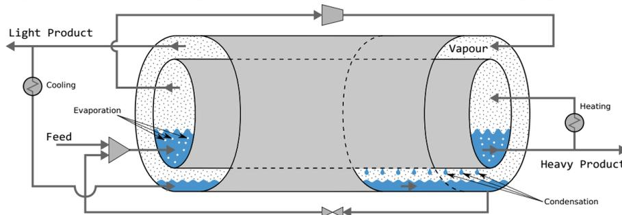
Figure 1. The heat integrated distillation system. The stripper is represented by the inner chamber and the rectifier is represented by the outer chamber. Dimensions: Length = 2 m, stripper diameter = 1.8 m and rectifier diameter = 2 m.
