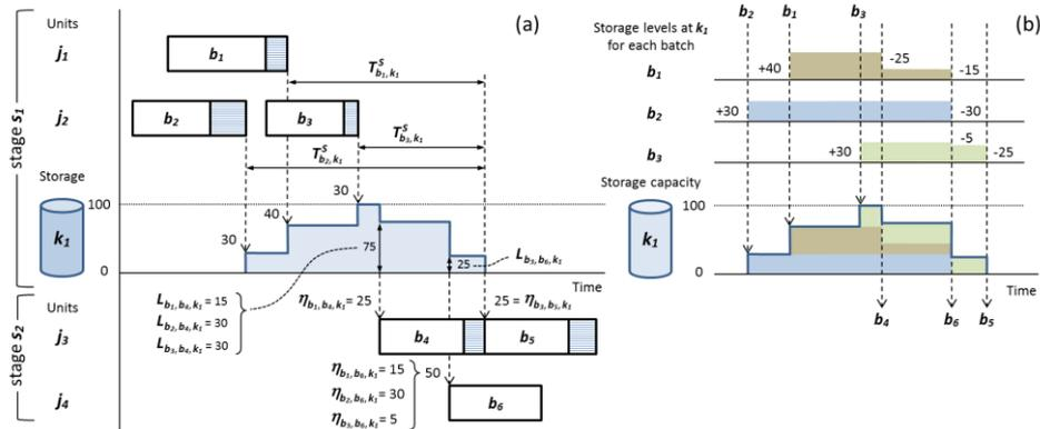
Figure 1: (a) Illustrative schedule considering multiple intermediate storage mixing and splitting operations; (b) Individual storage levels for each batch at  $k_1$ .
