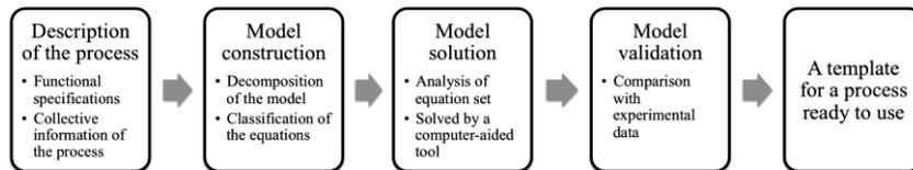
Figure 2. Workflow for the creation and use of a process template.
