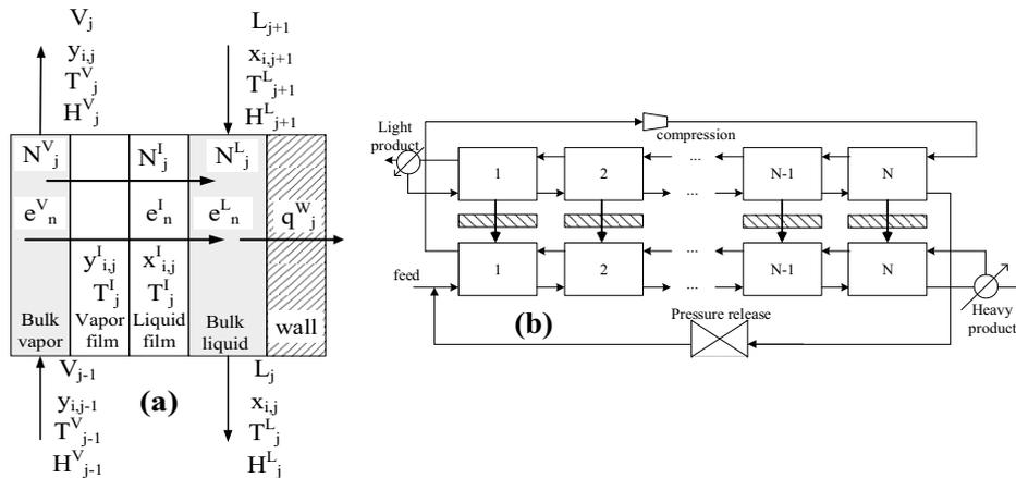
Figure 2. Model representation. (a) Single segment  $j$  and (b) integration of the  $N$  segments, together with compression and expansion.
