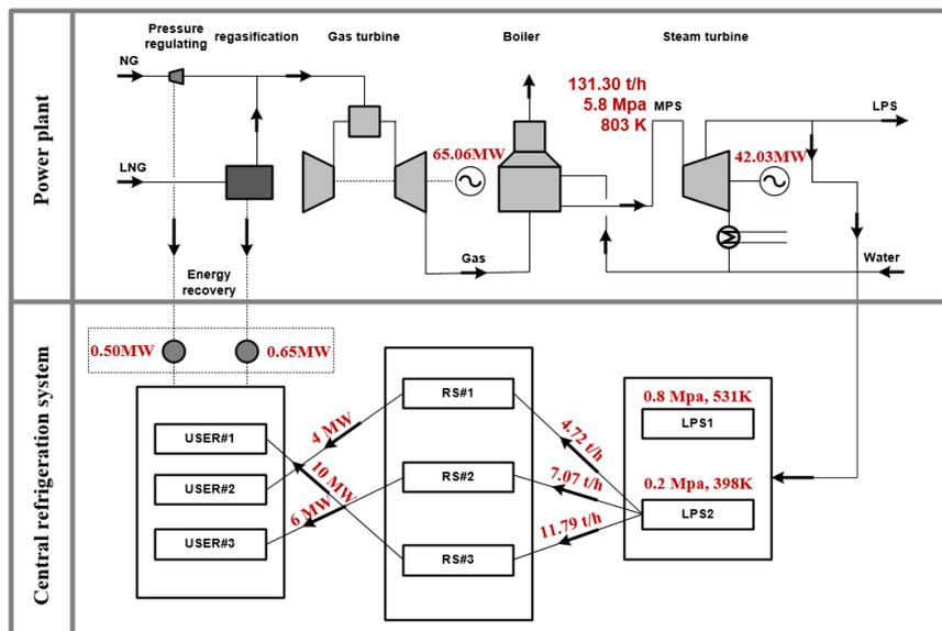
Figure 2. The optimal flowsheet and heat load of CRS
