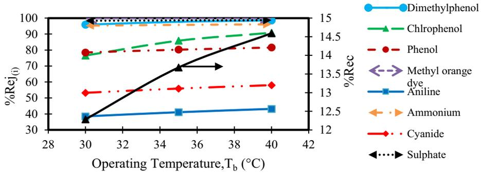
Fig. 4. Effect of operating temperature on rejection and recovery rate (operating conditions:  $2.583E-4$  m<sup>3</sup>/s, 10 atm, 350 ppm)
