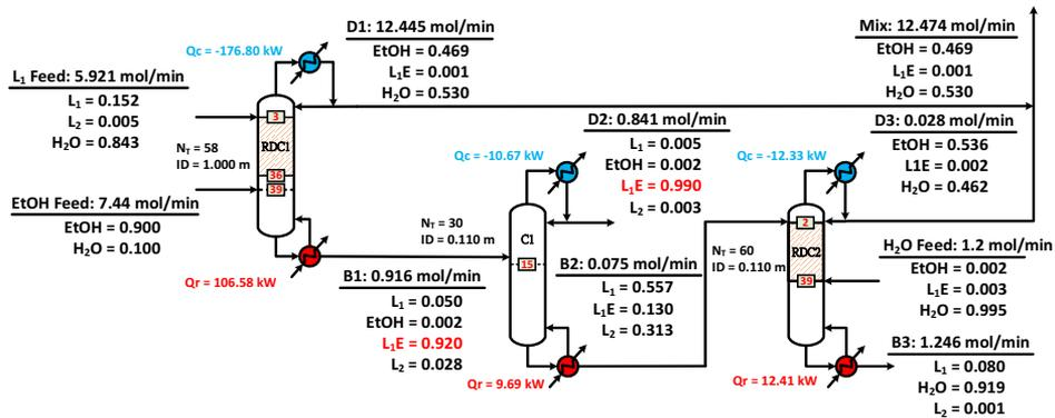
Figure 1. The simulation results from the process concept of Miller et al. (2010)
