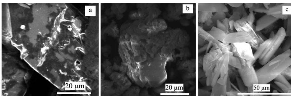
Figure 4. SEM images of selected samples: a. Direct crystallization of CaP from digester supernatant (Vasenko and Qu, 2017 c); b. Fast precipitation/recrystallization technology; c. Novel hybrid technology.
