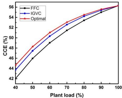
Figure 7 CCE versus plant load under FFC, IGVC, and optimal strategy.
