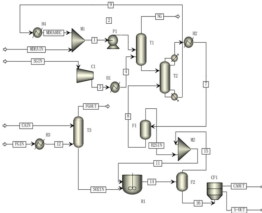
Figure 1 Novel wet Claus sulfur recovery process flowsheet
