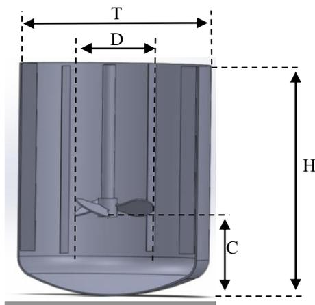
Figure 1. Pilot scale crystallizer.
