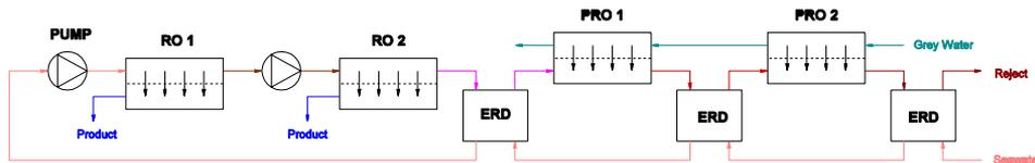
Fig. 3 Schematic of a hybrid two-stage RO-PRO process for energy-efficient seawater desalination.
