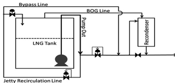
Figure 5. Flow scheme for recirculation and send out flow
