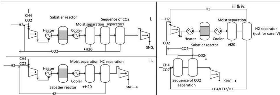
Figure 2. The four process configurations.
