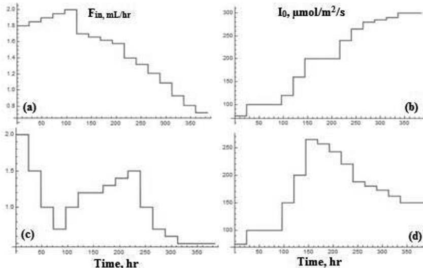
Figure 1: Optimal control actions under different scenarios. (a) and (b), (c) and (d): nitrate inflow rate and light intensity in the optimistic and pessimistic case, respectively.
