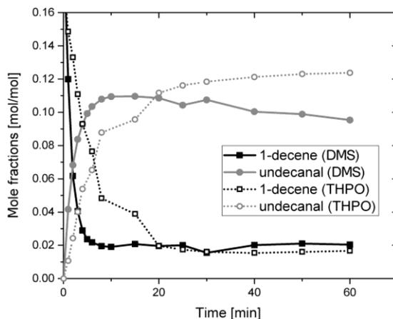
Figure 3. Mole fractions of 1-decene and undecanal during the reaction. The reactions were carried out at 105°C and 19 bar with 1-decene/decane/polar solvent = 0.20/0.48/0.32 mass ratios, H<sub>2</sub>:CO = 1:1, catalyst/1-decene = 1:2000 for DMS, catalyst/1-decene = 1:6000 for THPO, and Rh/ligand = 1:5. All ratios given in mol/mol except for reactants and solvents.
