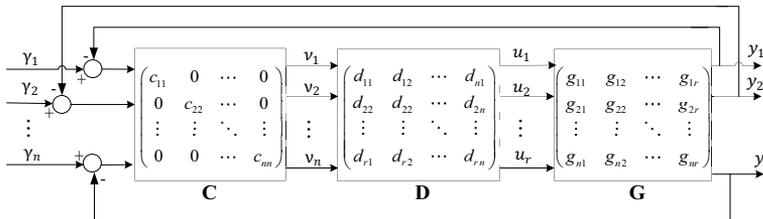
Figure 1. Decoupling control system for a  $n \times r$  multivariable process.
