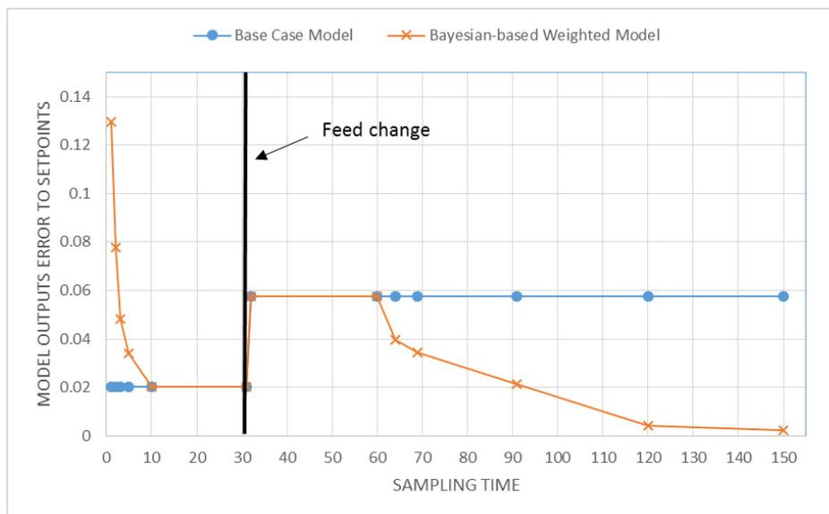
Figure 3. Model set-point error with feed change
