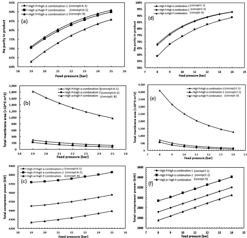
Figure 2. Helium purity in product, total membrane area, and required compressor power consumption in 4-stages/cross flow cascade membrane design concepts-A1, A-2 & B (a-c), and 4-stages/counter-current flow cascade membrane design concepts-C-1, C-2 & D (d-f).
