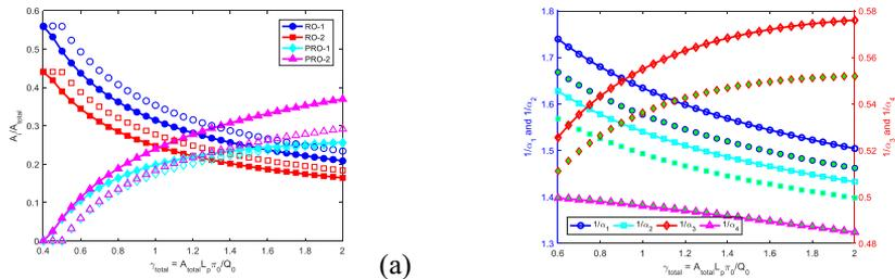
Fig. 5 Optimal (a) membrane area and (a) pressure among all membrane units in two-stage RO-PRO under different  $\eta_{PRO}$  (100%, solid symbols and 70%, hollow symbols) at 30% water recovery.
