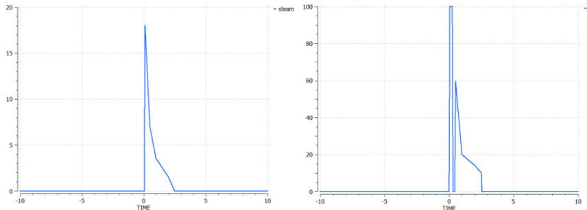
Figure 2. Profiles of the steam flow (left) and syrup demand (right) over the operation of a crystallizer approximated by piecewise linear segments at different time points  $tp(n)$
