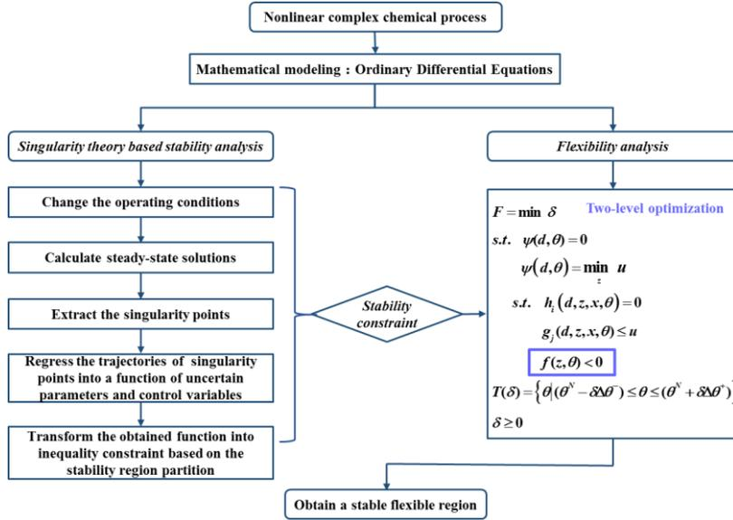
Figure 3. Flowchart of the novel method for integrating flexibility and stability
