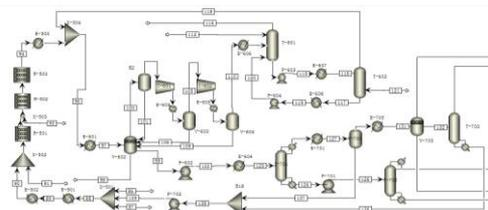
Figure 4 Flowsheet for an industrial process for the production of styrene through dehydrogenation of ethylbenzene drawn in Aspen plus.
