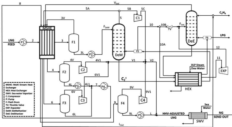
Figure 1: Proposed superstructure for the HHR process.
