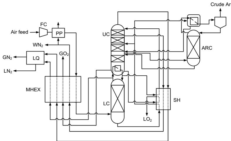
Figure 1: Industrial Air Separation Process Flowsheet.
