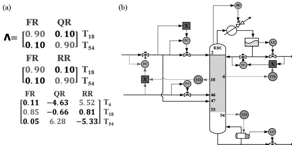
Figure 3: (a) RGA analysis results (b) The overall control scheme of CS3.
