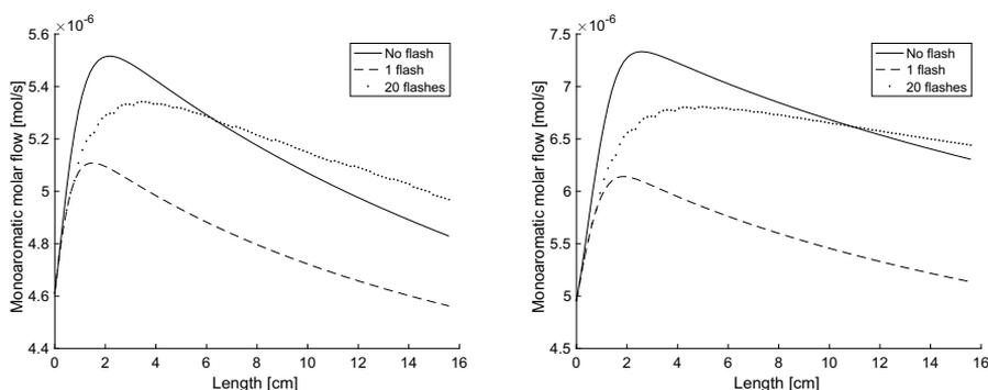
Figure 5 Molar flow profile of monoaromatics with or without flashes. The plots present the inlet with 75 wt.-% (left) and 25 wt.-% methylated inlet (right).
