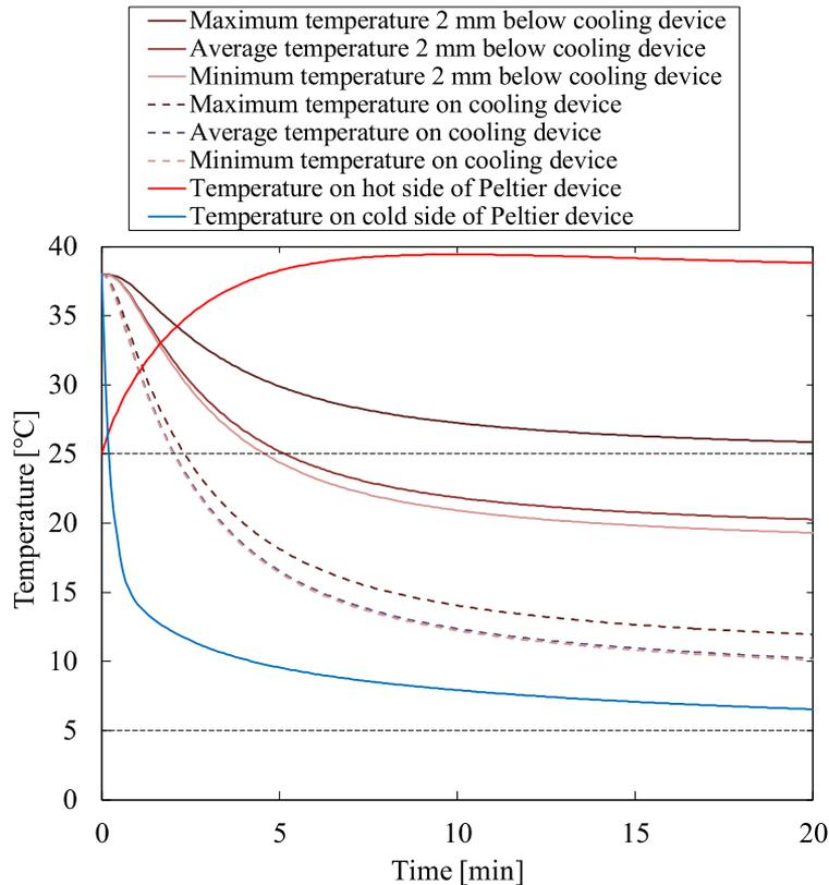
Figure 3. Temporal change of temperature in brain and Peltier device.
