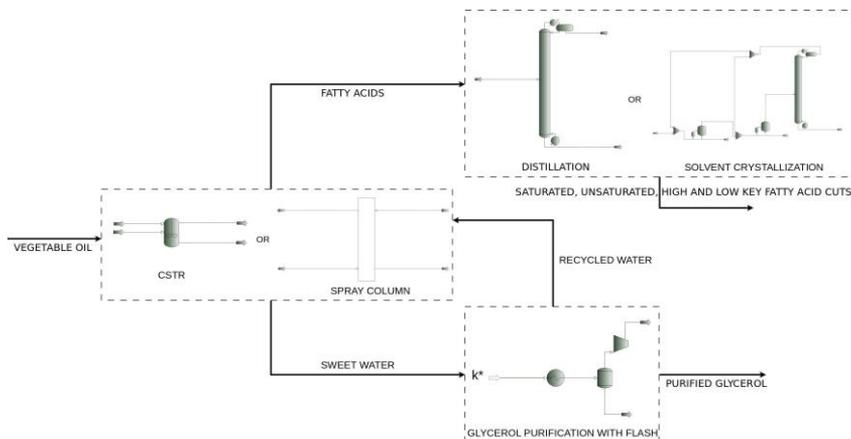
Figure 3: Schematic representation of possible process steps for the oleochemical process domain under research
