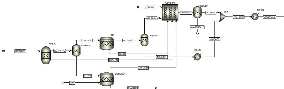
Figure 1. Biomass gasification model in Aspen Plus.
