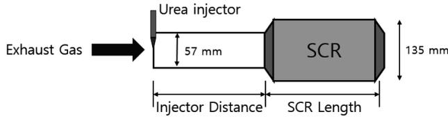
Figure 1. Configuration of SCR with urea injector (not in scale)
