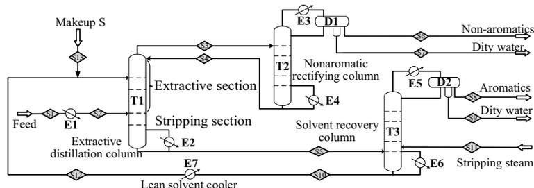
Fig. 1. Flowsheet of the sulfolane extractive distillation process
