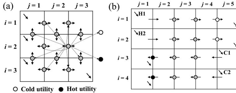
Figure 3. Heat exchanger network representation using block superstructure.
