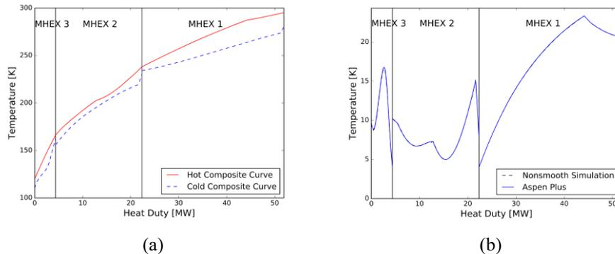
Figure 3: (a.) Composite curves for Case II. (b.) Corresponding driving force plot.
