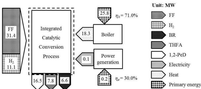
**Figure 3.** Energy flow diagram after heat integration
