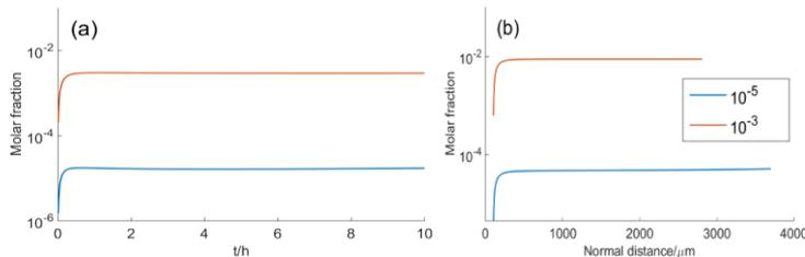
Figure 3 Crystal with different  $\text{KNO}_3/\text{NaNO}_3$  molar ratio. (a) Evolution of  $\text{KNO}_3$  molar fraction in the whole crystal (b)  $\text{KNO}_3$  molar fraction distribution in the normal direction of face  $\{104\}$
