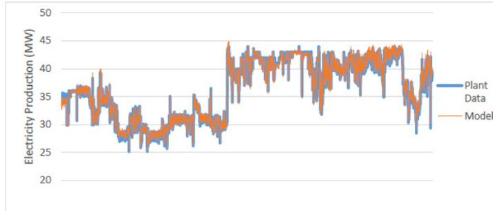
Fig.1 Comparison between the regression model and the plant data.
