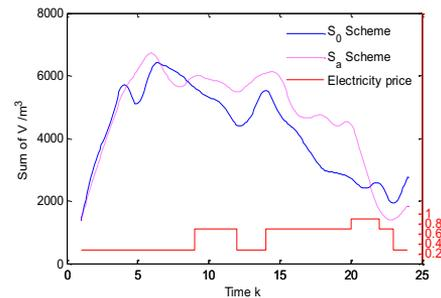
Figure 3: Comparison of total water volume with electricity price between  $S_0$  and  $S_a$
