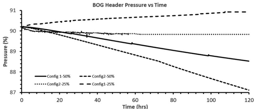
Figure 7. Pressure profile with variable compressor capacity
