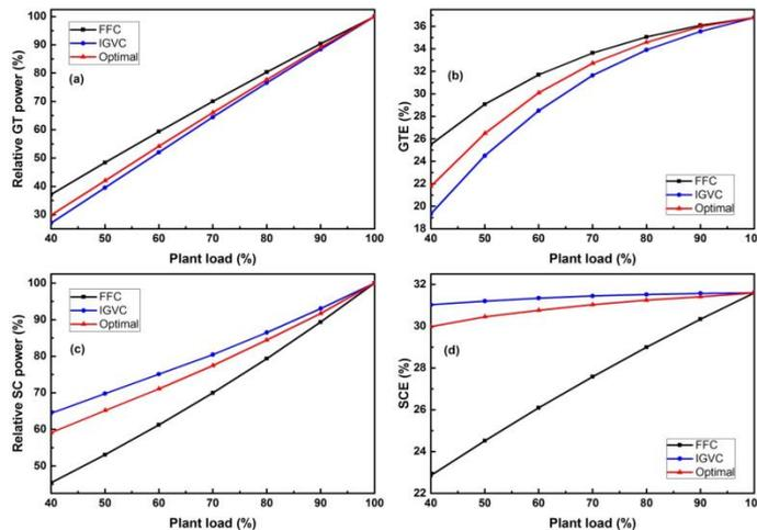
Figure 6 GT power, GTE, SC power, and SCE versus plant load under FFC, IGVC, and optimal strategy.
