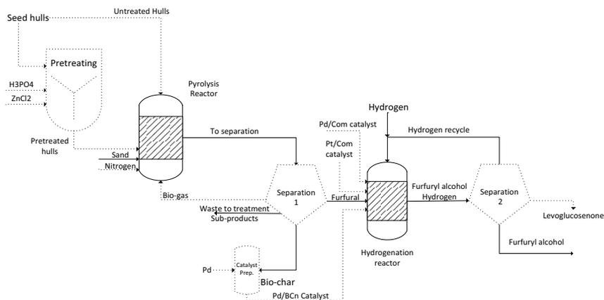
Figure 1: Simplified superstructure of the furfural and furfuryl alcohol production process. Equipment in dotted lines (together with associated streams) are represented by sets of logic propositions, each one represented by a Boolean variable. Separation sectors include several alternatives for the separation of products, being furfural, furfuryl alcohol and levogluosenone (if applicable) the desired products.
