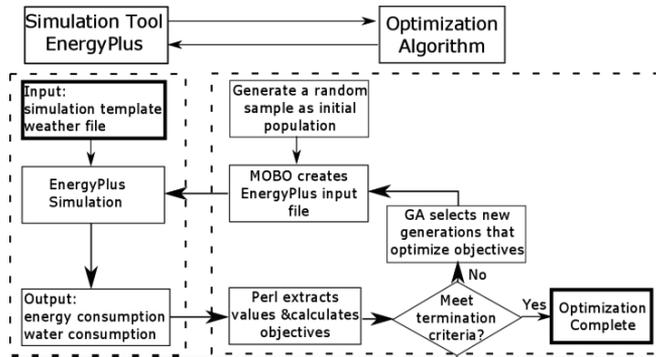
Figure 2: Simulation-based optimization flow chart
