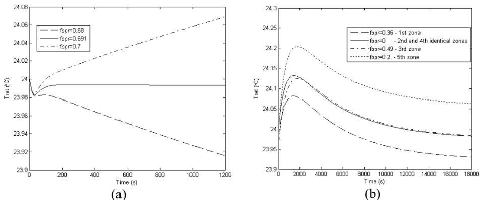
Figure 3: Response to perturbation in thermal load and bypass ratio
