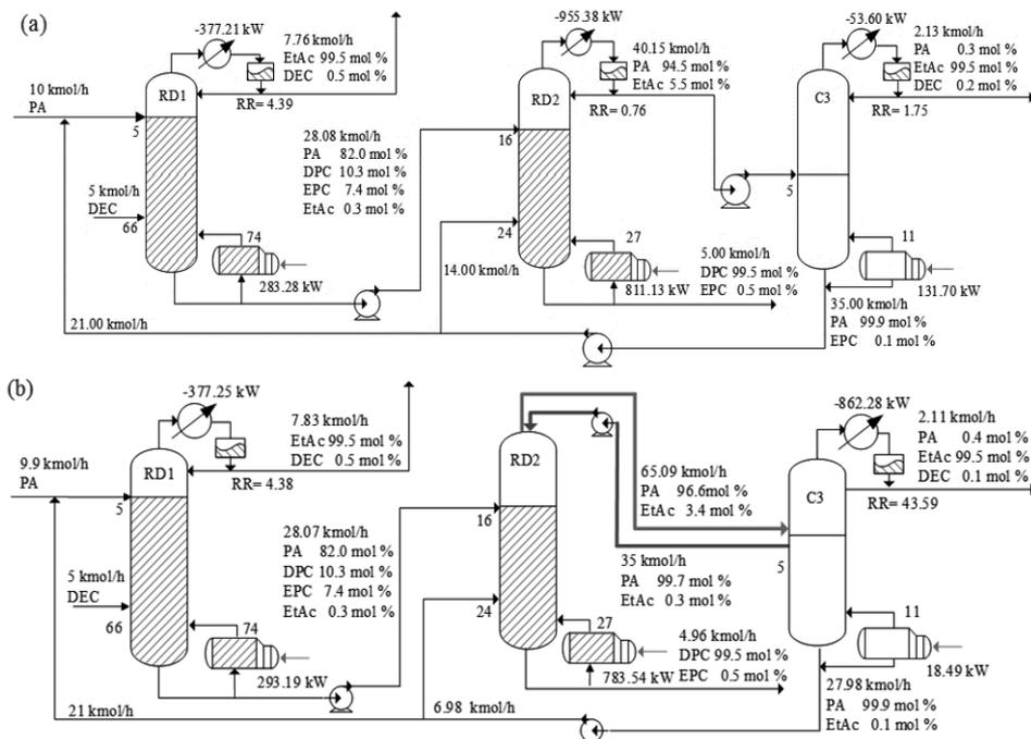
Figure 1: (a) Conventional RD configuration; (b) Thermally coupled design (Chen et al., 2015)
