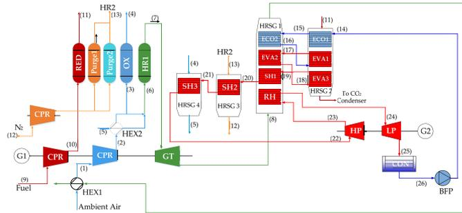
Figure 1. Diagram of the optimal CC power plant with fixed bed CLC reactors.
