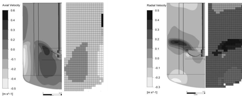
Figure 4. Characterization of the compartmental zone network via the auto zoning with 0.3 m/s tolerance of flow velocity: (left) axial direction, (right) radial direction.
