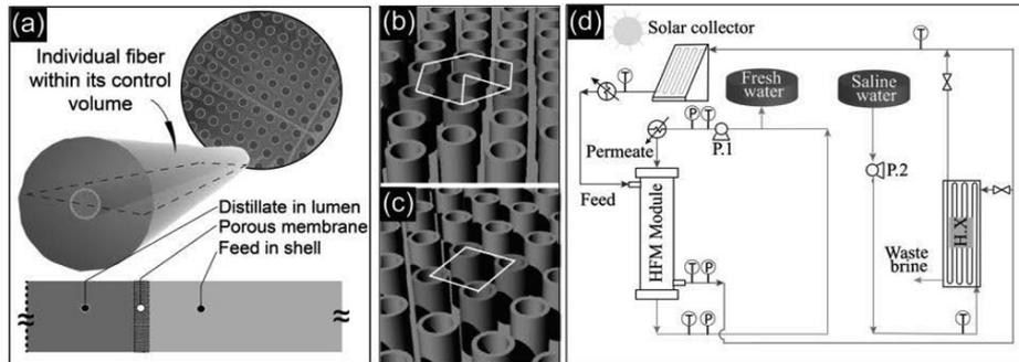
Figure 1. The schematic of the hollow fiber membrane module configuration and a lab-scale membrane distillation setup. (a) an individual fiber in its control volume (the cross-section representation is not to scale); (b) hollow fiber membranes in the close-packed configuration; (c) hollow fiber membranes in the square configuration; (d) the schematic of a lab-scale solar-assisted membrane distillation process.
