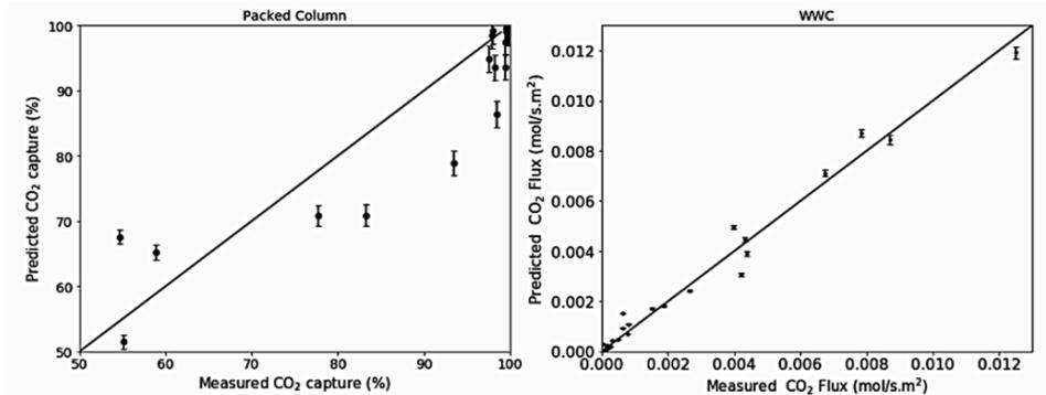
Figure 2: Parity Plots (a) Packed Column, (b) WWC
