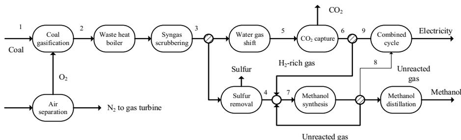
Figure 2. Schematic diagram of the methanol and power polygeneration process.
