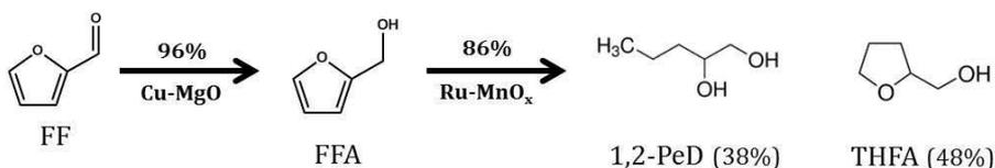
**Figure 1.** Reaction schematic view of FF-to-1,2-PeD and THFA
