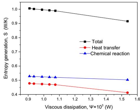
Figure 3: Variations of the entropy generation due to the chemical reaction and heat transfer, and the total entropy generation, with respect to the viscous dissipation
