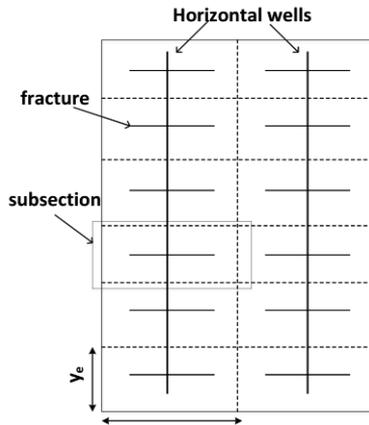
Figure 1. Illustration of a section for the case of two horizontal wells ( $n_c = 2$ ) and six fractures per well ( $n_r = 6$ ).
