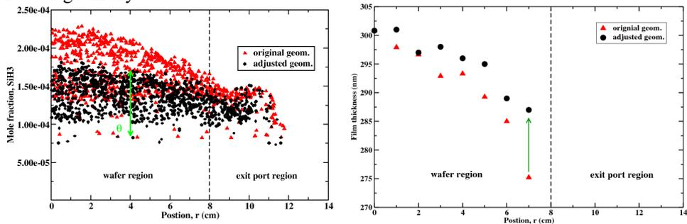
Figure 5. (left)  $\text{SiH}_3$  mole fraction as a function of radial position,  $r$ , and azimuthal position,  $\theta$ . (right) Radial  $\alpha$ -Si:H product thicknesses.
