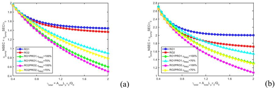
Fig. 4 Optimal NSEC in different membrane configurations under different  $\eta_{PRO}$  (70% and 100%) and different water recoveries  $Y_{total}$  (a) 30% and (b) 50%.
