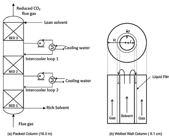
Figure 1: Packed Column and Wetted Wall Column
