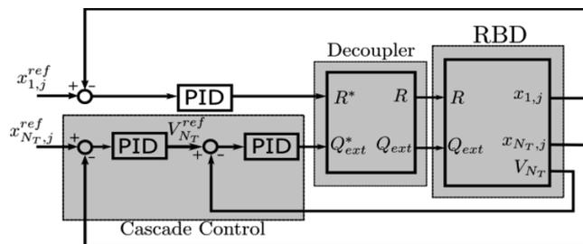
Figure 1: Cascade control structure with decouplers for the RBD
