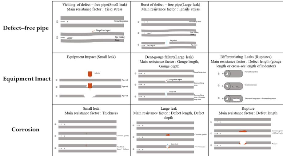
Figure 2. Description about main underground pipeline failure causes for limit state design
