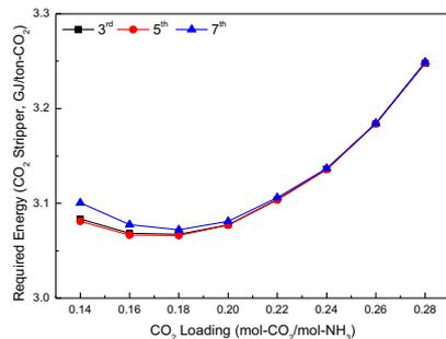
Figure 6. Energy requirement under varying the location of the single inter-heater.
