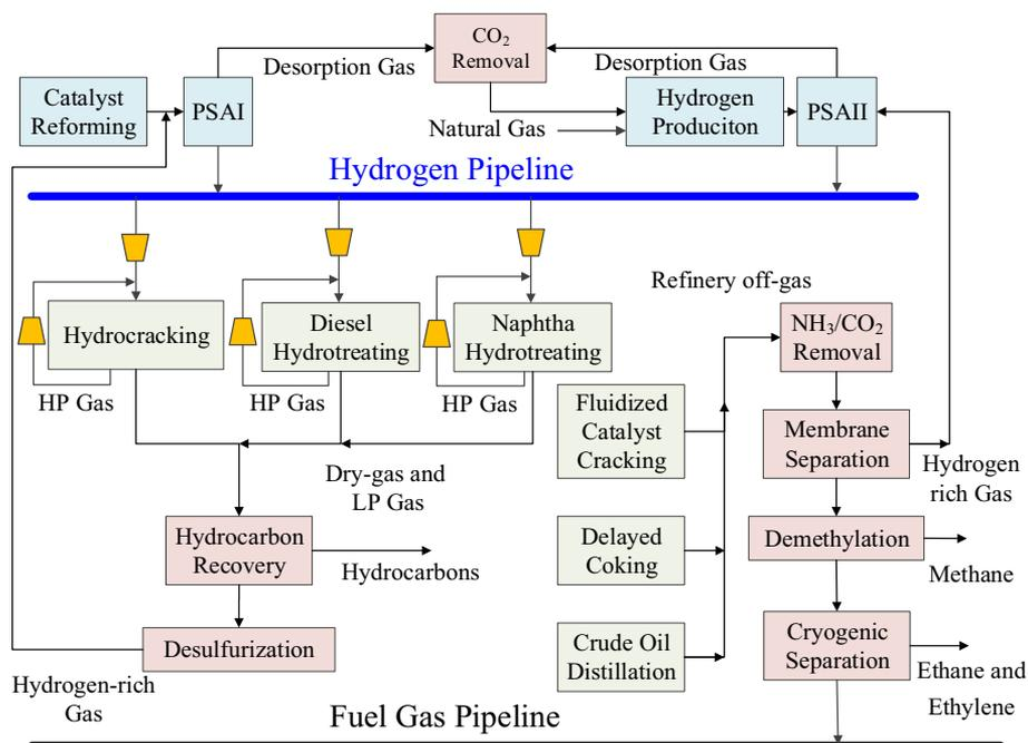
Figure 2: Improved refinery hydrogen network with near - zero hydrogen emission
