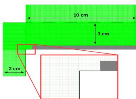
Figure 2. 2D axisymmetric geometry after discretization using a structured mesh containing 120,000 cells.
