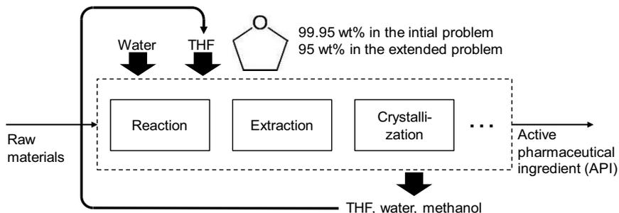
Figure 1. Overview of the main process and the THF recovery process
