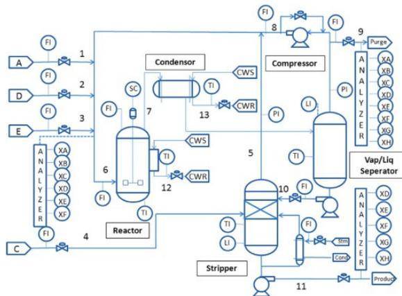
Figure 5. Flowchart of the Tennessee Eastman process
