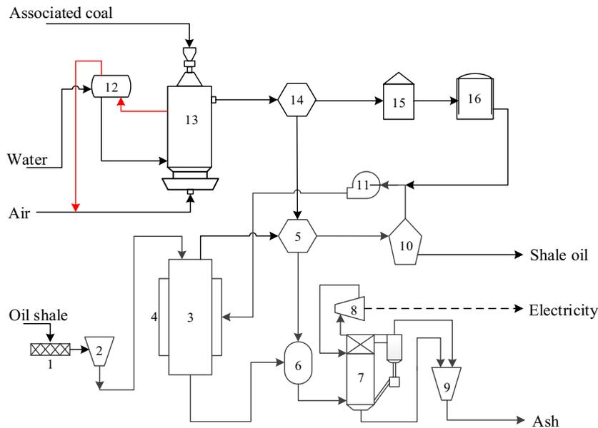
1 grinding mill; 2 shale hopper; 3 retort; 4 gas furnace; 5 flying ash separator; 6 mixture hopper; 7 CFB furnace; 8 steam turbine; 9 ash hopper; 10 oil-gas separator; 11 compressor; 12 steam pocket; 13 gasifier; 14 cyclone separator; 15 intercooler; 16 gas holder
