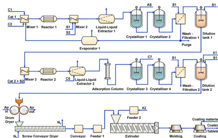
Figure 2: Flowsheet for continuous pharmaceutical pilot plant (Benyahia et al., 2012)
