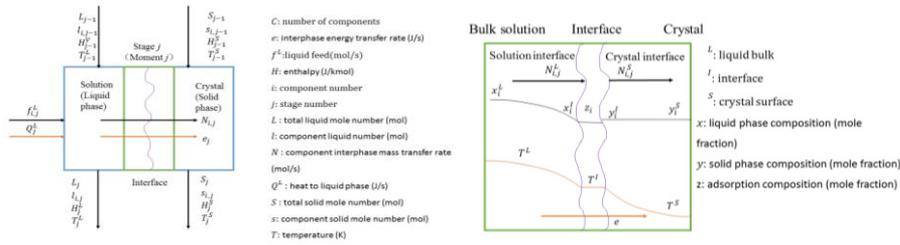
Figure 1 Schematic diagram of non-equilibrium stage model for solution crystallization: stage model (left) and interface model (right)
