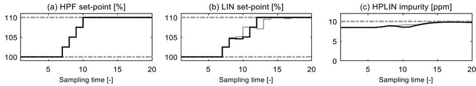
Figure 2: Temporal course of relevant process variables for a 10 % load increase of the ASU without disturbances. Solid black lines show optimal trajectories from NL DO. Thin grey lines show results of the industrial benchmark (without NL DO). Dashed-dotted grey lines show constraints.
