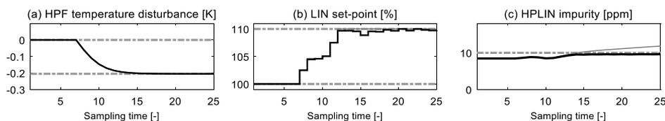
Figure 3: Temporal course of relevant process variables for a 10 % load increase of the ASU considering disturbances. Solid black lines show the simulation using the two-layer APCS. Thin grey lines show the results without tracking control. Dashed-dotted grey lines show constraints
