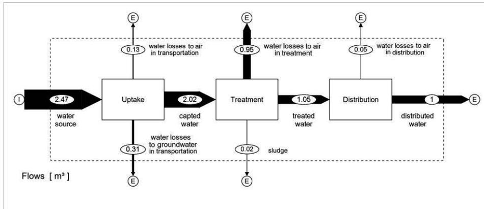
**Fig. 1** Water balance along the water supply system (Base Scenario)
