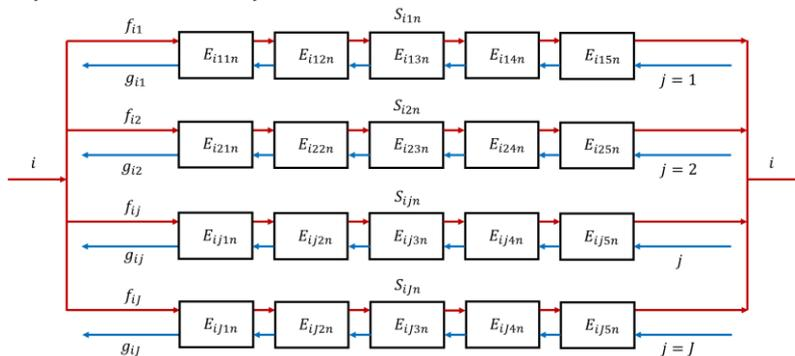
Figure 1. Schematic of our single-stage superstructure with  $I \times J$  potential exchanges.
