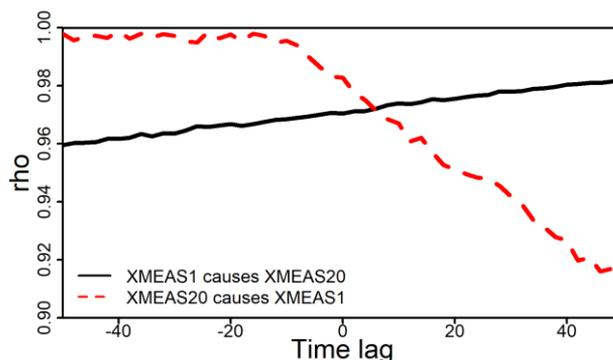
Figure 6: Calculate the correlation coefficient rho by shifting the time lag. In the full line, the time lag maximizing the rho is positive, which means XMEAS1 is the driving variable. In the dotted line, the time lag maximizing the rho is negative, which means XMEAS 20 is the response variable.
