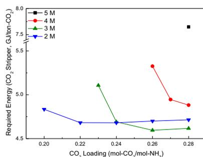
Figure 3. The required energy for the atmospheric CO<sub>2</sub> stripper.
