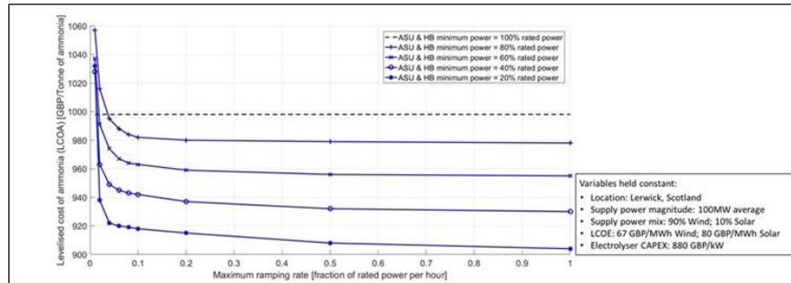
Figure 5: LCOA sensitivity to ASU & HB process minimum power and maximum ramping rate
