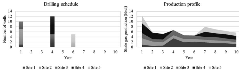
Figure 2. Optimal drilling schedule and shale gas production profiles at shale sites.
