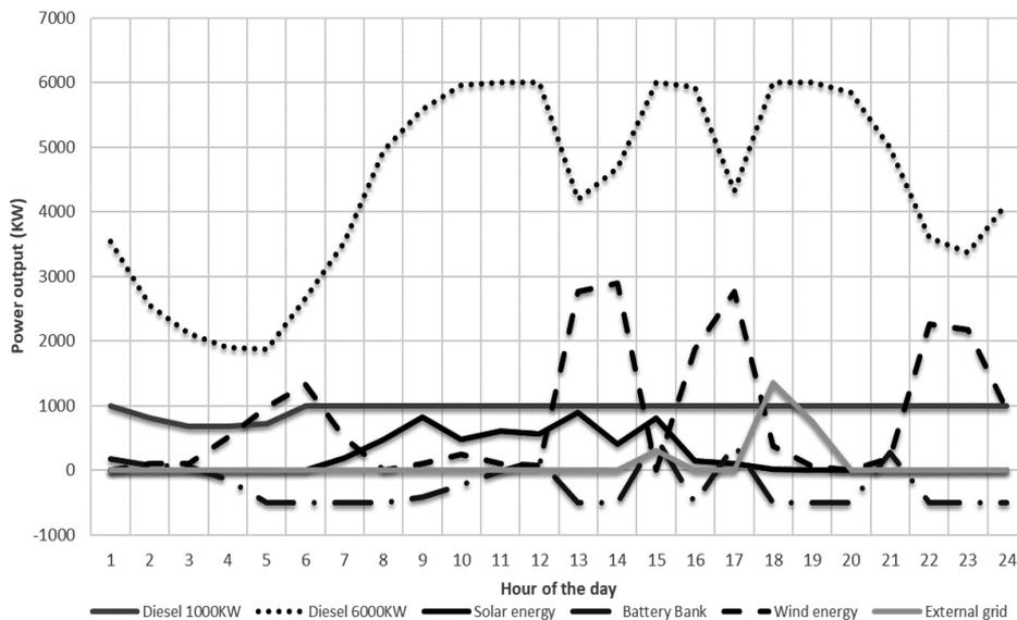
Figure 3. Power output of DES in one-day period
