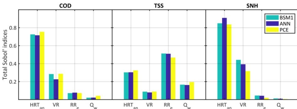
Figure 4: Total Sobol' sensitivity indices are calculated for the model outputs of COD, TSS, and SNH using both the original model (BSM1) and the surrogate models of type ANN and PCE.
