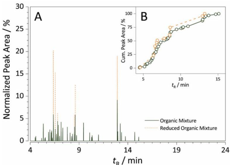
Figure 1. Exemplary depiction of reduction method on the organic phase of dataset 3: A) a normalized GC-MS chromatogram, B) comparison of trends of cumulative peak area over retention time. Experimental organic phase is denoted in full line, while reduced organic phase is denoted in dashed line.
