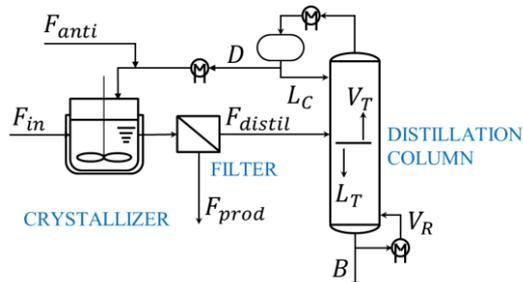
Figure 1. Schematic illustration of continuous anti-solvent crystallization process with antisolvent separation and recycling.
