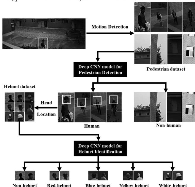
Figure 1-Flowsheet of the automated visual helmet identification method.
