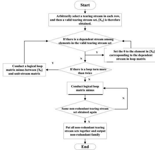
Figure 3 Algorithm block diagram
