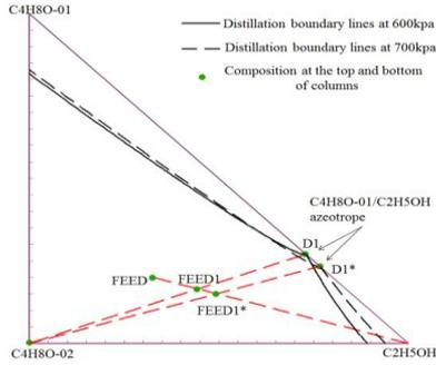
Fig. 6 RCMs of C2H5OH/C4H8O-01/C4H8O-02 at 600kpa and 700kpa
