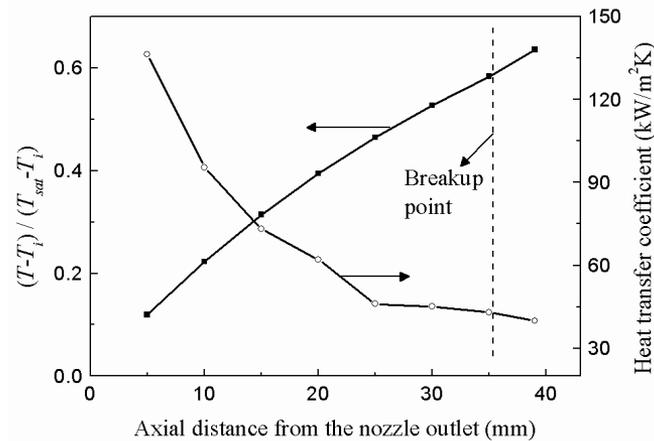
Figure 7: Variations of dimensionless temperature and heat transfer coefficient along the flow direction
