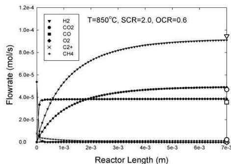
Figure 2. Flowrate profile of main components at different operating conditions. Simulation (closed symbol) compared with the micro-reactor experimental data (open symbol).
