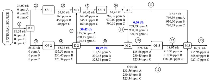
Figure 5. New WN for maximum reuse without violation and new internal flowrate.
