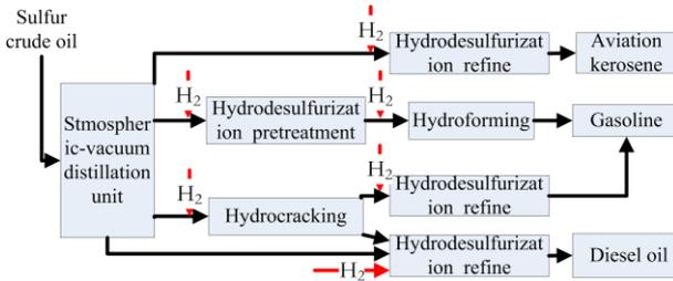
Figure 1: Upstream and downstream sites of hydrodesulfurization in petroleum processing
