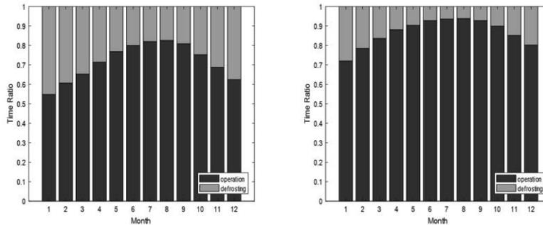
Figure 6. The ratio of operation time to defrosting time (left: original design, right: optimal design – 4 clusters)
