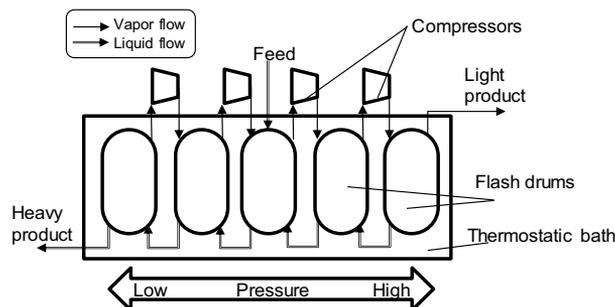
Figure 4. Pressure-driven distillation system (PDDS)
