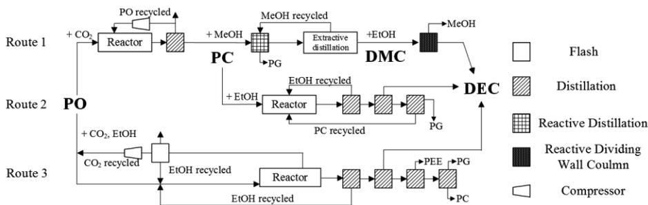
**Figure 2.** Illustration of three DEC synthesis routes.
