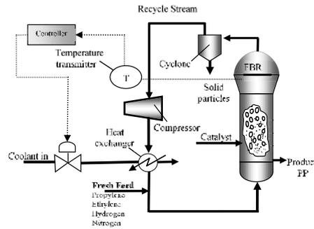
FIGURE 1. Simplified schematic diagram of fluidized bed propylene and ethylene. (from Shamiri et al., 2015)
