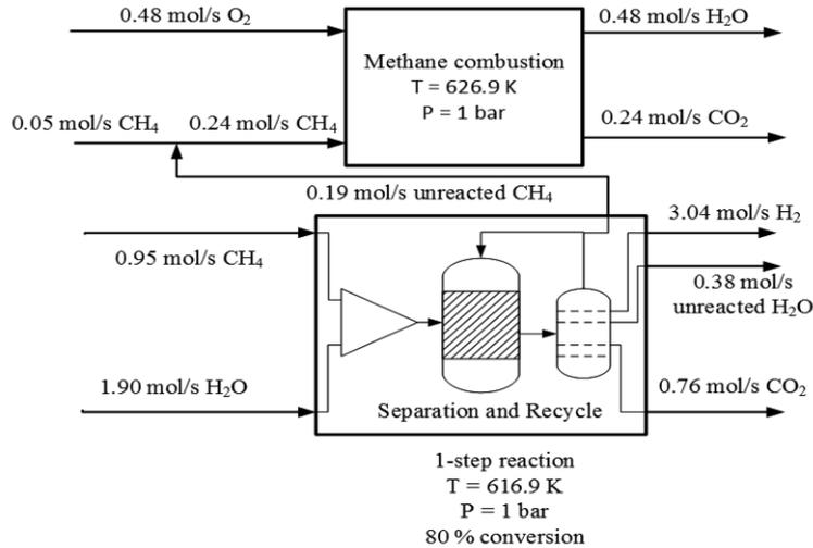
Figure 1: Flowsheet for hydrogen production using the 1-step reaction
