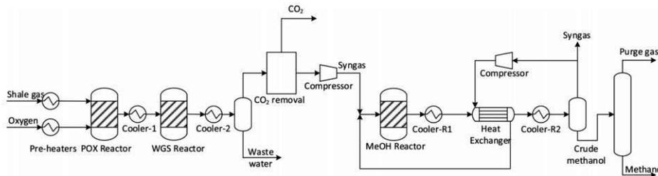
Figure 1. Methanol production flowsheet using POX (Julián-Durán et al., 2014)
