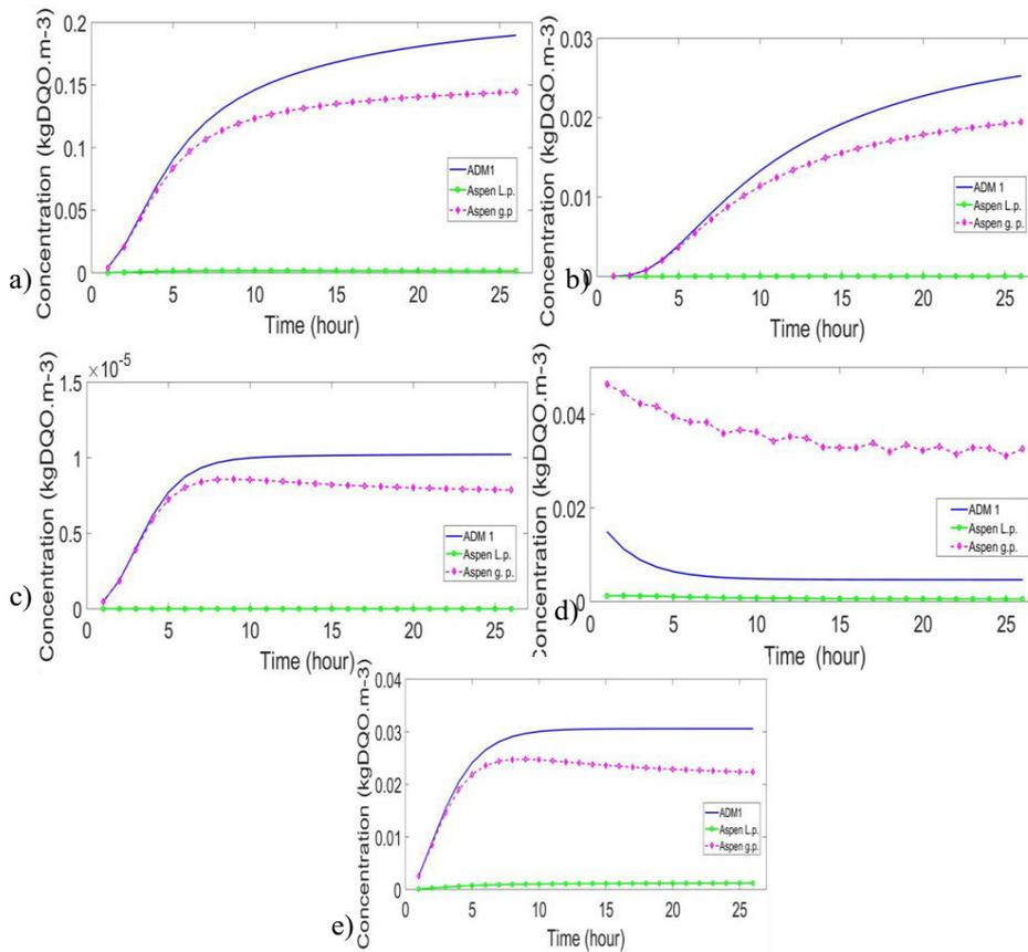
Figure 2- Results for prediction of concentration in each instant t: a) CH<sub>4</sub> b) N<sub>2</sub> c) H<sub>2</sub> d) CO<sub>2</sub> e) Acetic acid
