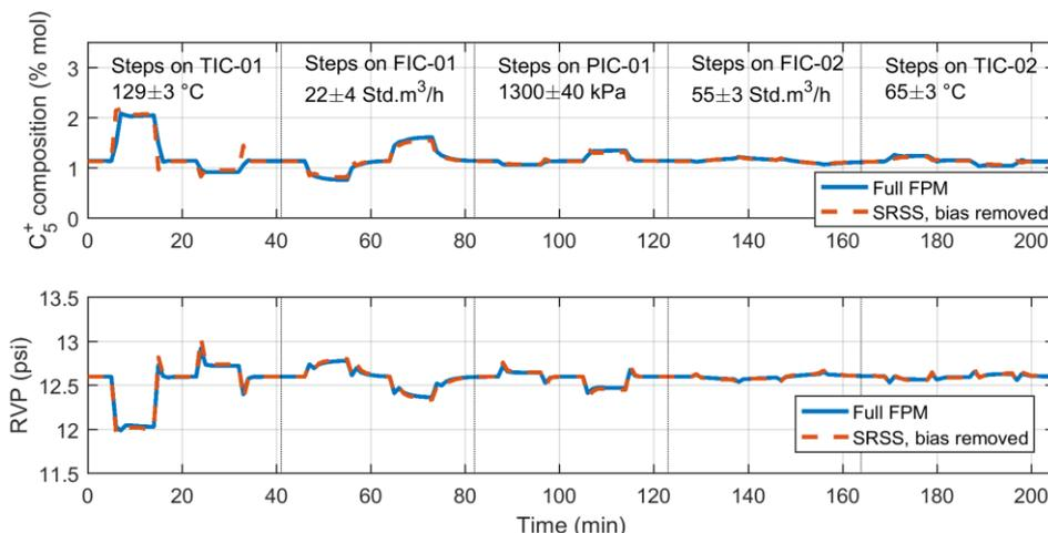
Figure 5. Prediction of total pentanes in the debutanizer overhead product and RVP from bottom product in different step tests in the regulatory controls of distillation units.
