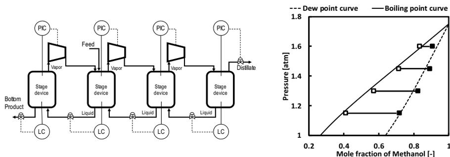
Figure 6. Configuration of 4-stage PDDS (left) and composition distribution (right)
