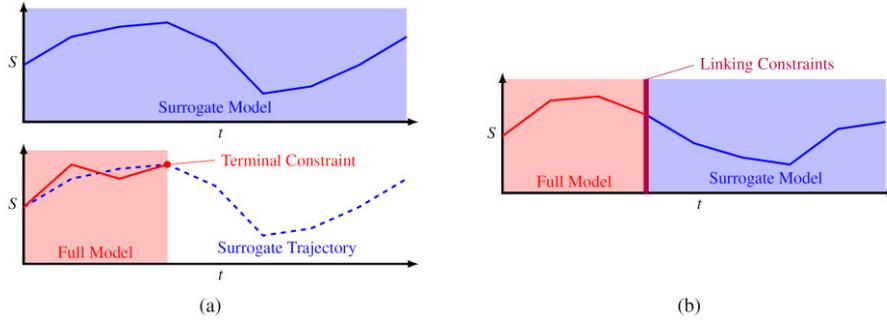
Figure 1: Diagram of two-stage (a) and one-stage (b) hybrid optimization strategies. Axes show different optimization problems, and shaded regions show prediction horizon and model type.
