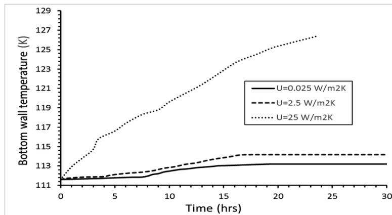
Figure 2. Plot of average bottom wall temperature with time at different values of  $U$ .
