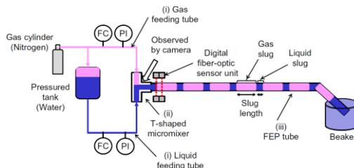
Figure 1 Experimental system of a single T-shaped channel reactor
