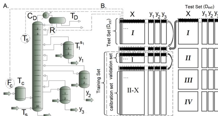
Figure 1. Schematic representation of (A) the CDU; (B) model training/testing algorithm. Construction of the predictor matrix is demonstrated using representative process variables (dashed arrows). Solid arrows (between the blocks of data) represent the inclusion of validation/test data to calibration/training data in stepwise manner for the adaptive local RVM method.
