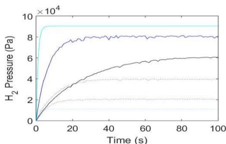
Figure 2. Partial pressures in the cathode.  $H_2$  solid line.  $H_2O$  dotted line.  $j_{el} = [0.02, 0.1, 1]$   $Acm^{-2}$  (darker to lighter).
