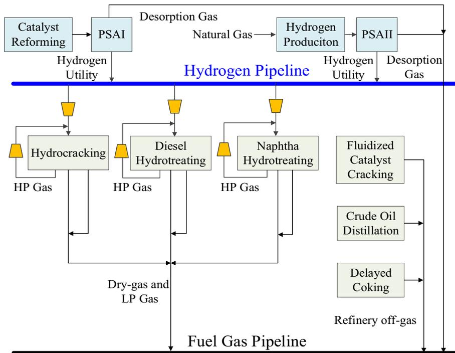
Figure 1: Conventional refinery hydrogen network
