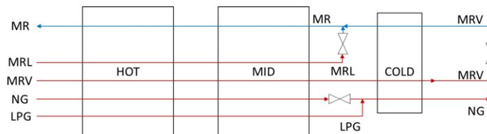
Figure 2. MCHE configuration in the LNG case study
