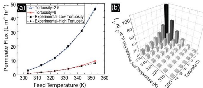
Figure 3. (a) Comparison between experimental results for the permeate flux of two hollow fiber membranes with low and high tortuosity and the prediction of the model for the membranes in a close-packed configuration[15]; (b) effect of feed temperature and tortuosity on the permeate flux.
