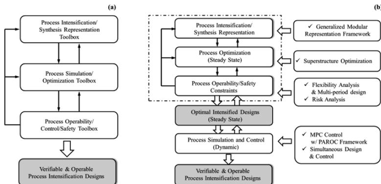
Figure 1. Proposed framework for the synthesis of operable intensification systems
