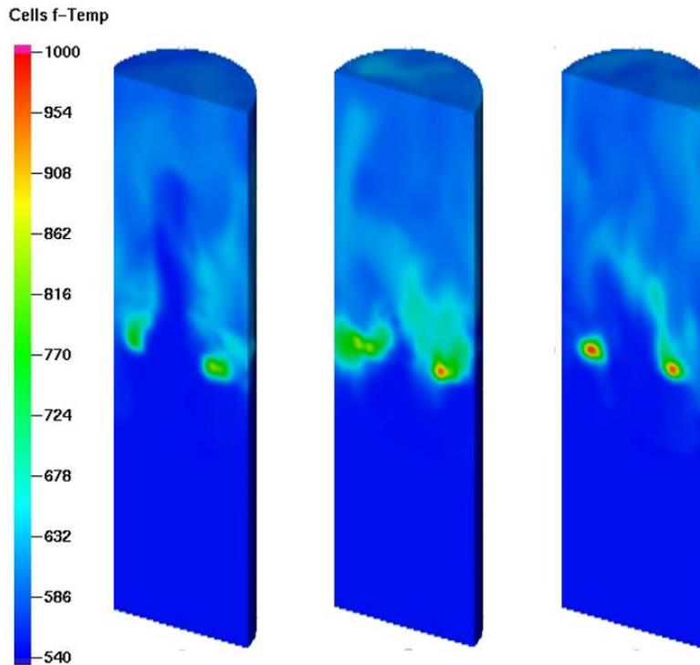
Figure 4: Hot spot profile, (a)5:5, (b)6:4, (c)7:3 (DBP:Water)
