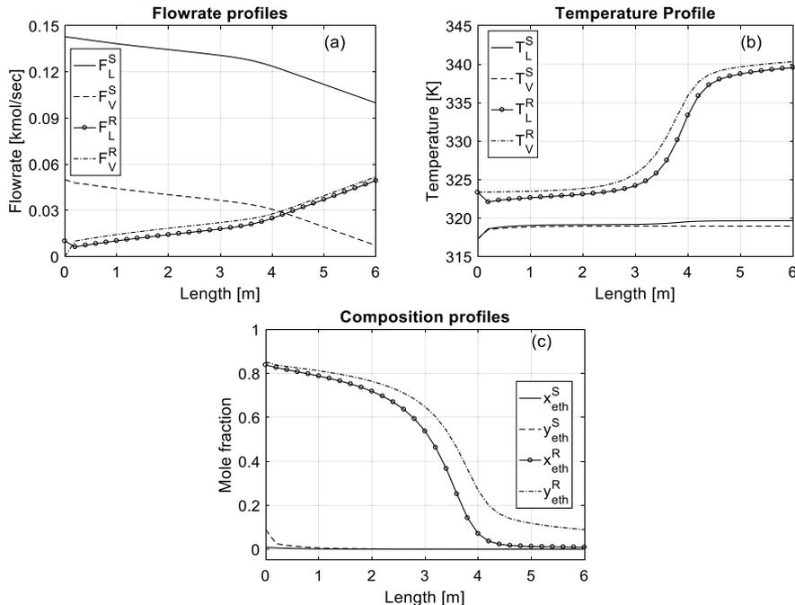
Figure 3. Simulation results for the heat integrated horizontal system. (a) Internal flow rate profiles, (b) internal temperature profiles and (c) internal composition profiles. Note that in the liquid flows direction [0→6 m] and the vapor flows at the opposite direction.
