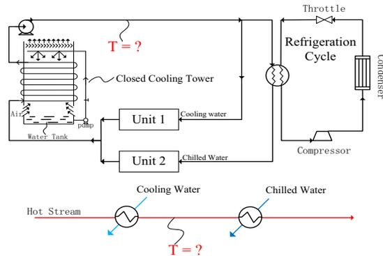
Figure 1. Illustration of two-stage cooling configuration.
