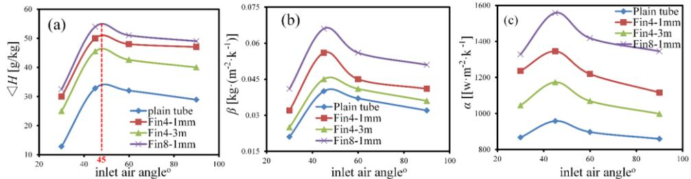
Figure 3 Influences of inlet air angle on (a) humidity difference ( $\Delta H$ ), (b) air-water mass transfer coefficient  $\beta$ , and (c) heat transfer coefficient  $\alpha$
