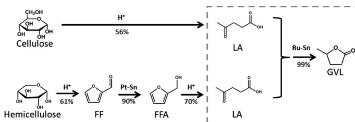
**Figure 1.** Reaction scheme of the LA-based GVL production from lignocellulosic biomass.
