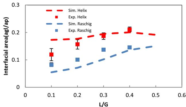
Figure 2 The validation of the interfacial area of helical rings and Raschig rings
