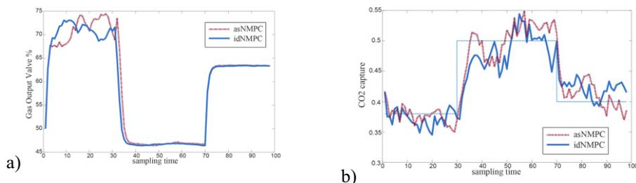
Figure 3 Results for the NMPC of the BFB; a) controller input profile, b) output profile
