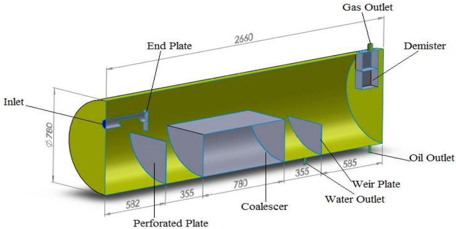
**Fig. 1.** Geometry of air-oil-water separator.
