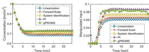
Figure 4. Closed loop performance comparison for the various controllers and open loop dynamic optimization for the CSTR example
