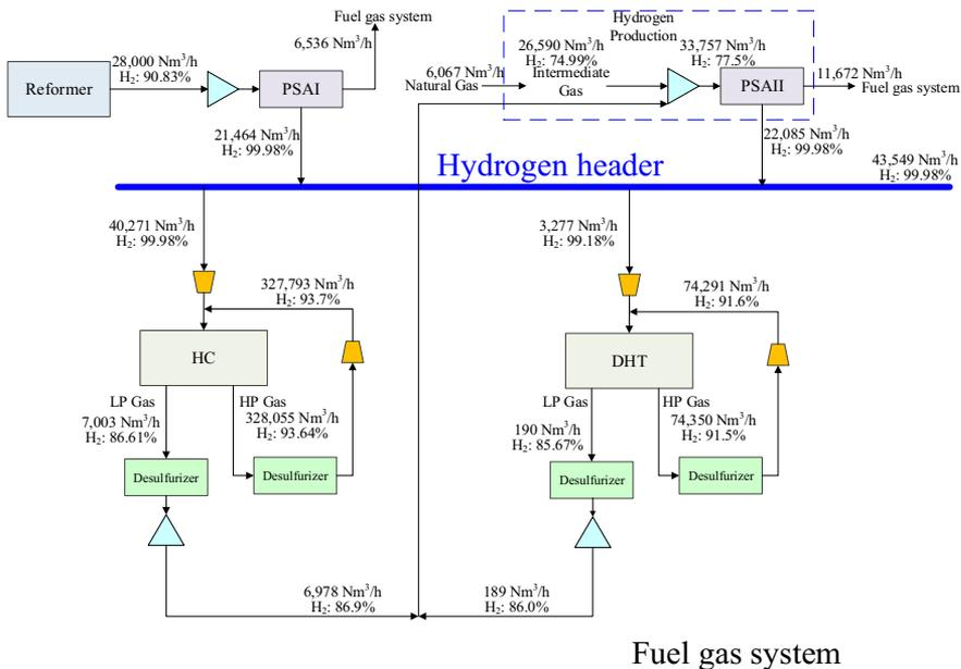
Figure 1: Current hydrogen network
