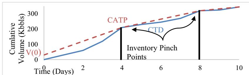
Figure 1: Example of inventory pinch points obtained from constructing CTD and CATP curves
