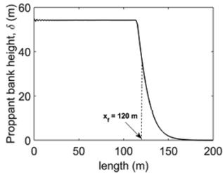
Figure 5. Spatial proppant bank height profile obtained at the end of pumping.
