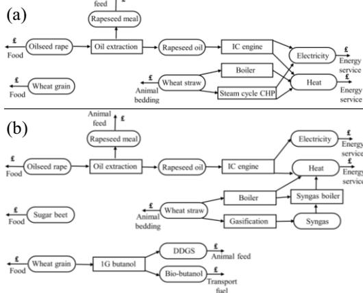
Figure 5. Optimal biomass value chains in (a) 2010 and (b) 2050
