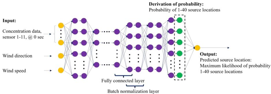
Fig. 3 Feed-forward neural network using the current time point data as inputs.
