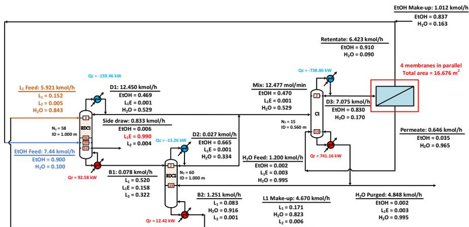
Figure 4. Reactive distillation with pervaporation (RD + PV) configuration
