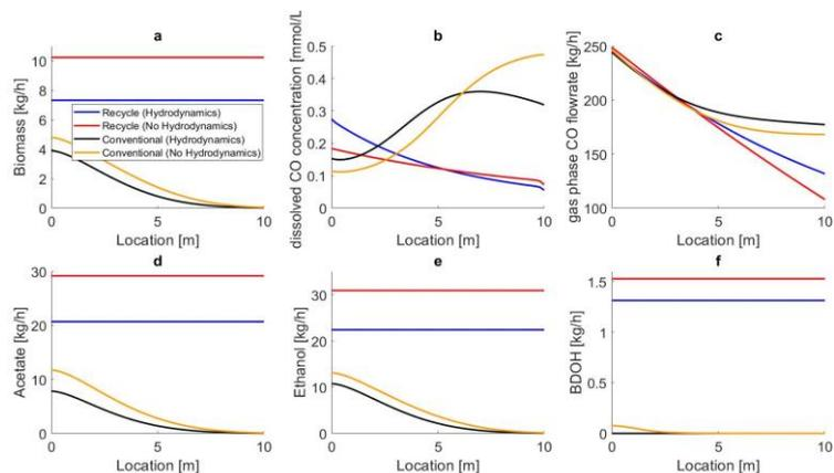
**Figure 2.** Steady-state production rate profiles predicted for two bubble column reactors (conventional, liquid recycle) with and without hydrodynamics. The liquid phase exited the column at  $z = 0$  m and the gas phase exited the column at  $z = 10$  m. Liquid-phase concentration profiles for the recycle reactors were flat due to the assumption of homogeneity.
