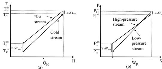
Figure 2. Comparison of (a) heat transfer in a HE and (b) work transfer in a WE.
