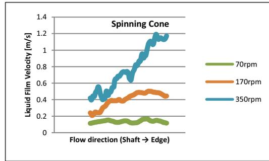
Figure 4. Liquid film velocity on the spinning cone with different rotation speed
