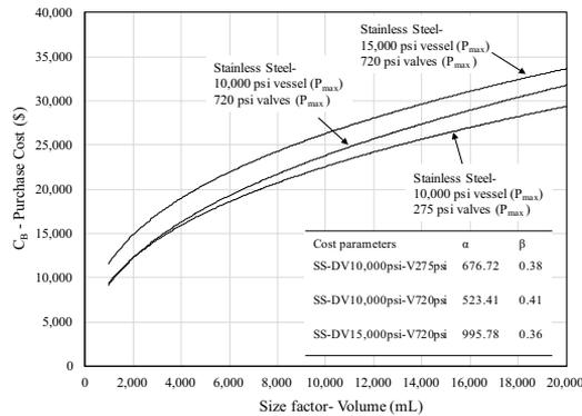
Figure 4. Cost estimation for one work exchanger unit.
