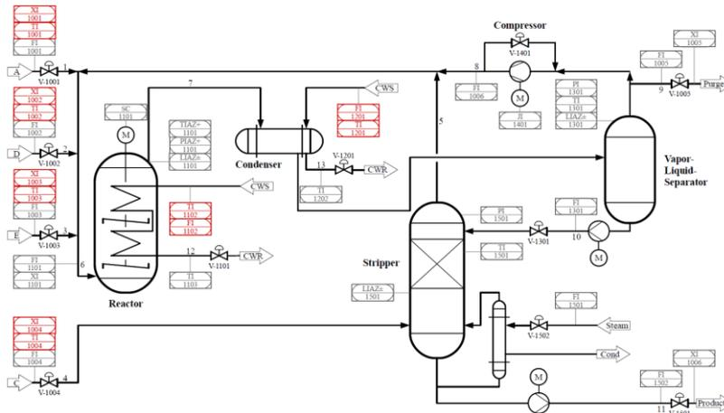
Fig. 1 P&ID of the revised TE process model;
