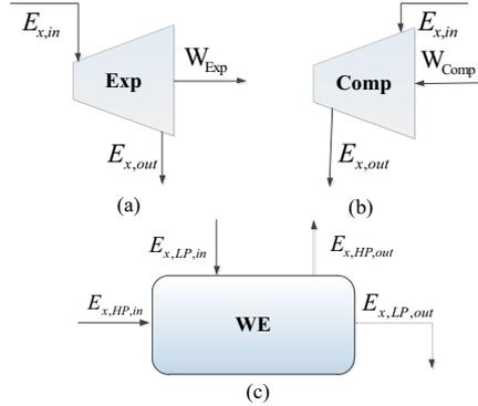
Figure 3 The exergy analysis for expander (a), compressor (b) and work exchanger (c)
