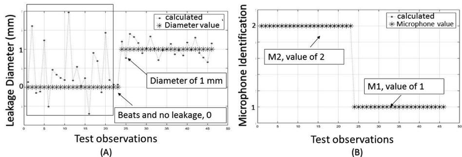
Figure 2. Values calculated by the supervised network and the observations used to test the network. (A) Leakage diameter value; (B) Microphone value
