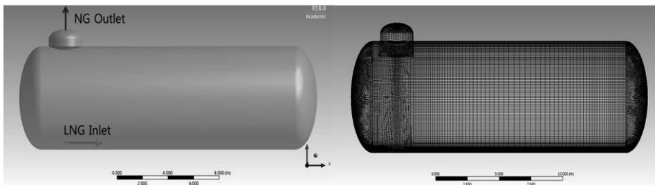
Figure 1. Geometry and mesh of a LNG tank
