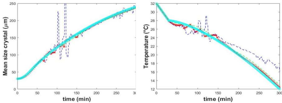
Figure 2- Mean particle size (left) and temperature profile predictions (right) of the different RBFs. (full: reference trajectory and temperature, dashed: IMQ RBF, remaining lines are similar to the reference trajectory)
