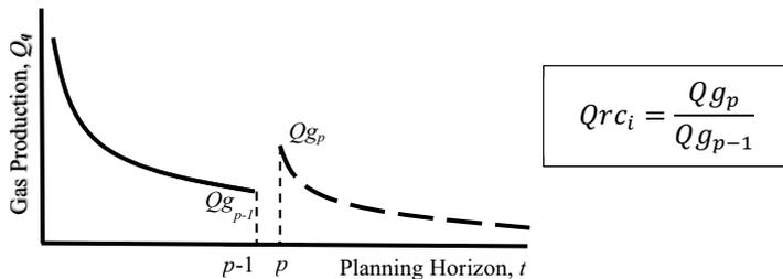
Figure 1. Production decline curve before and after ALM  $i$  is installed.
