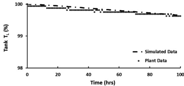
Figure 4. Bulk Liquid temperature profile inside tank
