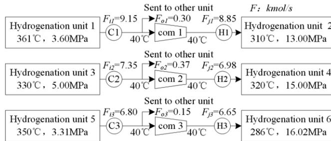
Figure 2 The schematic diagram of case
