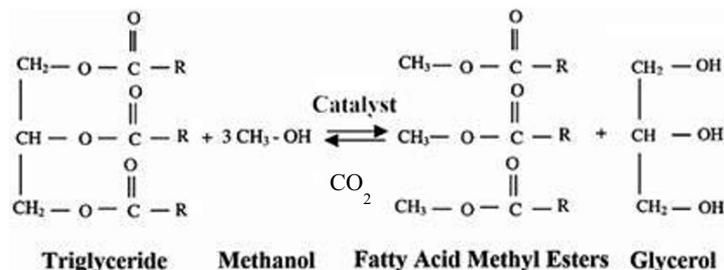
Figure 1. A single reversible transesterification reaction to convert triglycerides into biodiesel
