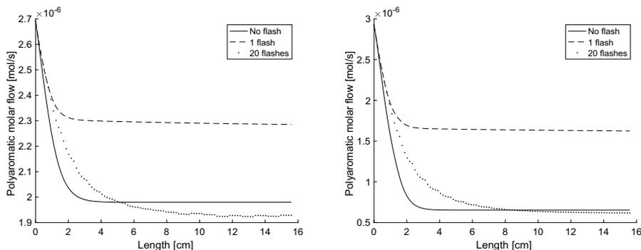
Figure 4 Molar flow profile of polyaromatic compounds with or without flashes. The plots present the feed with 75 wt.-% (left) and 25 wt.-% methylated substrate (right).
