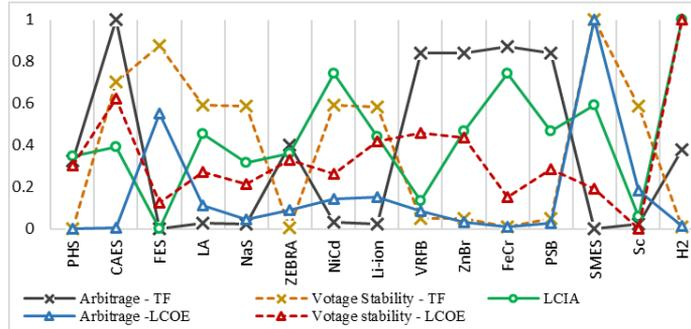
Figure 2. Trend for  $TF_i$ ,  $LCOE_i$  and  $LCIA_i$  with varying technologies for arbitrage and voltage stability applications, where values are normalized.
