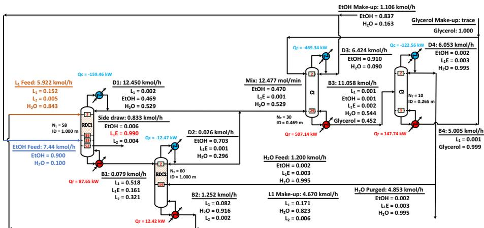
Figure 3. Reactive distillation with extractive distillation (RD + ED) configuration
