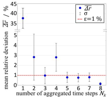
Figure 4: Mean relative deviation  $\overline{\Delta r}$  of the objective function value of the 25 working fluids identified with 1-stage CoMT-CAMD using  $N_k$  aggregated time steps and the full time series as well as the corresponding standard deviation  $\sigma$  over all working fluids.
