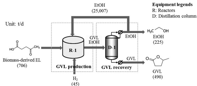
**Figure 4.** Simplified process flow diagram of EL-based GVL production process.
