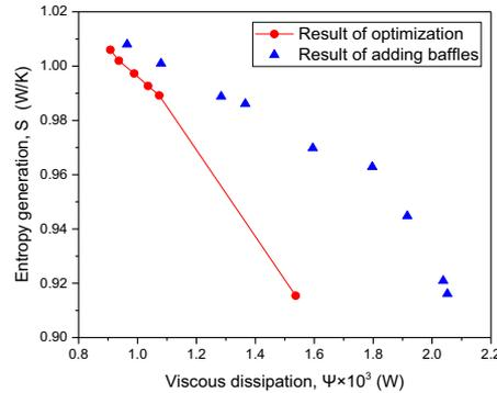
Figure 7: Entropy generation comparison after optimization and adding baffles
