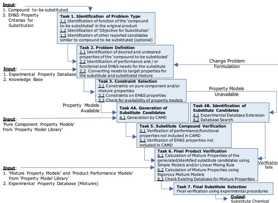
Figure 2: Methodology for Model-based Chemical Substitution
