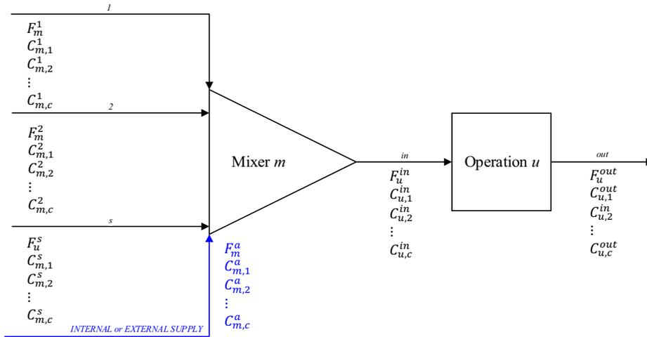
Figure 2. Scheme for the addition of water supply.
