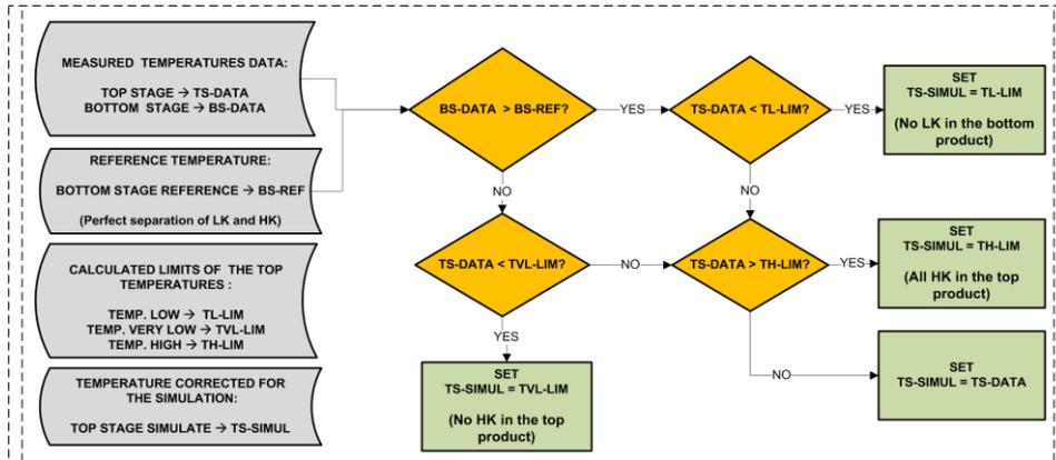
Figure 3. Temperature data correction scheme based on the top stage constraints.
