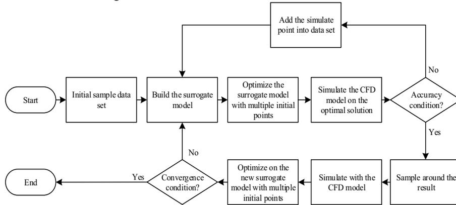
Figure 3. Flowchart of the iterative surrogate model method.
