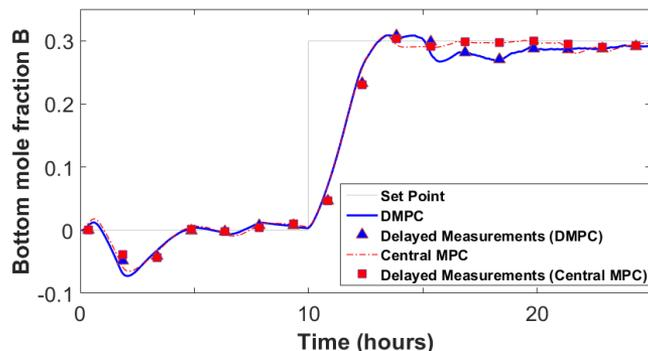
Figure 3: Comparison between centralized and distributed MPC (with primary variable sampled at 90 min). Markers represent the values of primary variables plotted at the arrival time.
