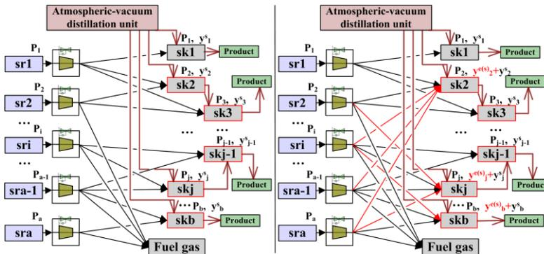
Figure 2: Original structure (left) and superstructure (right)
