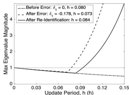
**Fig. 3.**  $\lambda_{\max}$  ( $M$ ) as a function of the update period under normal operation (dash-dotted), under plant-model mismatch (dashed) and for the identified model (solid).
