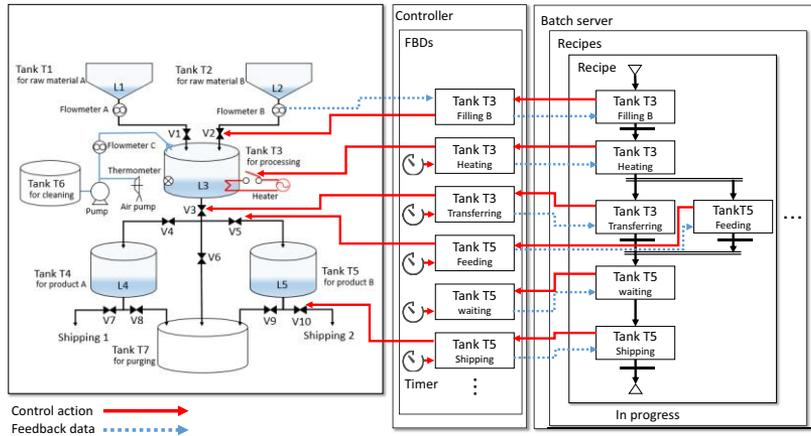
Figure 3: Control Structure Diagram in More Detail
