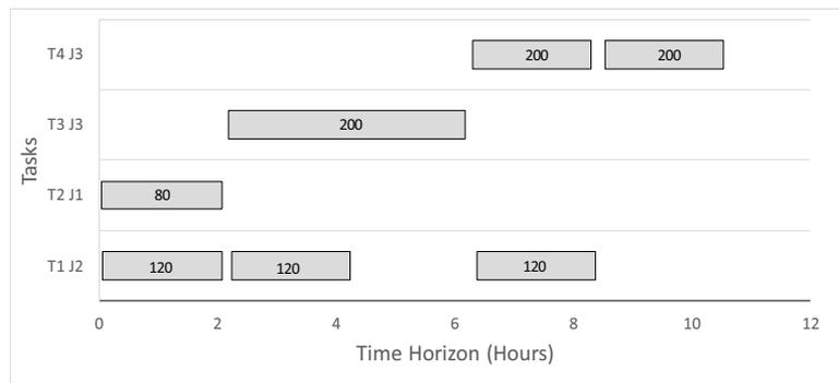
Figure 5 Optimal processing schedule using floating pumps
