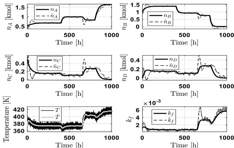
Figure 2. Trajectories of  $n_A$ ,  $n_B$ ,  $n_C$ ,  $n_D$ ,  $T$  and  $k_f$ : Simulated (—), Estimated (---)
