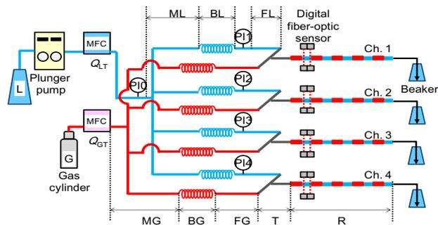
Figure 5 Experimental system of a multi-channel reactor
