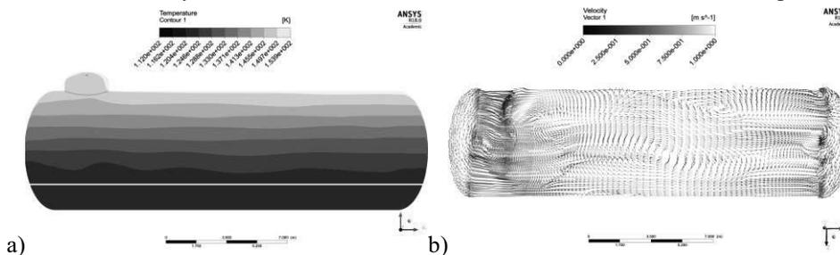
Figure 2. CFD result of a LNG tank in a pseudo-steady state, a) temperature, b) velocity.
