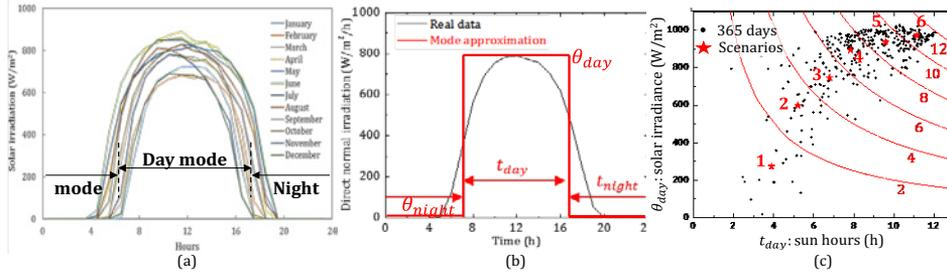
Figure 3. (a) Daily profiles of solar irradiance (b) mode-represented profiles from piecewise constant approximation and (c) 6 scenarios generated from 365 days.
