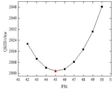
Fig. 9 The dependence of the reboiler heat duty on feed stage of T1 column
