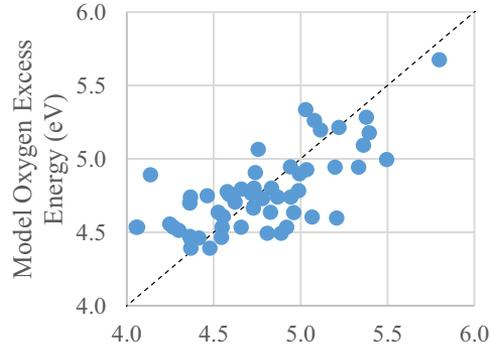
Figure 3: Parity between DFT evaluations and simplified structure-function model evaluations
