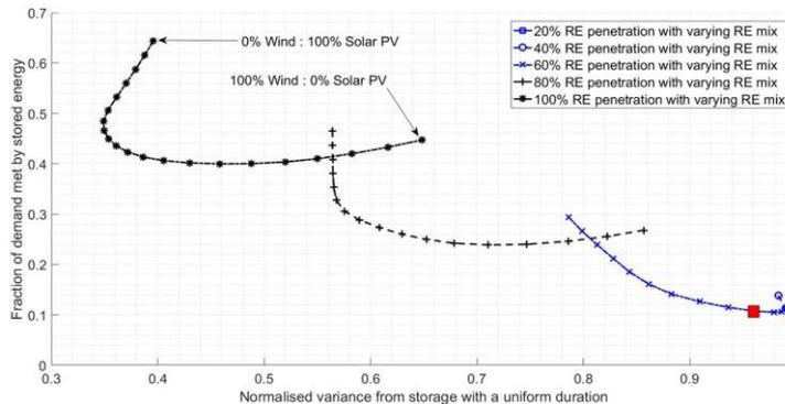
Figure 2: The impact of RES ratio (Wind:Solar PV energy supplied) and RES penetration on the system's storage duration index (SDI)
