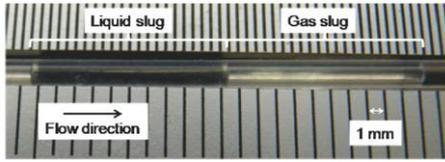
Figure 2 Slug flow in the FEP tube
