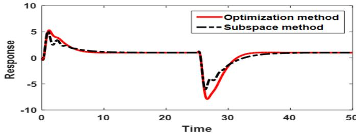
Figure 3: Closed loop response of the controllers designed based on the identified model by optimization method and subspace methods by IMC method for example 1
