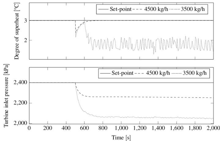
Figure 2: Response of process variables to significant decreases in exhaust gas flow rate
