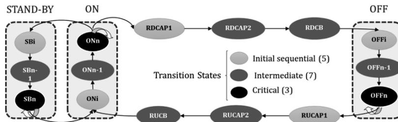
**Figure 1.** Process Transition Network (Basán *et al.*, 2018). Operation modes with minimum stay time: on ( $ON_i$ ,  $ON_{n-1}$ ,  $ON_n$ ), stand-by ( $SB_i$ ,  $SB_{n-1}$ ,  $SB_n$ ), and off ( $OFF_i$ ,  $OFF_{n-1}$ ,  $OFF_n$ ). Start-up operation modes: ramp-up compressor A phase I (RUCAP1) and II (RUCAP2), and ramp up compressor B (RUCB). Shutdown modes: ramp down compressor A phase I (RDCAP1) and II (RDCAP2), and ramp down compressor B (RDCB).
