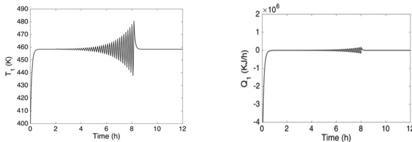
**Fig. 2.** Closed-loop temperature (left) and heat input rate (right) profiles for the first reactor.
