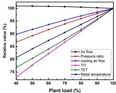
Figure 3 Plant operating variables versus plant load under FFC.
