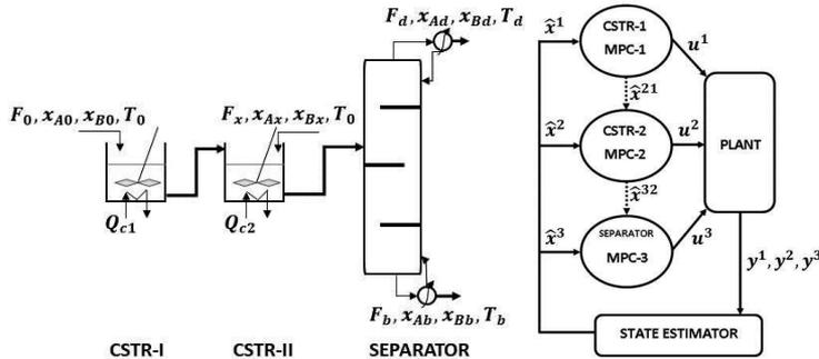
Figure 1: (a) Schematic of the reactor-separator system considered; (b) DMPC architecture
