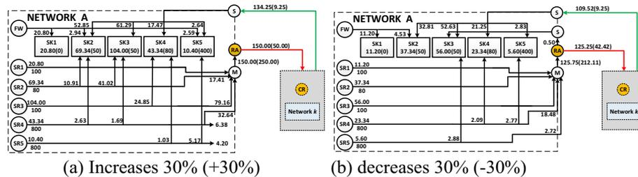
Figure 1. Water network structure of plant A at its production scale changing 30 %
