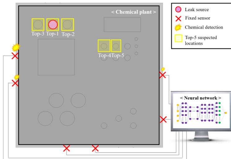
Fig. 1 Schematic diagram of the leak-source tracking system using fence-monitoring data.
