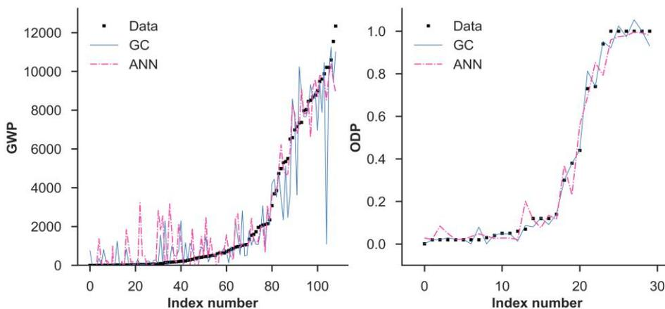
Figure 1: Comparison of group contribution method (line) and artificial neural network (dashed line) based method for predictions of the global warming potential data (left) and ozone depletion potential data (right). ANN models more closely follow the data points.
