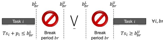
Figure 1. In non-preemptive scheduling, a task can either end-before or start-after a break.
