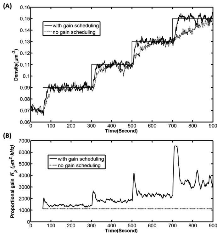
Figure 3. (A) Density and (B) Proportional gain as function of time during a set-point tracking experiment for cases with and without gain scheduling.
