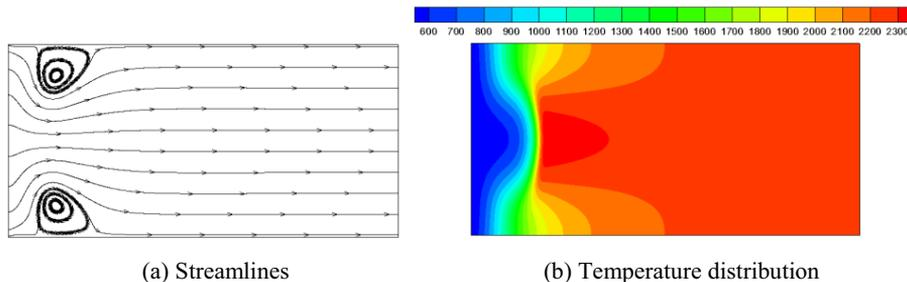
Figure 4: Streamlines and Temperature distribution with optimization
