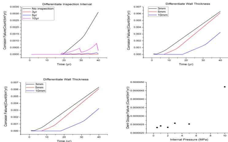
Figure 3. Case studies about propylene pipeline failure rate changes (Differentiate Inspection Interval and pipeline parameters)
