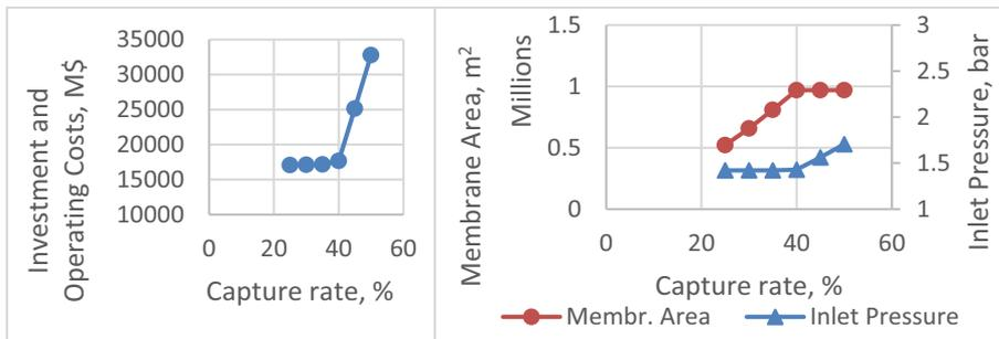
Figure 3. Single unit MOO analysis (M1 – membrane 1), costing method - Hasan et al. (2012).
