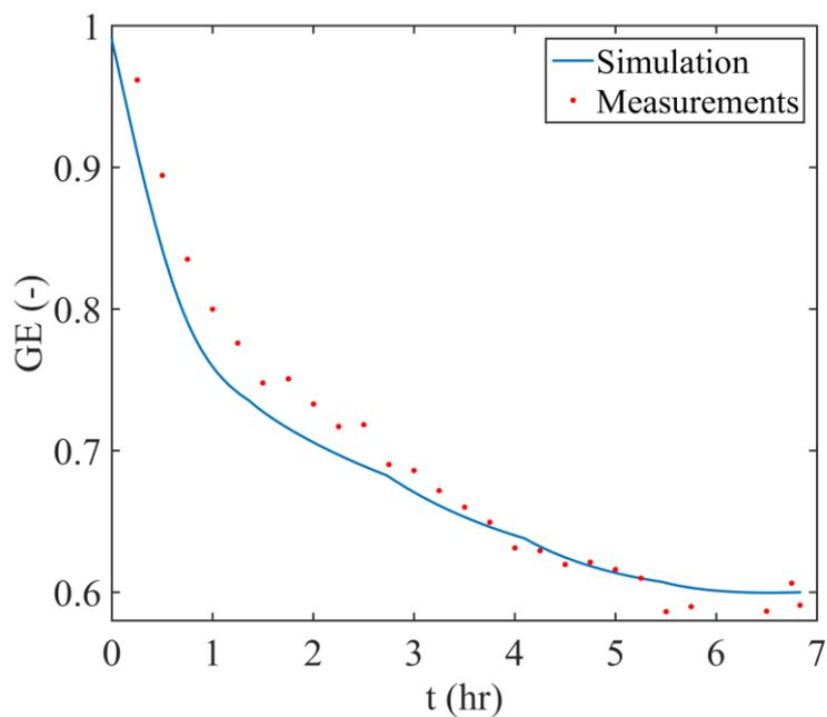
Figure 3: Time-varying profile of the grafting efficiency for  $GE_f = 60\%$  and  $X_f = 80\%$ .
