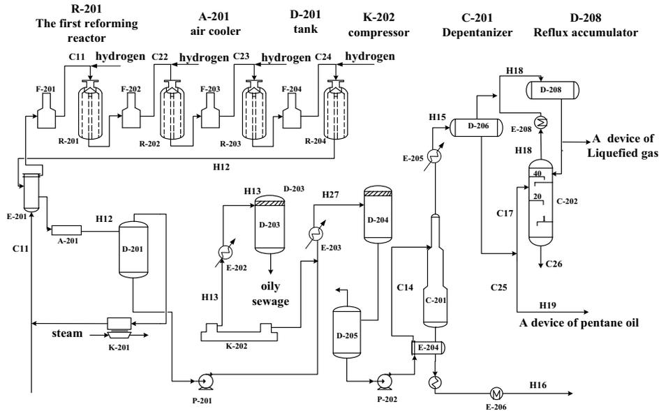
Figure 2. The reforming process of CRR unit
