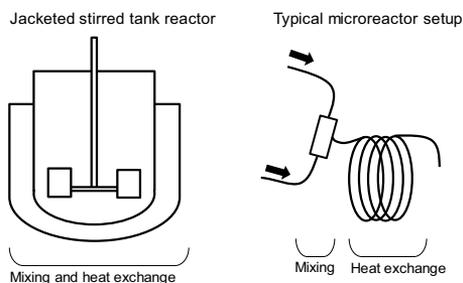
Figure 1. Functions of stirred tank reactor and microreactor setup
