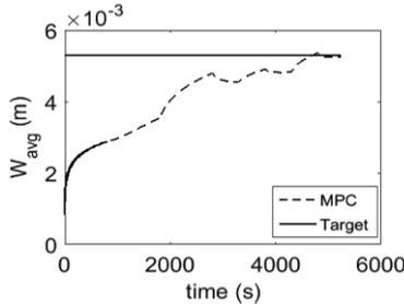
Figure 3. Average fracture width
