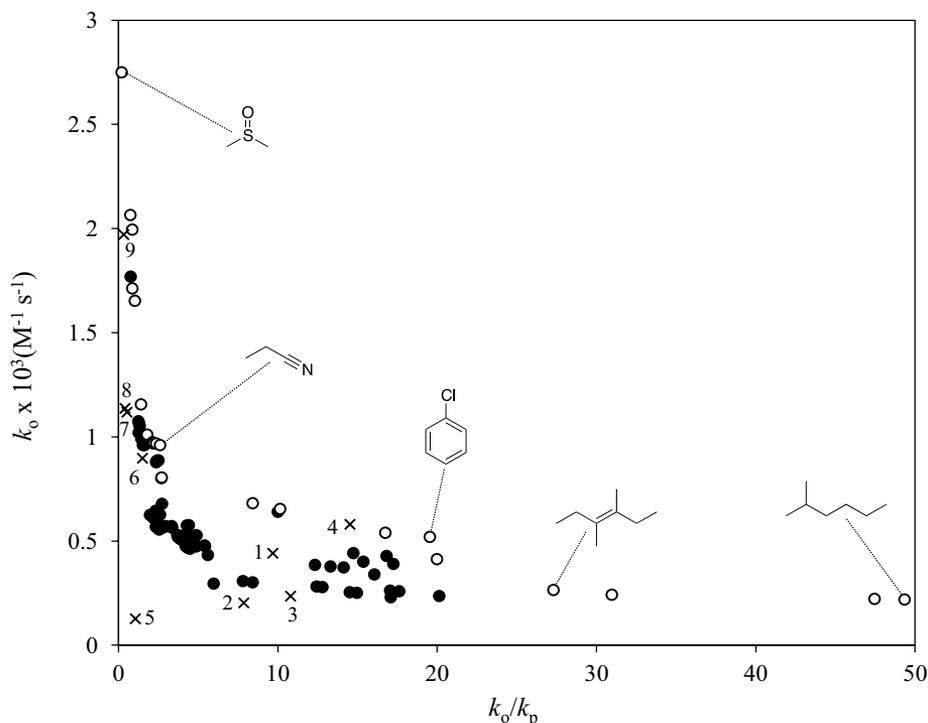
Figure 3: Experimental and CAMD solutions to the MOO problem. Numbered crosses correspond to the experimental values for the solvents in the initial set, closed circles correspond to dominated solutions to the optimization problem, and open circles indicate the Pareto-optimal solutions with example molecules highlighted.
