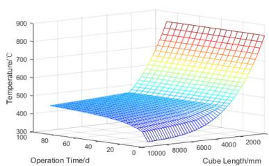
Figure 4. The temperature distribution of the TLE system.
