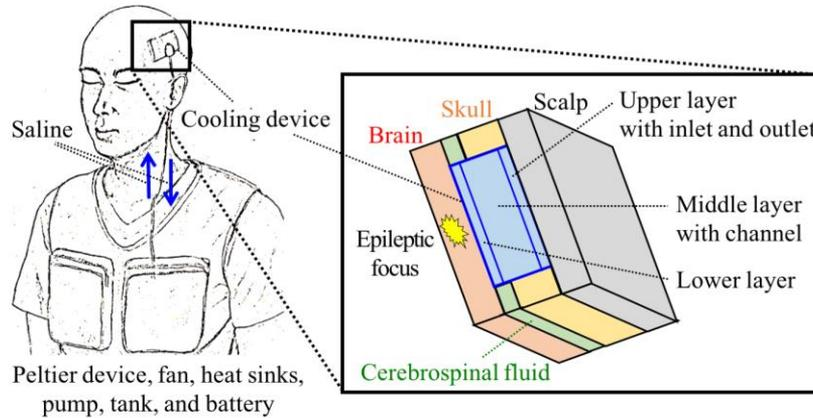
Figure 1. Focal brain cooling system.
