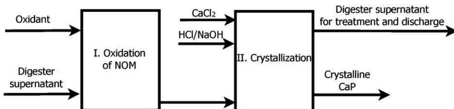
Figure 3. Hybrid oxidation/crystallization technology for high-purity CaP recovery.
