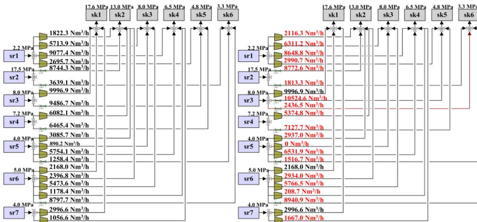
Figure 4 Optimal network of 0.4 % sulfur content (left) and 2.8% sulfur content (right)
