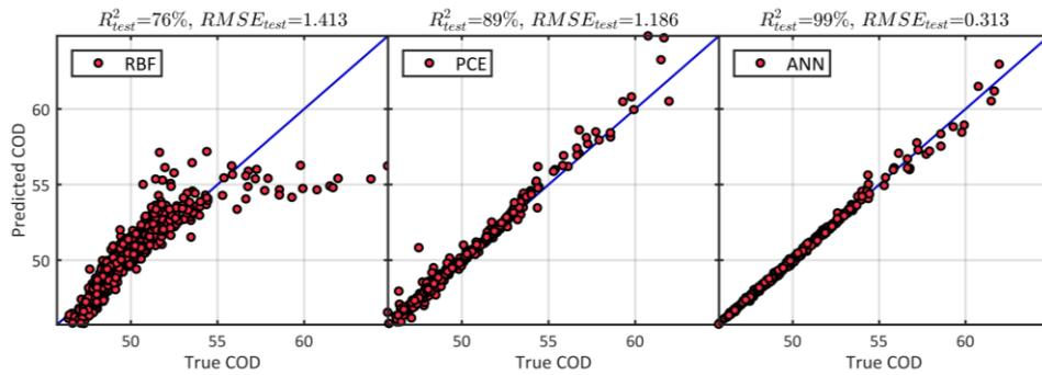
Figure 3: Predictions of RBF, PCE, and ANN type surrogate models trained on a sample size of 200 are compared for the original model response of COD.
