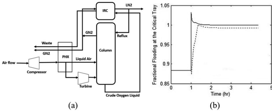
Figure 1 (a) Schematic of nitrogen plant, (b) Ratio of vapor velocity to flooding velocity for step changes in manipulated variables (solid line) and optimized inputs (dot-dashed line)
