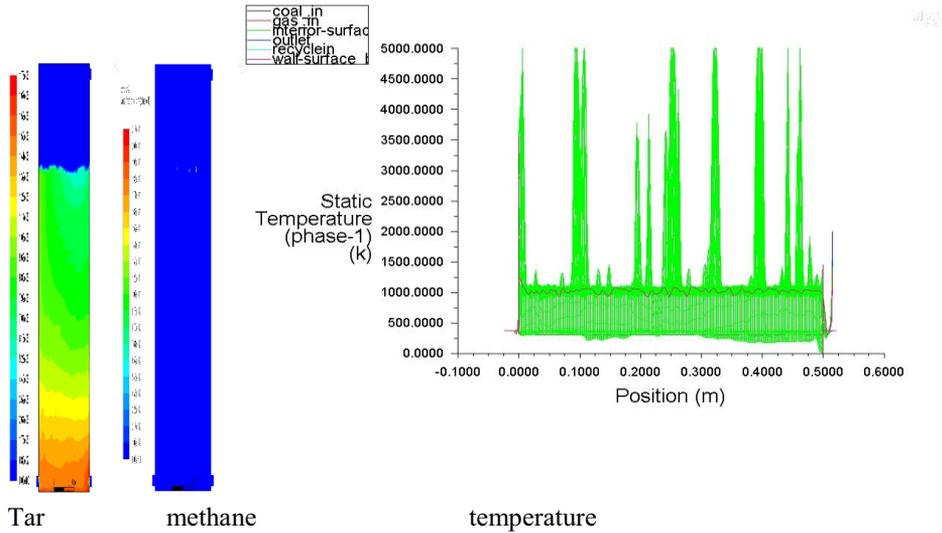
Figure 1: Model results with zero input of syngas from the recycle stream
