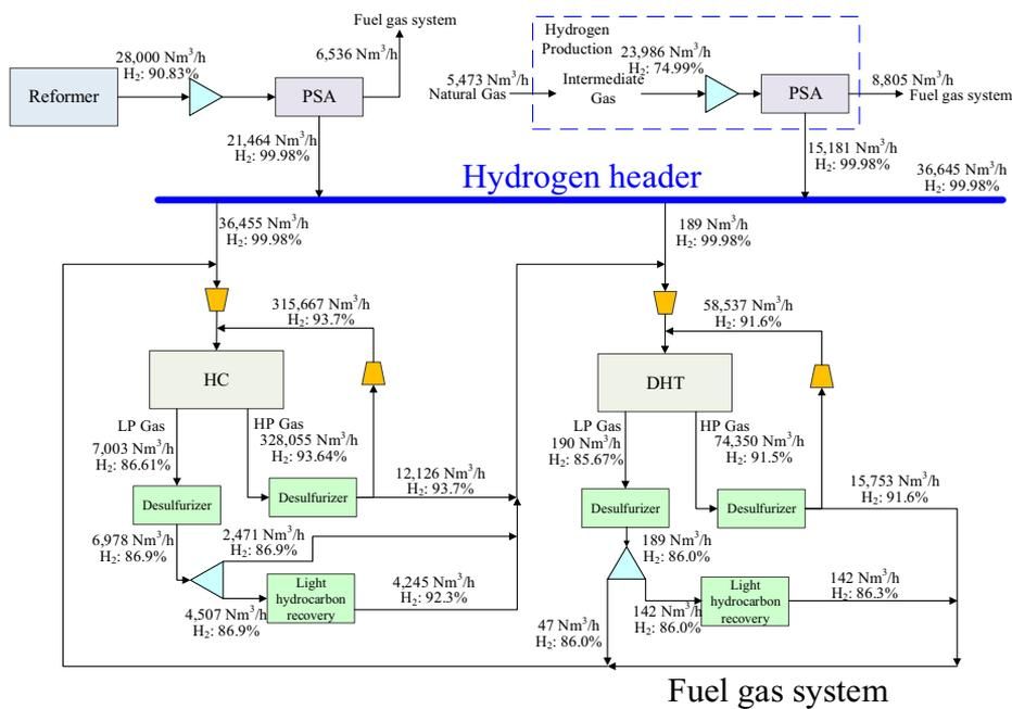
Figure 2: Optimal retrofitted hydrogen network
