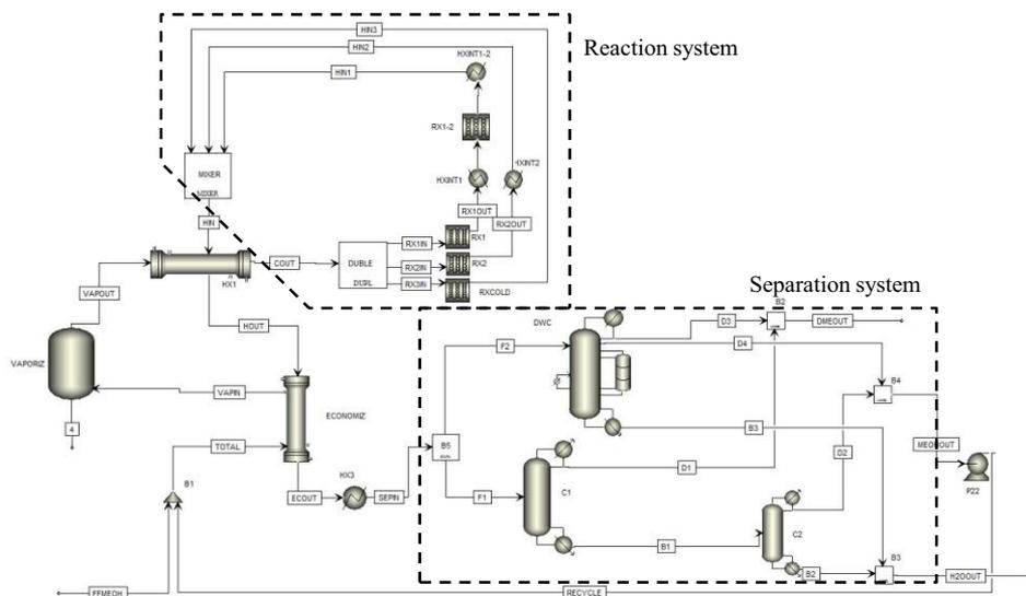
Figure 2: Aspen Plus® flowsheet of the superstructure for the multi-objective optimization of a dimethyl ether production process.
