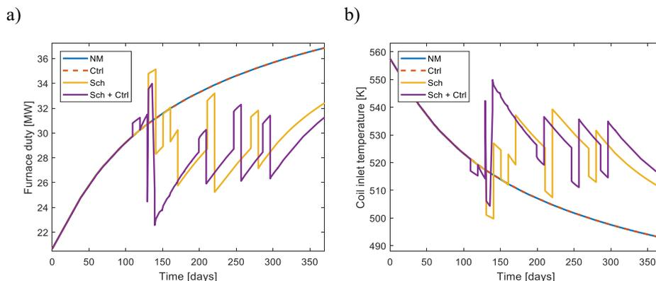
Figure 2. Case study furnace duty (a) and CIT (b) for the optimal cleaning schedule.
