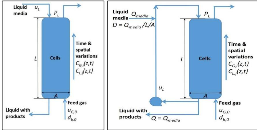
**Figure 1.** Schematic representation of the countercurrent bubble column reactors.  $u_{G,0}$  and  $d_{b,0}$  are the feed superficial gas velocity and bubble diameter,  $u_L$  is the liquid velocity,  $L$  is the reactor length,  $A$  is the reactor cross-sectional area,  $P_L$  is atmospheric pressure,  $Q_{media}$  is the media feeding rate, and  $D$  is the dilution rate.
