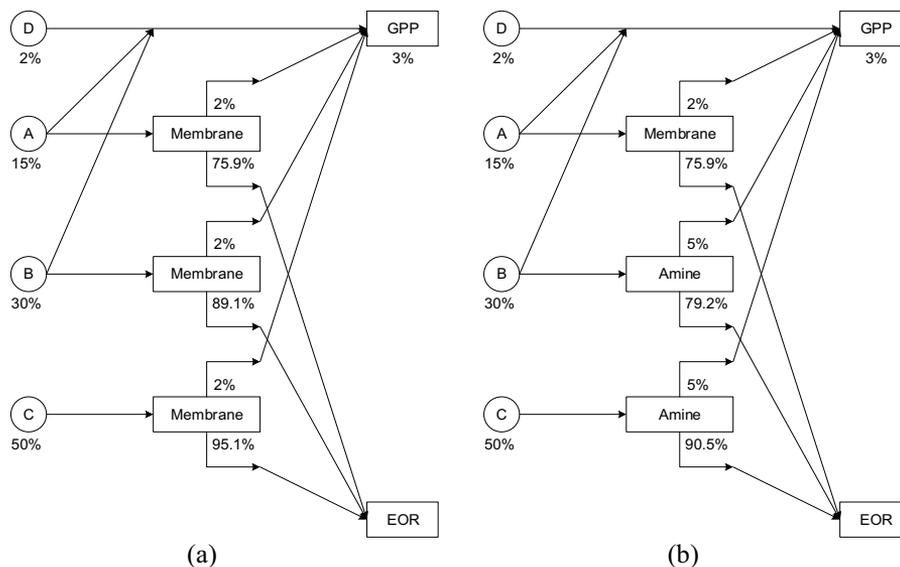
Figure 3. Gas Sweetening System for (a) Scenario 1 and (b) Scenario 2.
