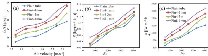
Figure 6 (a-c) shows the humidity difference( $\Delta H$ ), mass transfer coefficient( $\beta$ ) and heat transfer coefficient ( $\alpha$ ) of the four tube cases with respect to a variable inlet air velocity.
