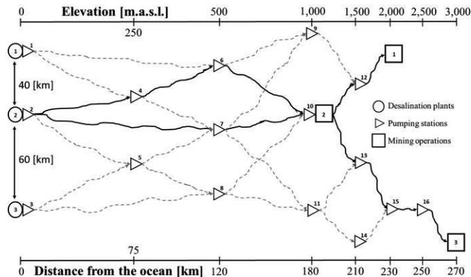
**Figure 1:** Conceptual representation of case study (dotted lines are potential pipes; the continuous lines represent the optimal solution).
