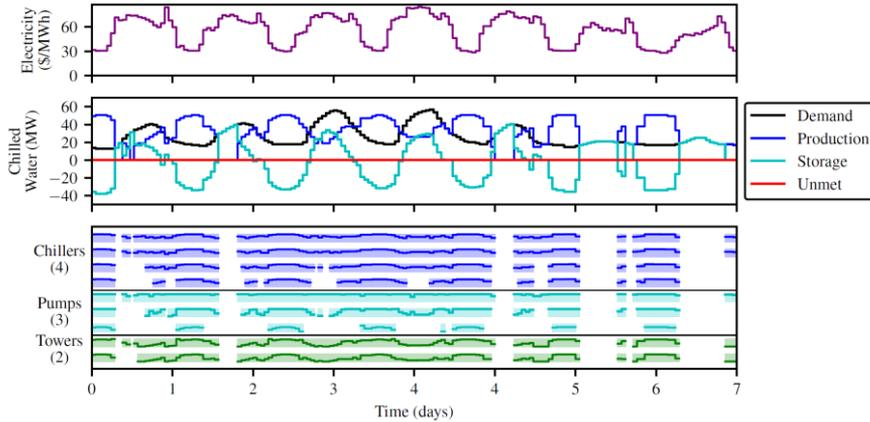
Figure 2: Sample optimal trajectory for the cooling-only system. Central plant equipment is shown in the Gantt chart with light bars showing equipment on/off and solid lines showing loading between minimum and maximum capacity.
