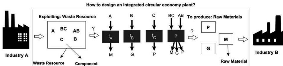
Figure 1: In what manner to combine waste-to-chemicals transformation processes in order to design a feasible integrated circular economy plant? A, B, C are pure materials, while AB and BC are blended, inseparable material.
