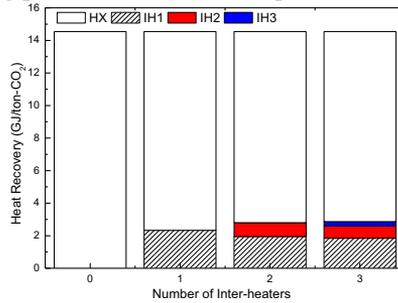
Figure 8. Overall heat recovery by the cross-flow heat exchanger and the inter-heaters.
