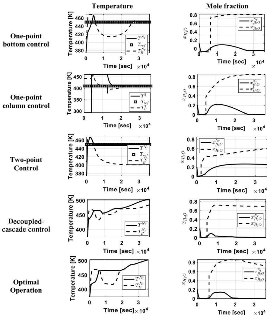
Figure 2: Closed loop trajectories of the main variables of the RBD. Temperature:  $T_i$  (—),  $T_{B_i}$  (---), and  $T_{ref_i}$  (□). Concentration:  $x_{H_2O}^1$  (---), and  $x_{H_2O}^{Nr}$  (—).
