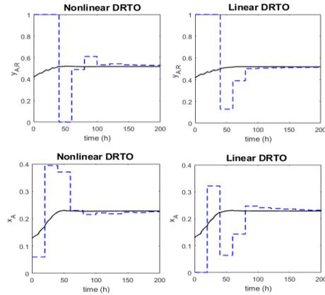
Figure 2: Set-points and output response for distributed MPC cases
