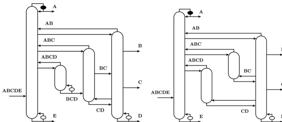
Figure 2: Configurations amenable for retrofitting of indirect split configuration, for light crude fractionation example. (a) and (b) require 19.4 % and 16 % less vapor duty compared to indirect split configuration
