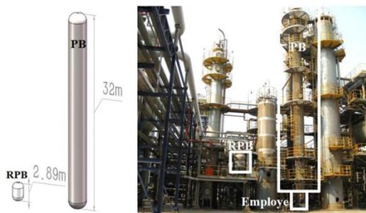
Fig. 1 The comparison between RPB and PB within an industry case
