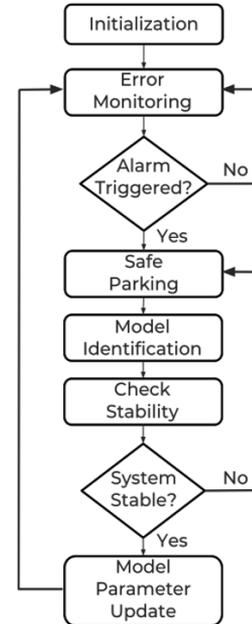
Fig. 1. Flowchart of the algorithm integrating model identification and model-based control.
