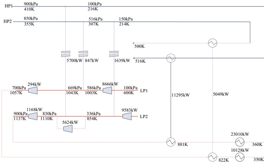
Figure 6 Optimal WHEN configuration for Case B
