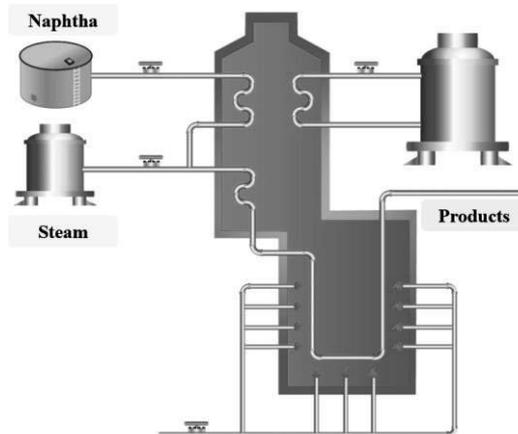
Figure 1. Schematic production process of the steam cracking furnace
