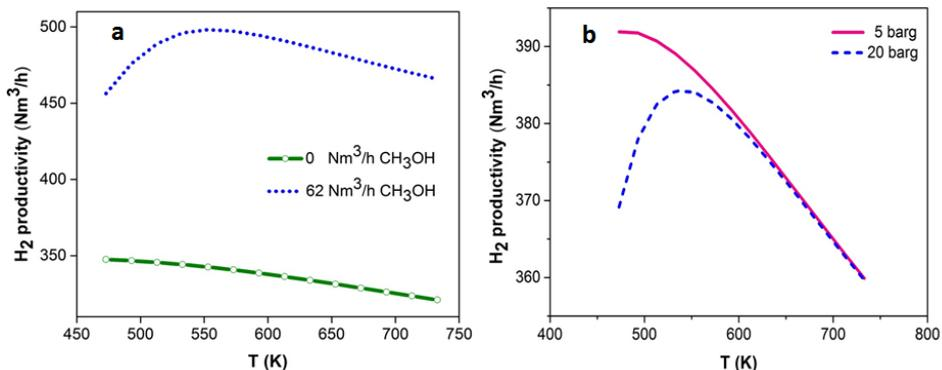
**Figure 1.** (a) Effect of methanol addition (20 barg). (b) Effect of temperature and pressure ( $CH_3OH$ :  $16 \text{ Nm}^3/\text{h}$ )
