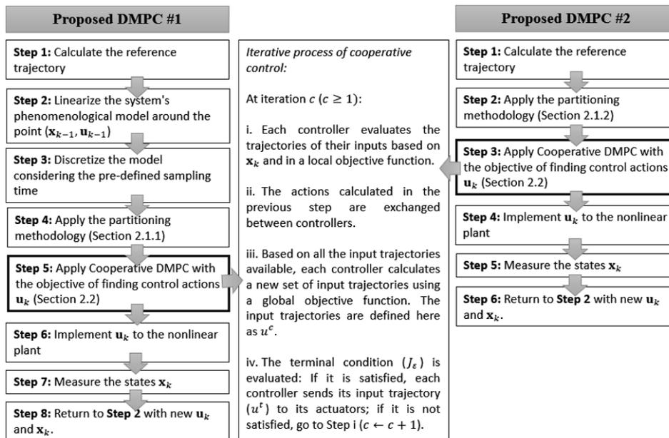
Figure 1: Cooperative DMPC schemes proposed in this work, with emphasis on the iterative process of cooperative control methodology.
