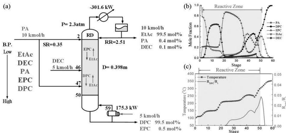
Figure 2: The DEC proposed design of (a) steady-state results (b) composition profile (c) temperature profile
