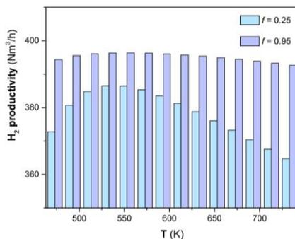
**Figure 3.** Effect of temperature on the H<sub>2</sub> productivity, SEMtoS (20 barg, 16 Nm<sup>3</sup>/h CH<sub>3</sub>OH)
