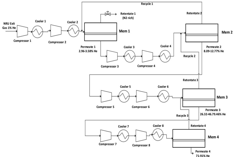
Figure 1. Illustration of four-stage cascade membrane processes with cross-flow and counter-current flow patterns used for Concept-A-1 & A-1, Concept-B, Concept-C-1& C-2 and Concept-D. All simulations are performed to produce >90% He with fixed 99% recovery from 1% He feed concentration at Nitrogen Rejection Unit off-gas.
