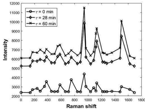
Figure 1: Raman Spectra for reaction mixtures as a function of  $\tau$
