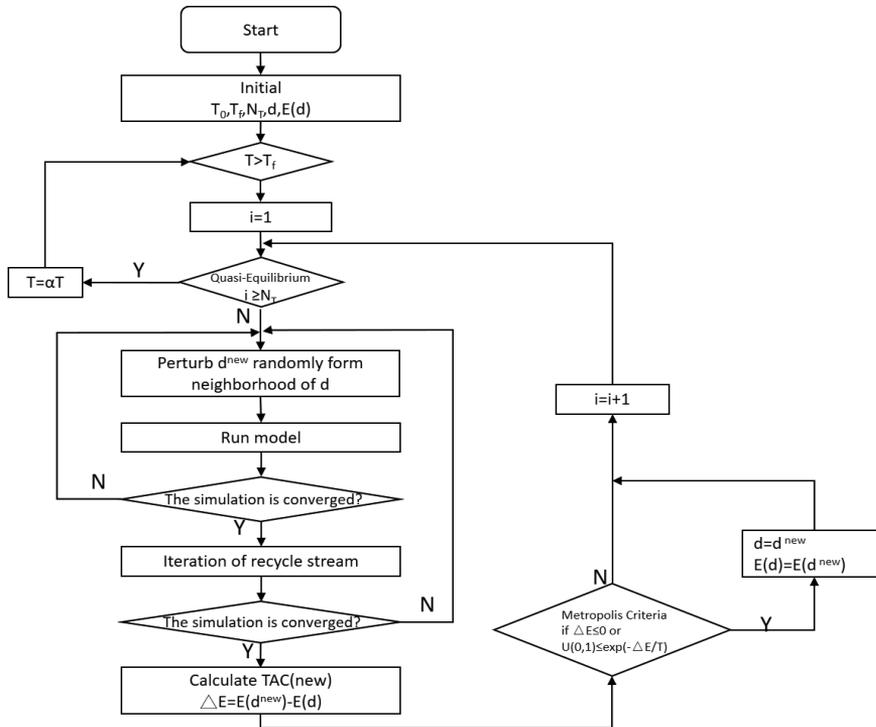
Figure 3. Flowchart of the simulated annealing algorithm
