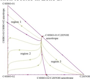
Fig. 1 RCM of the ternary mixture at 101.3 kPa
