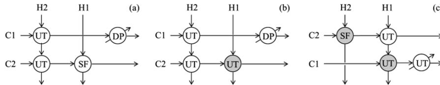
Figure 2. Topology of HEN at different operability level:
