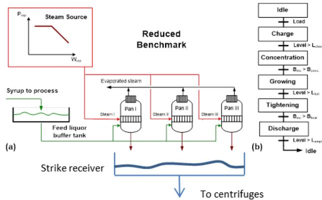
Figure 1. Schematic of the benchmark problem with two buffer tanks and three vacuum pans for sugar crystallization
