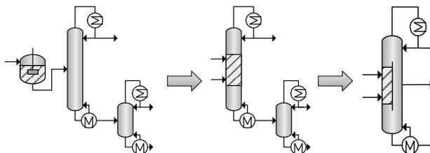
Figure 1: Levels of process integration: reactor and direct distillation column sequence (left), direct reactive distillation sequence (middle) and reactive dividing wall column (right)
