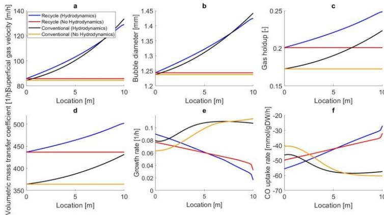
**Figure 3.** Steady-state profiles of hydrodynamic and GEM variables for two bubble column reactor configurations with and without hydrodynamics.
