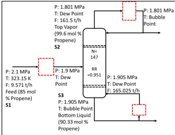
Figure 1. Flowsheet for the C3 splitter
