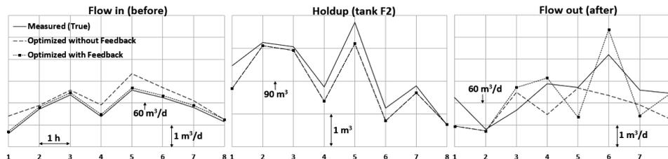
Figure 3. Measured and optimized solutions for tank F2 (see Figure 2).
