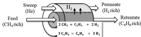
Figure 1. DMA-MR cocurrent configuration scheme.
