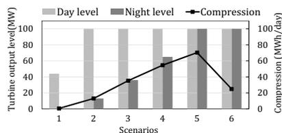
Figure 6. Turbine output levels and compression demand for storage in all scenarios
