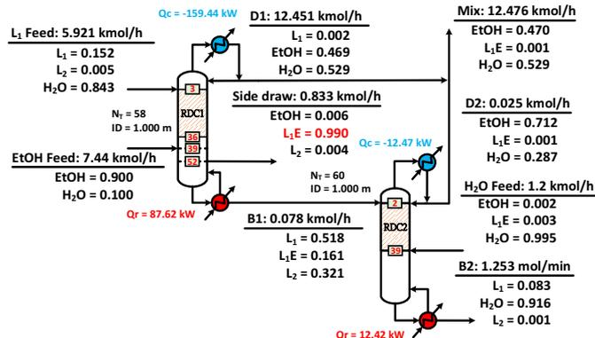
Figure 2. The modified process for reactive part
