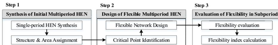
Figure 1 Procedure for design of flexible multiperiod HEN
