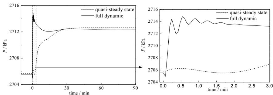
Figure 4. Dynamic response of reactor in quasi-steady state and full dynamic model
