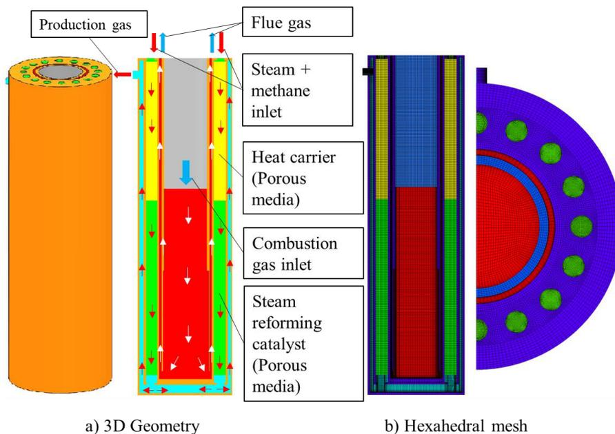
Fig. 1. Schematic diagram of SMR reactor and hexahedral mesh structure.
