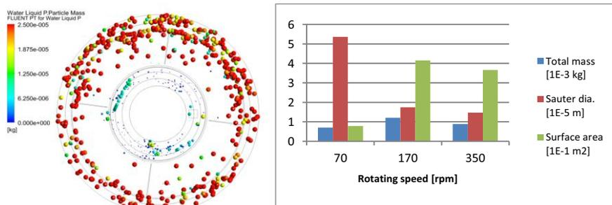
Figure 5. Simulation results on liquid droplets (left-overall configuration, right-summary)
