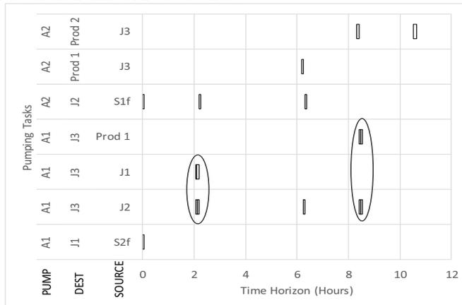
Figure 4 (a) Optimal pumping scheduling using floating pumps
