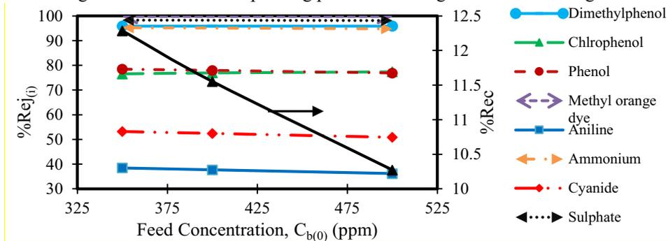
Fig. 3. Effect of compound concentration on rejection and recovery rate (operating conditions:  $2.583\text{E-}4$  m<sup>3</sup>/s, 10 atm, 30 °C)
