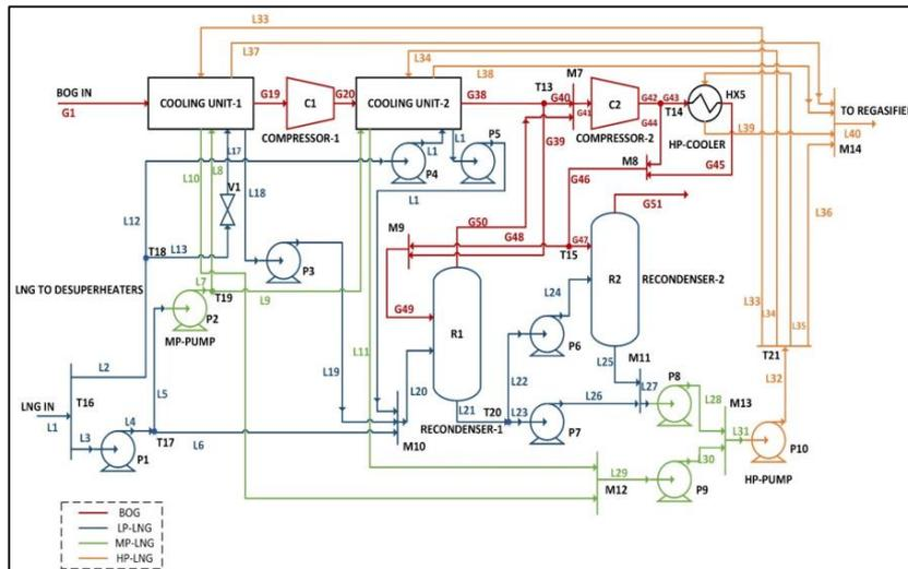
Figure 3: Superstructure for BOG reliquefaction
