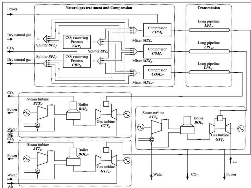
Figure 1. A schematic diagram of a typical DNGN
