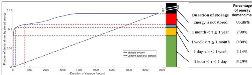
Figure 1: Storage profile against the duration of storage for Lerwick with 60% RES penetration and 50% Wind:50% Solar power supply
