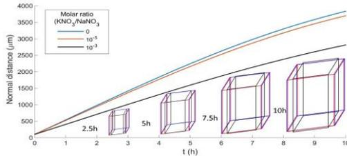
Figure 2 Evolution normal distance of face  $\{104\}$  and crystal shape during  $\text{NaNO}_3$  crystal growth with different  $\text{KNO}_3/\text{NaNO}_3$  molar ratio
