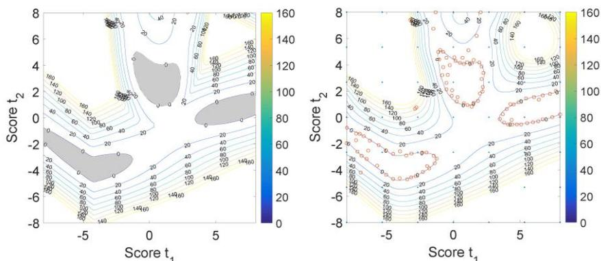
Figure 2. (a) Projection of the original function onto the 2-dimensional latent space. The grey-shaded area is the feasible region. (b) RBF model after 100 iterations. Dots represent the initial samples. Circles represent the adaptive sampling points after 100 iterations.
