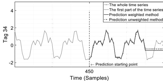
Figure 5 Prediction of Tag 34 with  $N = 450$ ,  $h = 30$ ,  $k = 26$ ,  $m = 27$  using the weighted ( $E_{av} = 0.0178$ ) and unweighted ( $E_{av} = 0.0202$ )  $k$ -nearest neighbor methods.
