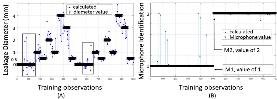
Figure 1. Values calculated by the supervised network and the observations used to train the network. (A) Leakage diameter value; (B) Microphone value
