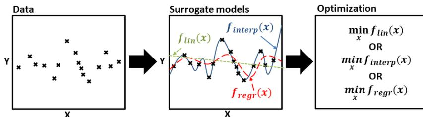
Figure 3. Concept of fitting parametric models (regression, interpolation) to data and finally using these functions for optimization.
