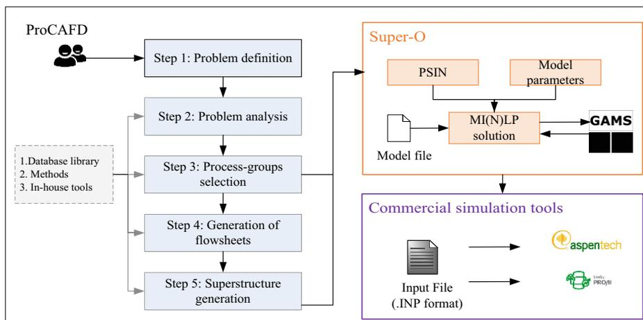
Figure 4: Schematic representation of integrated computer-aided tool for process synthesis
