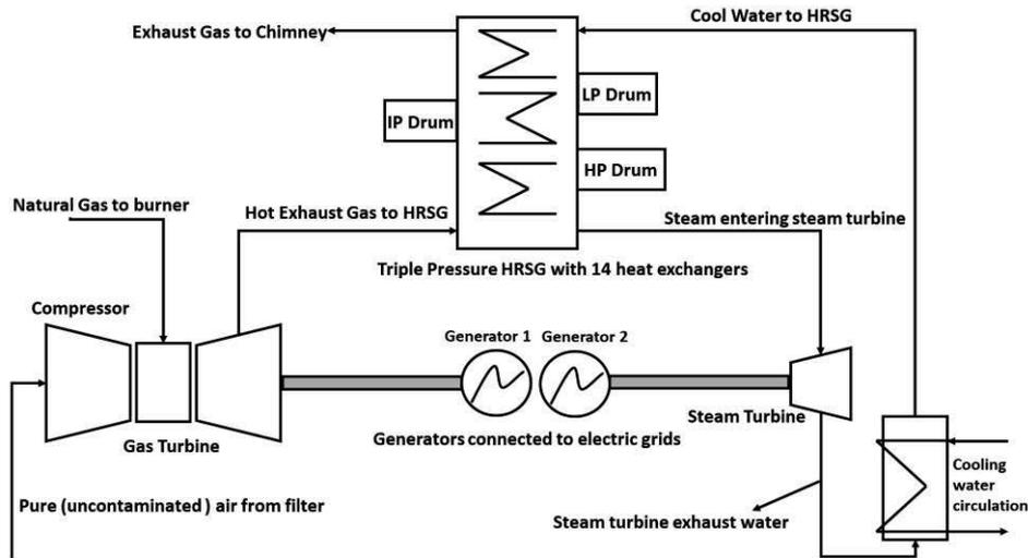
Figure 1. Schematic of CCPP with vertical HRSG
