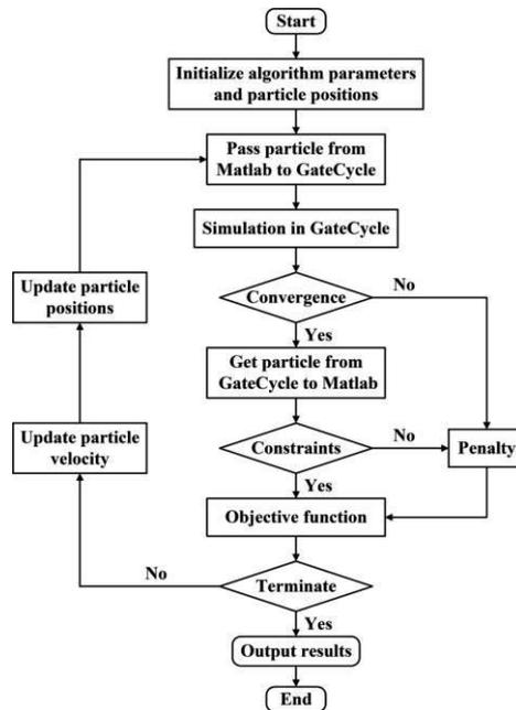
Figure 2 Simulation-based optimization using PSO algorithm.
