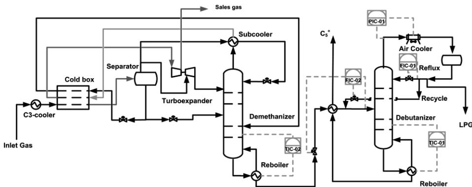
Figure 1. Simplified flow sheet representing the NGPP considered in this work.
