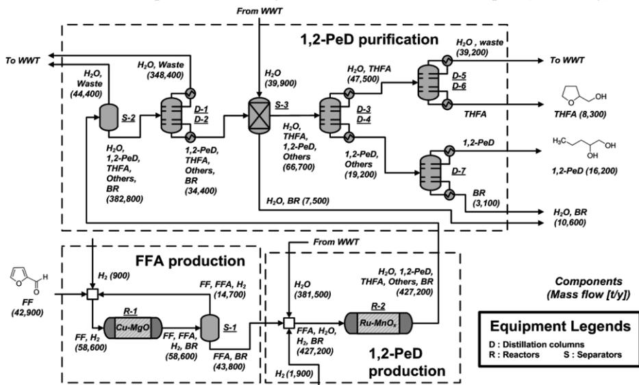
**Figure 2.** Simplified process flow diagram for the integrated process to produce 1,2-PeD and THFA from FF
