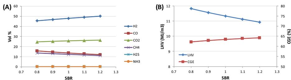
Figure 4. Effects of SBR in spruce gasification.
