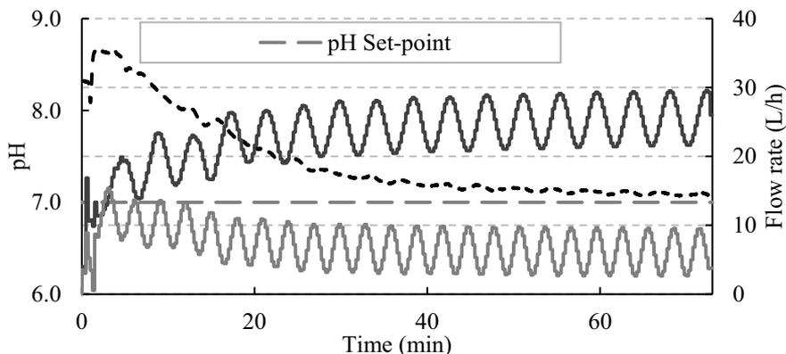
Figure 4 – MISO experimental results. Acid (FIC-101) and base (FIC-102) flow rates as manipulated variables.
