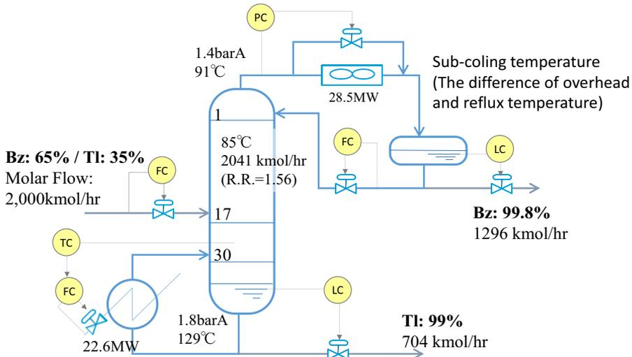
Fig.1 Example distillation column model and representative process variables
