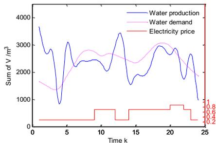
Figure 2: The relation between production water, water demand and electricity price under  $S_0$  scheme
