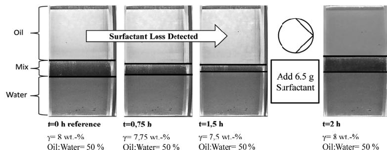
Figure 3: Gauge glass images of the settler over an operation horizon of 2 h and results of the soft-sensor calculations. The right picture shows the separation state after a performed control action derived from the dynamic optimization.
