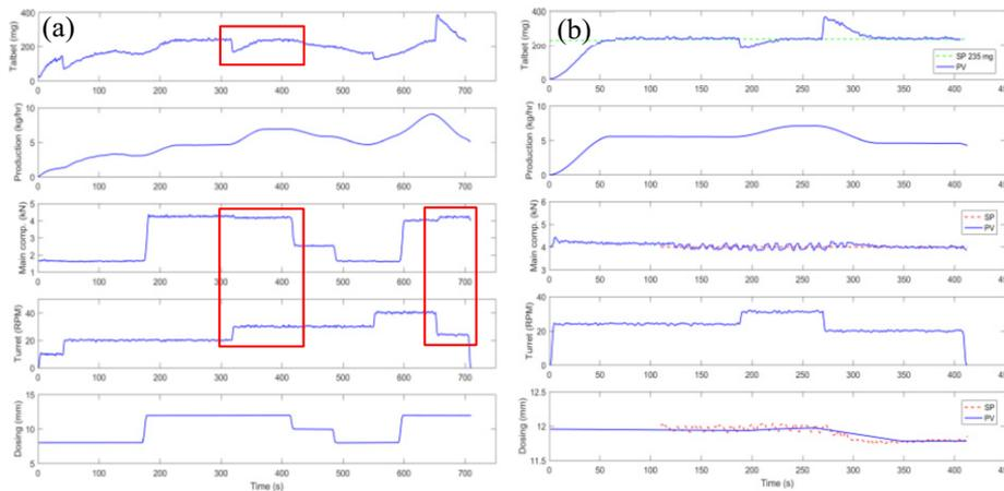
Figure 3. (a) Step changes in turret speed and dosing level under Level 0 control; (b) variation of the turret speed on tablet weight and main compression force control under Level 1 control when production rate control loop was deliberately set to be open.
