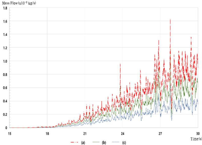
Figure 5 Flow rates of NO by time. (a)5:5, (b)6:4, (c)7:3
