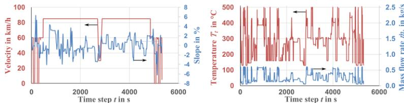
Figure 1: Time series of (left): the velocity and road slope of the VECTO LHC (Dünnebeil et al., 2015) and (right): the temperature and mass flow rate of the exhaust gas (Bergmann et al., 2017).
