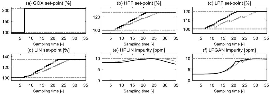
Figure 4: Temporal course of relevant process variables for a change of product mix of the ASU without disturbances. Solid black lines show optimal trajectories from NL DO. Thin grey lines show results of the industrial benchmark (without NL DO). Dashed-dotted grey lines show constraints.
