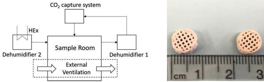
Figure 1: Schematic of the air capture process (left) and 3D zeolite 13X monolith (right)
