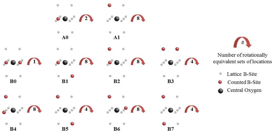
Figure 2: Examples of possible geometric descriptors for placement of dopant on B-sites
