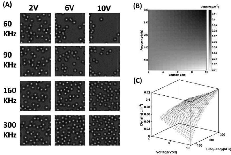
Figure 2. (A) Microscopy images of particle densities at different operating frequencies and voltages. Each image shows a part of the area that is used for measuring the density with image analysis for illustrative purposes; (B) Grayscale mapping of the density with respect to frequency and voltage; (C) Surface plot of the particle density as function of frequency and voltage.
