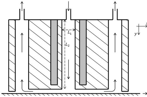
Figure 1. Cross-section of the deposition site in the direction of the flowing glass.
