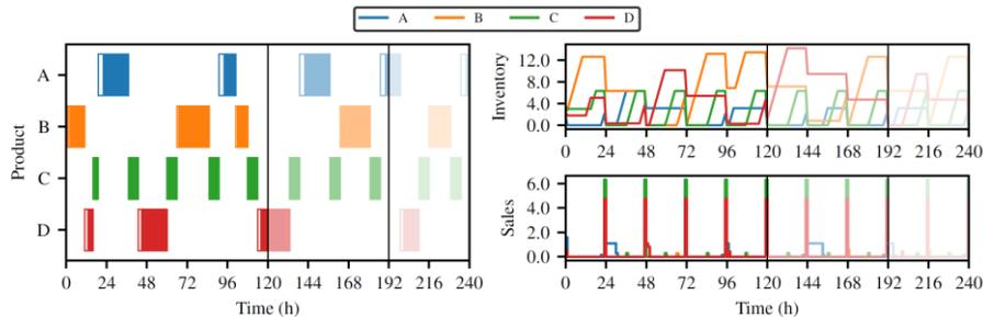
Figure 1: Beginning of closed-loop solution with horizon  $N = 72$  and terminal constraint  $T = 48$ . Plots are split into three sections by vertical lines. First section shows closed-loop solution so far. Second section shows incumbent schedule. Third section shows reference trajectory on which the incumbent schedule terminates.
