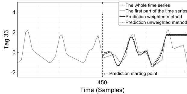
Figure 4 Prediction of Tag 33 with  $N = 450$ ,  $h = 30$ ,  $k = 26$ ,  $m = 27$  using the weighted ( $E_{av} = 0.0679$ ) and unweighted ( $E_{av} = 0.0855$ )  $k$ -nearest neighbor methods.
