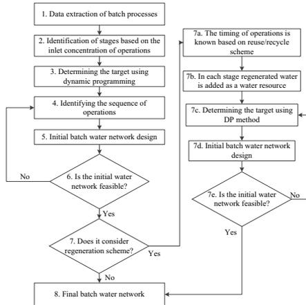
Figure 1 The design procedure for batch water network
