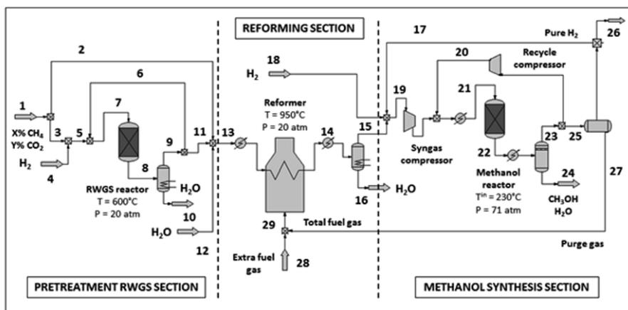
Figure 1. Methanol production from NG with a high  $\text{CO}_2$  content. Flow diagram.
