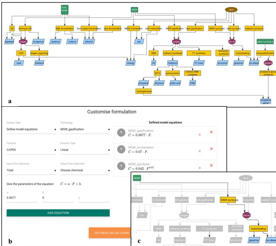
Figure 5. (a) The value chain produced for MSW, food waste, waste cooking oil and bark. (b) The interface of CAPS platform for customised optimisation formulation. (c) The optimised path.
