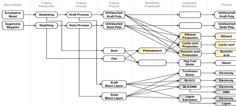
Figure 1. Overview of superstructure for integrated biorefinery network
