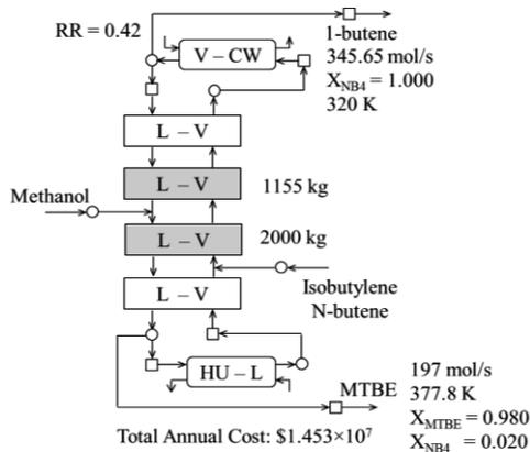
Figure 4. Optimal GMF design of MTBE reactive distillation
