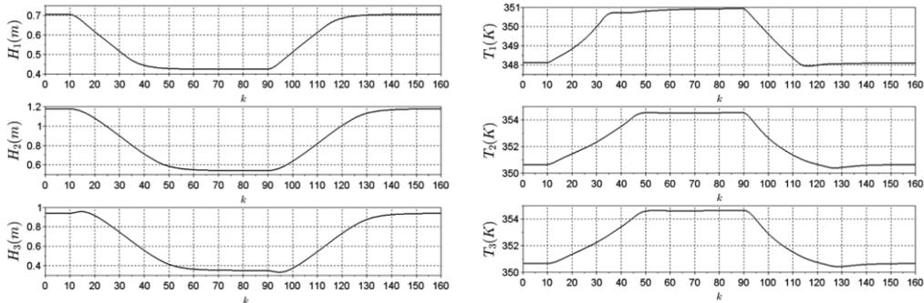
Figure 3: Dynamic evolution of controlled outputs obtained by centralized control and proposed DMPC approaches (overlapping curves).
