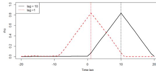
Figure 1: Calculate the correlation coefficient rho by shifting the lag between x and y. To the simple system, the time delay lag is the time lag at which the rho is maximum.
