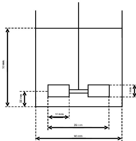
Figure 1 – Extraction vessel dimensions.
