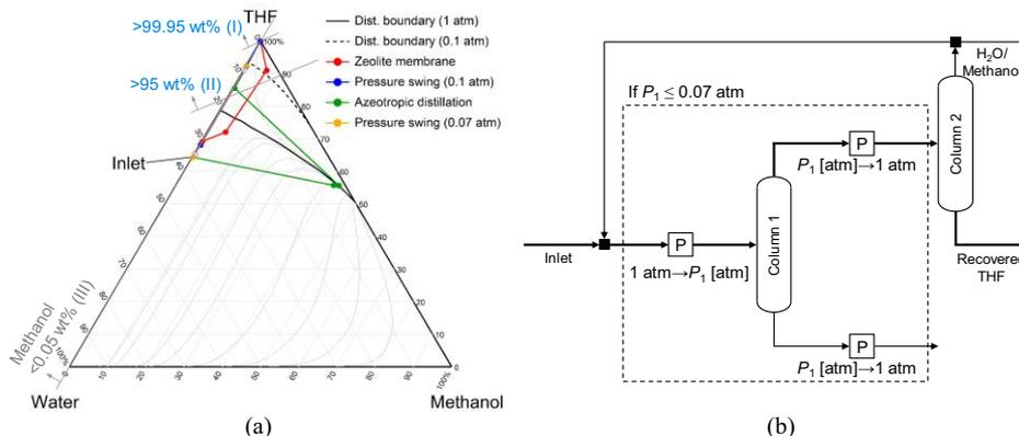
Figure 2. (a) ternary phase diagram of THF/water/methanol (b) pressure swing process
