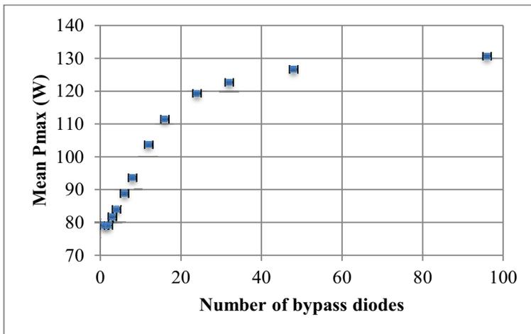
Figure (4): MC simulation results for each bypass diode case.
