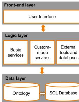
Figure 4. The architecture of the developed platform.
