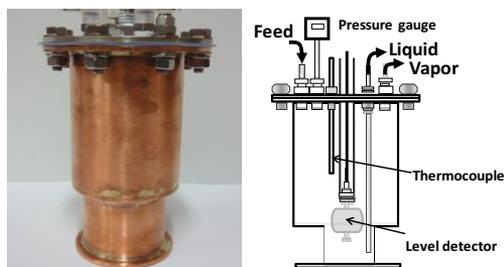
Figure 5. A device for a stage in PDDS
