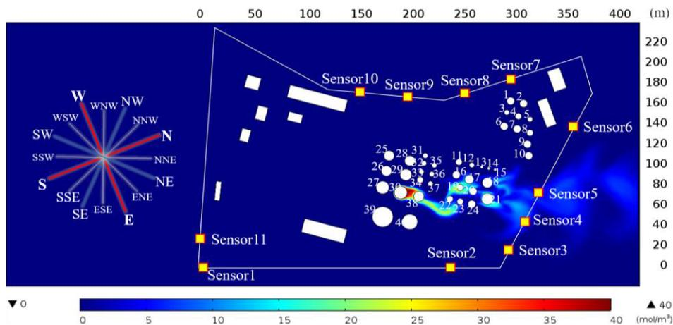
(b) An example of CFD simulation result: NNE wind, leakage of the 30-storage tank.
