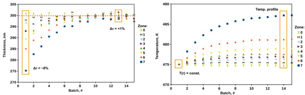
Figure 4. (left) Batch-to-batch thin film thickness. (right) Temperature profile developed via EWMA algorithm.
