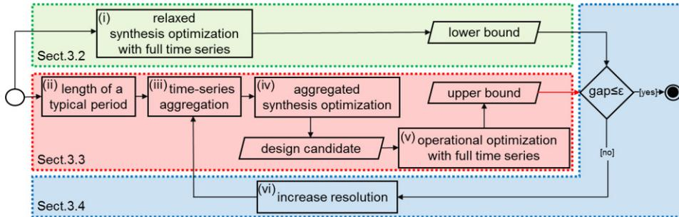
Figure 1: Rigorous synthesis method for energy systems employing time-series aggregation and relaxation to satisfy an optimality gap  $\epsilon$ .
