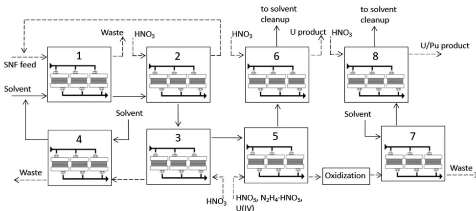
Figure 1: Diagram of COEX process. Continuous line refers to organic stream, dashed line refers to aqueous stream. Flow rate of SNF feed is approximately  $200 \text{ L h}^{-1}$ .
