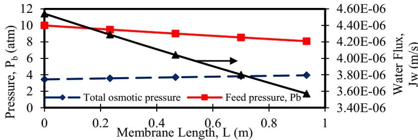
Fig. 2. The variation of operating parameters along the membrane length
