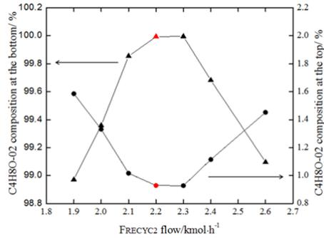
Fig. 7 The dependence of the T1 column product purities on the flow rate of RECYC2.
