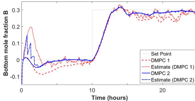
Figure 2: Comparison of DMPC with and without delayed primary measurements, DMPC 1 represents distributed MPC without primary measurements (secondary measurements only) and DMPC 2 includes delayed primary measurements.
