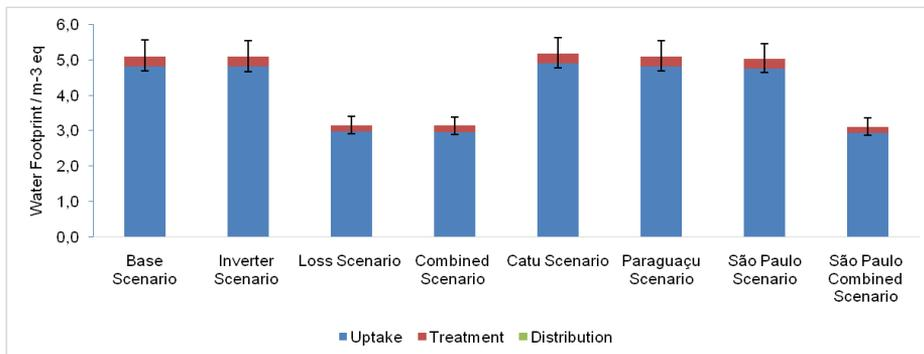
**Fig. 4** Impact contribution of Water Footprint with uncertainty\* (foreground) of 1 m<sup>3</sup> of distributed water per stage along the life cycle for each scenario
