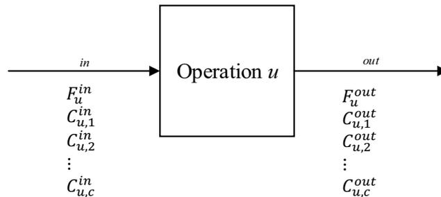
Figure 1. Representation of an operation  $u$  and its inlet and outlet contaminants concentrations and flowrates.
