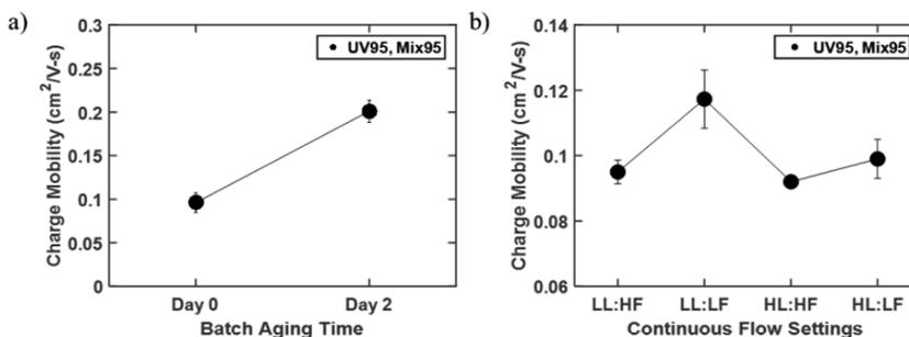
**Figure 1.** (a) Average charge carrier mobilities of OFETs for batch processing conditions. (b) Average charge carrier mobilities of OFETs for continuous flow processing conditions. Error bars denote standard errors over multiple replicates.
