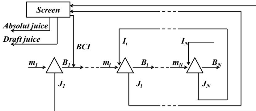
Figure 3 - Schematic flowchart of a sugarcane industry
