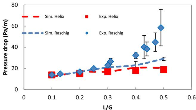
Figure 4 The validation of the pressure drop of helical rings and Raschig rings
