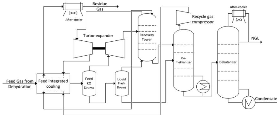
Figure 1: NGL unit simplified schematic
