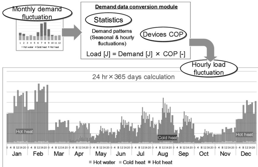
Figure 1 Data conversion of monthly demand of heat in Tanegashima, where the monthly data was investigated from actual buildings. The coefficient of performance (COP) of installed devices was also obtained from the investigation.
