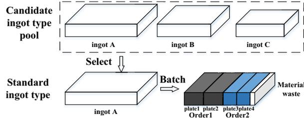
Figure 1. The integrated process of ingot type selection and order batching
