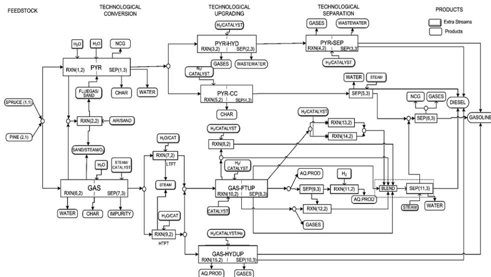
Figure 2. Thermochemical BtL process synthesis network superstructure
