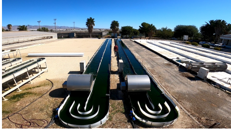
Fig. 1. Raceway reactor located at IFAPA
