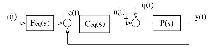
$$C_{eq}(s) = \frac{C(s)F_r(s)}{1 + C(s)G_n(s)(1 - e^{-L_n s}F_r(s))}, \quad F_{eq}(s) = \frac{F(s)}{F_r(s)},$$
