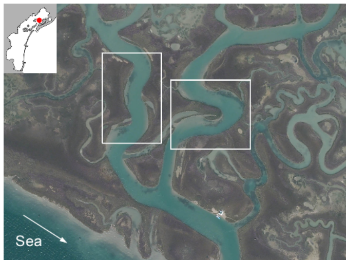
Fig. 1. Example of tidal meanders in the Venice Lagoon (Italy). The highlighted portions mark point bars, which are shifted seaward with respect to the apex of the meander.
